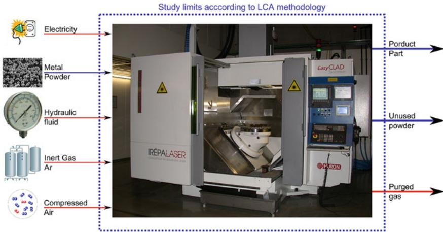
**Fig. 17** Directed energy deposition (CLAD) process
