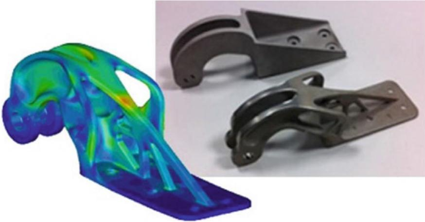
**Fig. 11** Airbus A320 nacelle hinge bracket (*back*) and the optimised design produced by ALM (*front*). Courtesy of EADS and ALTAIR [20, 63]
