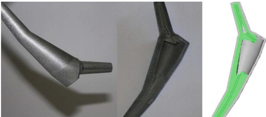
**Fig. 13** View of manufactured hip right out of the oven [20]
