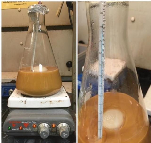
**Fig. 1** Alkaline hydrolysis setup for the production of glucan particles
