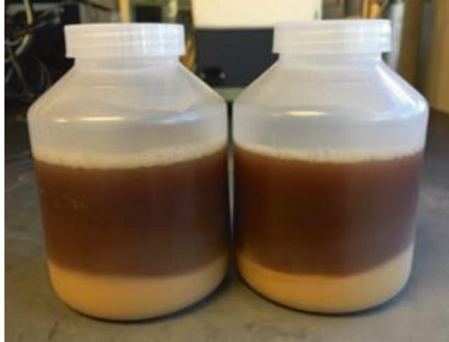
**Fig. 2** Centrifuge bottles after first spinning (pH > 10). *Dark brown* supernatant and *white* floating partially saponified lipids must be discarded. Pellet must be washed until the supernatant is clear and pH < 10 (it usually requires four to five washes)
