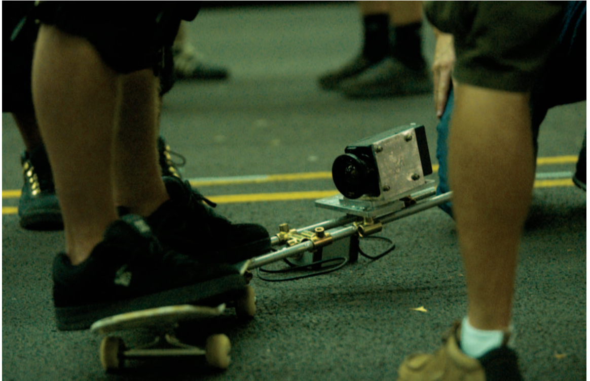
Figure 2-14 16mm GSAP camera mounted to pro skateboarder Danny Way's board.
