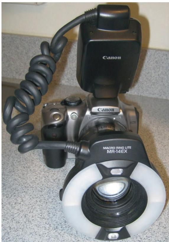
**Fig. 3.12** Digital SLR camera equipped for intraoral photography with macro lens and ring flash
