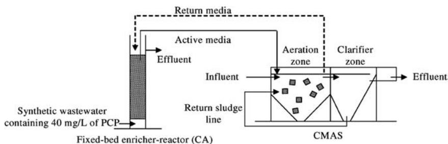
**Fig. 7.11** A diagram of immobilized cell augmented activated sludge system [6], Reprinted by permission of the publisher
