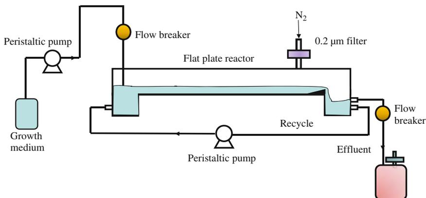
**Fig. 1.3** Schematic illustration (not to scale) of a flat plate reactor used to image biofilms and study uranium immobilization and local chemistry in biofilms
