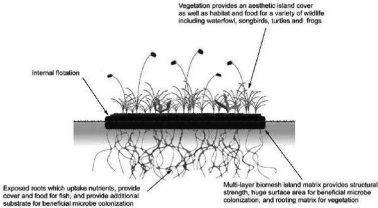
**Fig. 9.9** Schematic of floating platforms from Floating Island International and Floating Island International Southeast
