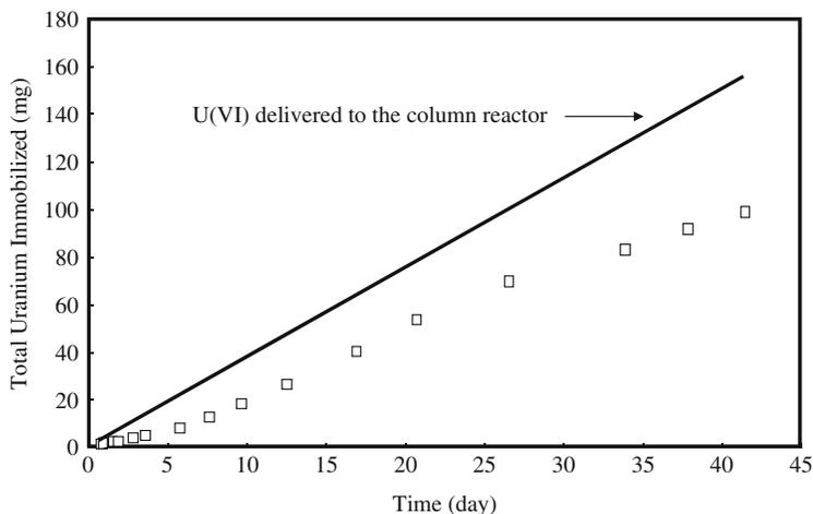
**Fig. 1.12** Total amount of uranium accumulated in lactate-stimulated indigenous biofilms on sediments from the Hanford 300 Area. The reactor was fed with 126  $\mu\text{M}$  U(VI) at a flow rate of 125 mL/day. The continuous line shows the cumulative amount of uranium delivered to the reactor (the maximum possible uranium accumulation)
