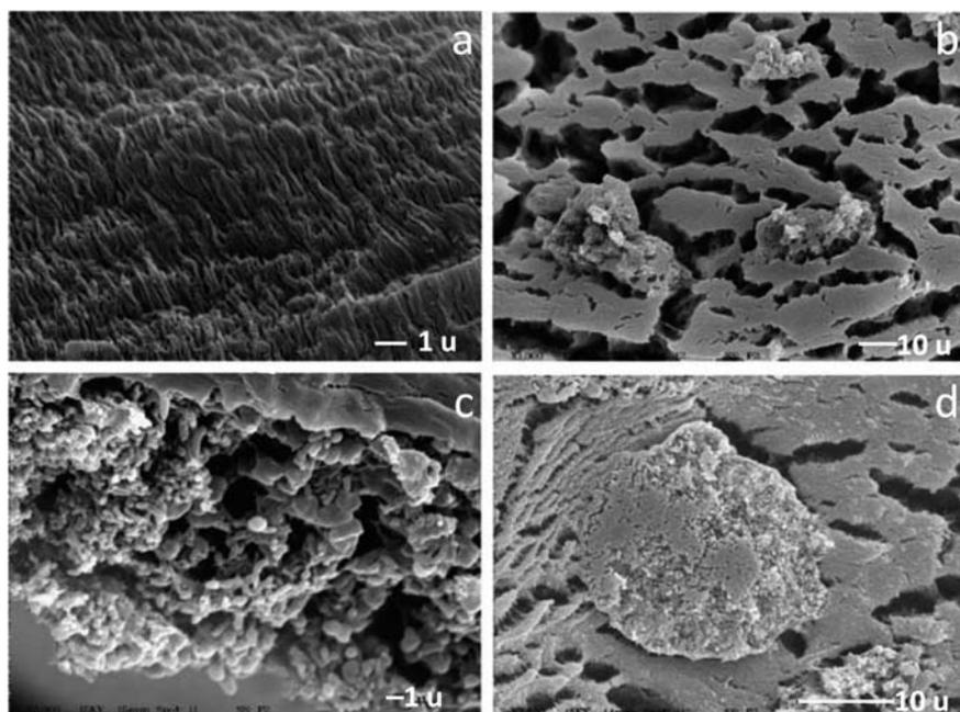
**Fig. 7.8** SEM images of calcium alginate entrapped nitrifying bacteria: (a) Bead surface after entrapment, (b) Interior bacterial floc after entrapment, (c) Surface rupturing bacterial colony after experiments, and (d) Interior bacterial colony after experiments [44]
