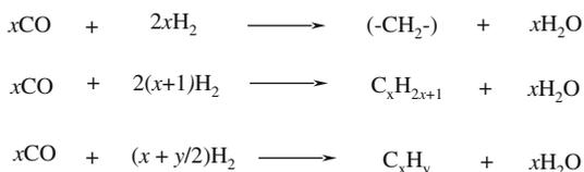
**Fig. 8.11** FTS reactions for the production of linear long-chain hydrocarbons
