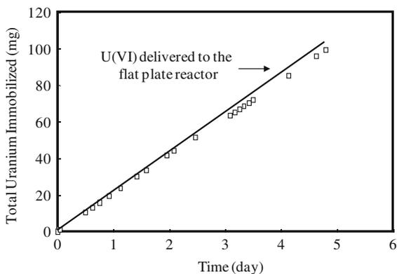
**Fig. 1.6** Total amount of uranium accumulated in *S. oneidensis* MR-1 biofilms. The flat plate reactor was fed with 126  $\mu\text{M}$  U(VI) at a flow rate of 30 mL/h. The continuous line shows the cumulative amount of uranium delivered to the reactor (or maximum possible uranium accumulation)
