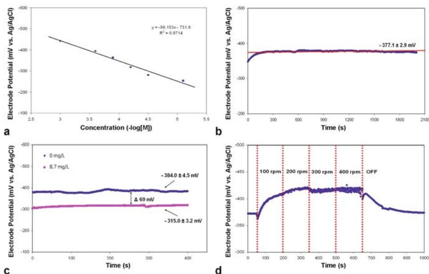
**Fig. 6.10** Characterization of phosphate MEA sensor at pH 7.5: (a) calibration curve in various concentrations of  $\text{KH}_2\text{PO}_4$ , (b) long-term stability test in  $10^{-3.9}$  M  $\text{KH}_2\text{PO}_4$ , (c) the oxygen effect in  $10^{-3.9}$  M  $\text{KH}_2\text{PO}_4$ , and (d) the stirring effect in  $10^{-3.9}$  M  $\text{KH}_2\text{PO}_4$  [59]
