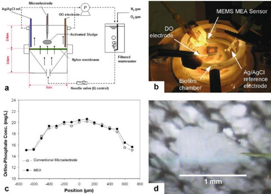
**Fig. 6.13** Phosphate measurements in Biofilm: (a) schematic diagram of up-flow chamber (adapted from [73]), (b) photograph of up-flow chamber, (c) microprofiles of phosphorus in flocs from the EBPR process, and comparison with the phosphorus microprofiles from conventional microelectrode (ME) and phosphate MEA, and (d) penetration of microelectrode through the floc during microprofiling [60]
