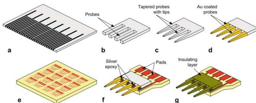
**Fig. 6.3** Microelectrode array (MEA) sensor batch fabrication sequence: (a) dice glass wafer, (b) form glass probes by dicing, (c) use meniscus etching to sharpen probes, (d) deposit Au conductive layer, (e) pattern PCB, (f) use silver epoxy to establish electrical connections, and (g) coat microelectrodes with parylene insulating layer and fabricate recessed tips [55, 57]
