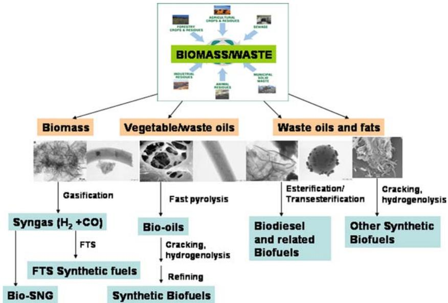
**Fig. 8.8** Biomass gasification and pyrolysis routes to synthetic biofuels
