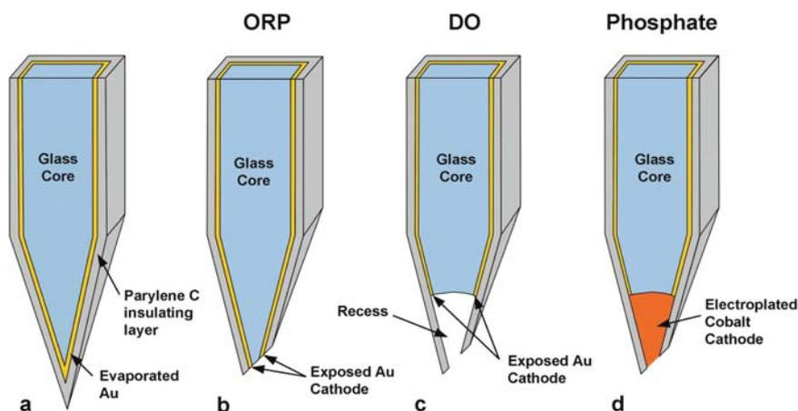
**Fig. 6.5** Tip structures of the multi-analyte MEA sensor: (a) Parylene C insulating layer covering the entire microelectrode, (b) beveled and exposed glass and gold cathode, (c) glass and Au etching for the recessed oxygen sensor, and (d) cobalt electroplating for the phosphate sensor
