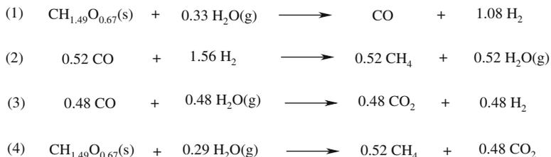
**Fig. 8.9** Reactions involved in the conventional gasification of biomass
