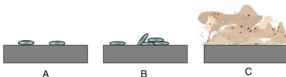
**Fig. 1.2** A mineral with attached cells on the surface: (a) a few cells are attached to the surface; (b) the cells increase in number and start to cover the surface; (c) the surface is covered by layers of cells
