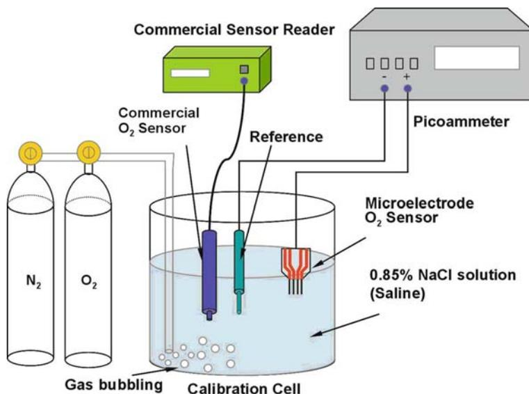
**Fig. 6.8** Schematic diagram of the calibration cell for DO MEA characterization. A picoammeter was used to measure current directly with respect to a commercial Ag/AgCl reference electrode
