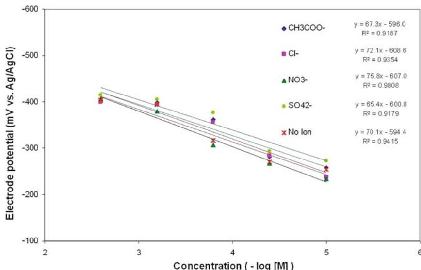
**Fig. 6.11** Results of the interference tests by the phosphate MEA sensors in various concentrations of  $\text{KH}_2\text{PO}_4$  at pH 7.5. No meaningful differences were found, indicating no interference susceptibility to the tested ions [59]
