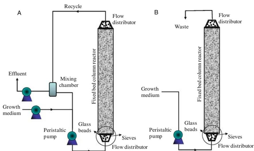
**Fig. 1.4** Experimental setup (a single column). (a) A polycarbonate column filled with minerals is operated continuously with a recycle. The recycle provides higher flow rates in the column. (b) A flow through a column reactor
