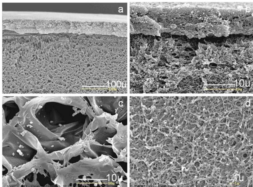
**Fig. 7.10** SEM images of PPVA entrapped cells: (a) Cross-section at 250 $\times$ , (b) Exterior layer at 3000 $\times$ , (c) Interior layer at 3000 $\times$ , and (d) External surface at 5000 $\times$  [57]
