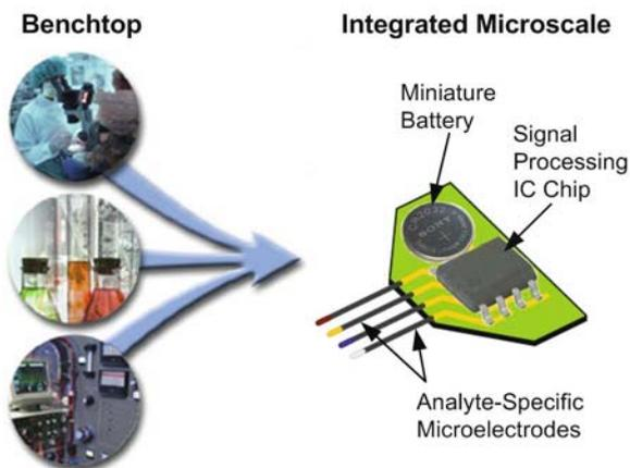
**Fig. 6.2** Concept of an integrated multi-analyte MEMS sensor array for *in situ* monitoring in biofilms and the environment [57]
