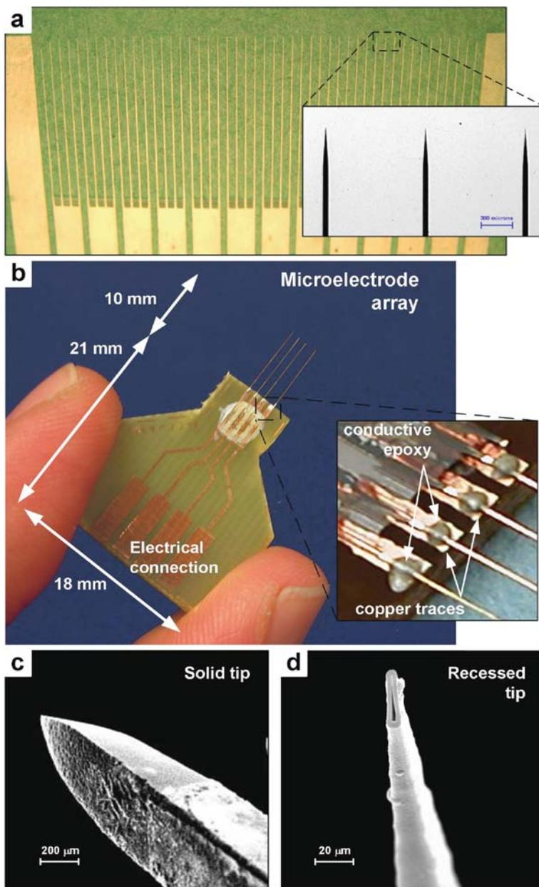
**Fig. 6.6** Photographs of (a) an etched glass wafer with probe tips at the center and near the edges. Close-up shows parallel tip ends at 900  $\mu\text{m}$  center-to-center spacing, and (b) the fabricated DO microelectrode array sensor packaged on a PCB carrier. Close-up shows the design of the MEA packaging using conductive silver epoxy. Scanning electron micrographs (SEMs) of (c) sharpened solid tip, and (d) recessed tip at 45° beveling angle. (Adapted from [57–59])
