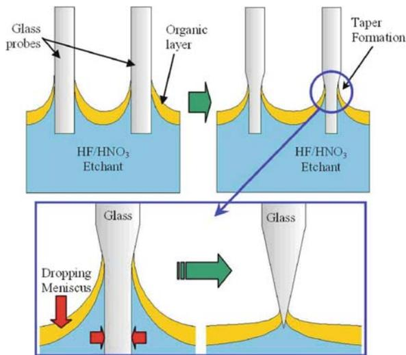
**Fig. 6.4** Fabrication of sharp MEA tips using meniscus etching. Meniscus height falls dynamically to form a taper with geometry dependant on the initial meniscus height [55, 57]
