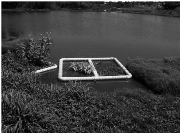
**Fig. 9.2** Platform of PVC pipe and chicken wire tested at commercial hog farm
