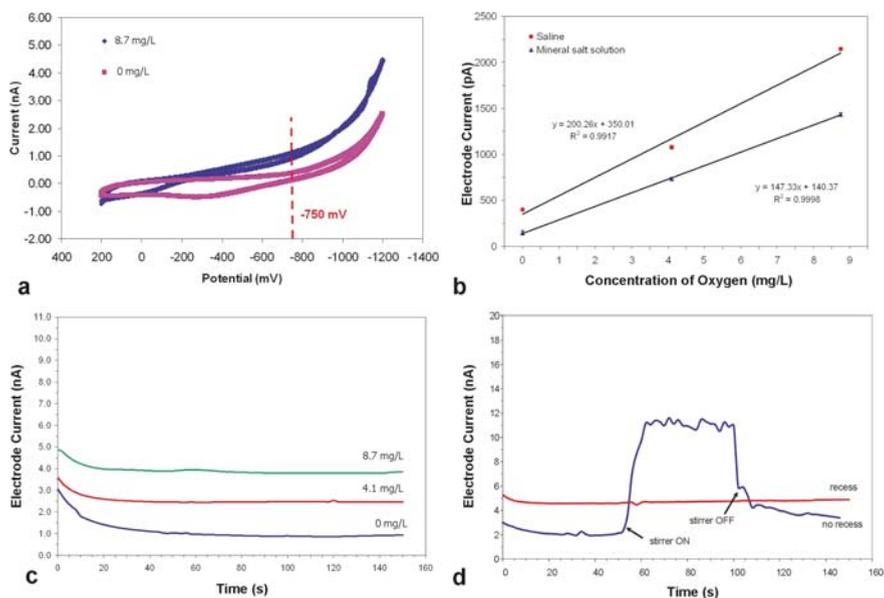
**Fig. 6.9** Representative results of DO MEA sensor characterization. (a) Cyclic voltammogram (CV) curve for 0 mg/L and 8.7 mg/L DO in saline solution at a scan rate of 10 mV/s. (b) Calibration curves in 0.85% NaCl saline and mineral salt solutions. (c) Representative current response for an MEA sensor at three DO concentrations. (d) Representative stirring effect results that compare response of recessed and non-recessed sensor tips at 500 rpm agitation. Adapted from [57, 58]
