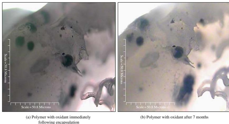
**Fig. 2.2** Photo of polymer with  $\text{KMnO}_4$  7 months after encapsulation
