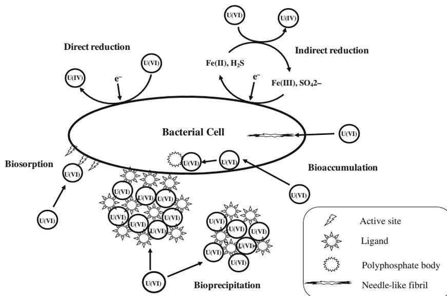
**Fig. 1.1** Reducing and non-reducing mechanisms during the bioremediation of uranium using bacterial cells: direct and indirect reduction, biosorption, bioprecipitation, and bioaccumulation [32, 35, 3, 44, 27]
