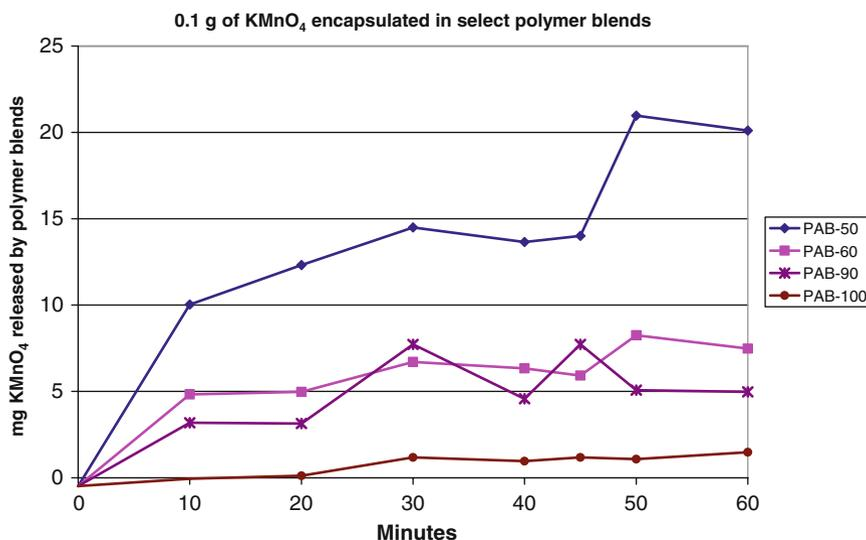
**Fig. 2.4** Prototype  $\text{KMnO}_4$  release for the hydrophilic and hydrophobic polymer blends
