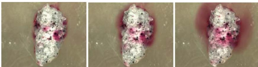
**Fig. 2.3** Time series photos of pellet with oxidant diffusing from shell
