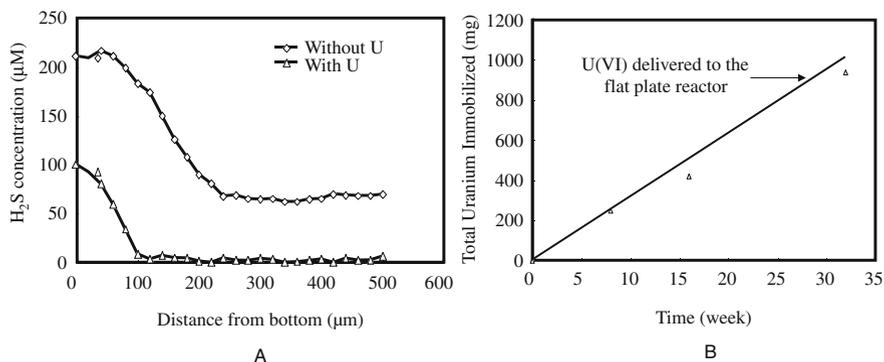
**Fig. 1.5** (a) H<sub>2</sub>S concentration profiles in three-week-old biofilms grown without U(VI) and with U(VI). (b) Uranium accumulated in SRB biofilms. Reprinted “in part” with permission from Beyenal et al. [18]. Copyright 2007 American Chemical Society
