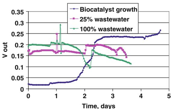
**Fig. 5.2** Voltage output during biocatalyst growth and during use of wastewater as the fuel source. The load on the MFC was 250 and 100  $\Omega$  during the growth period and the wastewater testing period, respectively
