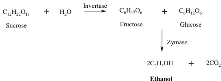
**Fig. 8.6** Production of bioethanol via fermentation of hydrolysed sugars from energy crops
