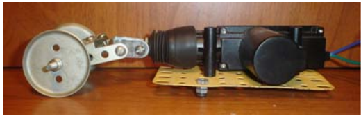
Fig. 8 General view of the prototype of a 1-D robot with one internal mass Fig. 9 Cleaner mini-robot with an electromagnetic actuator and two asymmetric friction elements: (a) general view of the cleaner: 1 – first body; 2 – electromagnet; 3 – armature; 4 – second body; 5 – asymmetric friction mechanism; 6 – elastic element; (b) design schematic of the cleaner: m_1 and m_2 – masses of the robot's components
