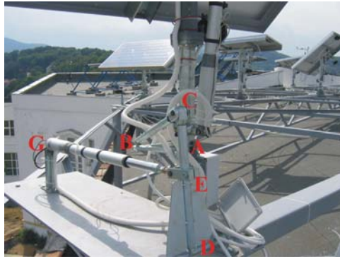
Fig. 15 An application example of the spatial tracking linkage with linear actuator at the University Transilvania of Brasov/Romania
