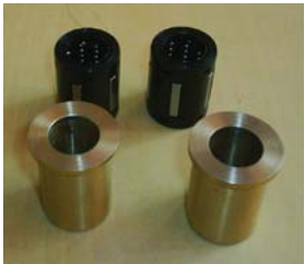
Fig. 12 Sliding and linear ball bearing bushings
