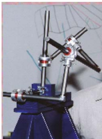
Fig. 6 Larochelle's RCCC mechanism [11]
