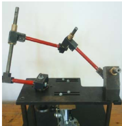
Fig. 5 RCCC mechanism from lab [10]
