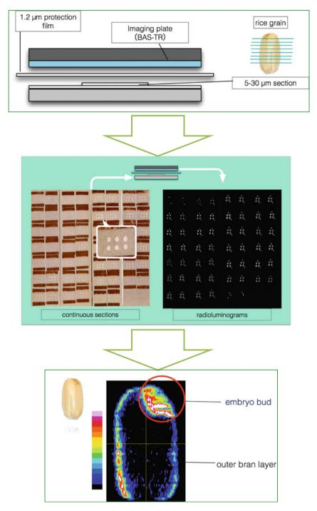
Fig. 19.4 The 3D construction from the sequential frozen sections in RLG. The sample shown here is a brown rice fed by  $^{137}\rm{Cs}$
