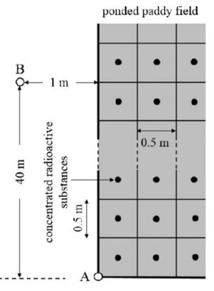
**Fig. 15.8** Paddy field and observation points A and B for numerical calculation of uncollided  $\gamma$ -ray flux. Paddy field is divided into *squares* of 0.5 m × 0.5 m and distributing radioactive substances are assumed to be concentrated at the center of each *square*
