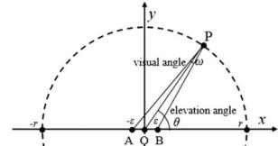
**Fig. 15.2** Visual angle  $\omega$  vs. elevation angle  $\theta$  when distance *r* is much longer than interval  $\varepsilon$
