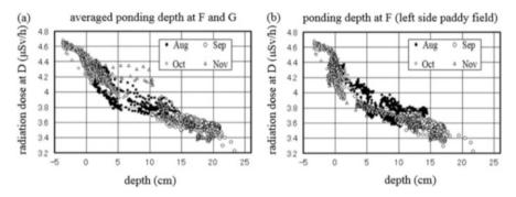
Fig. 15.15 Radiation dose at D (on the road) vs. ponding depth
