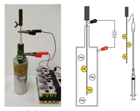
**Fig. 19.11** The <sup>42</sup>Ar–<sup>42</sup>K generator. A charge of 60 V was applied to the cathode to attract ionized <sup>42</sup>K. A few days after, the extracting solution was filled into the pipette in which the cathode was placed to obtain the <sup>42</sup>K
