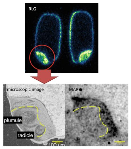
Fig. 19.5 The <sup>137</sup>Cs distribution in a rice grain visualized by RLG and MAR
