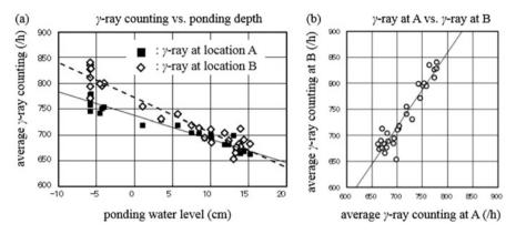
Fig. 15.7 Relationship between  $\gamma$ - ray counts and ponding depth at points A and B
