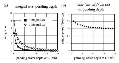
Fig. 15.17 Numerical integral at D and E to compare radiation doses
