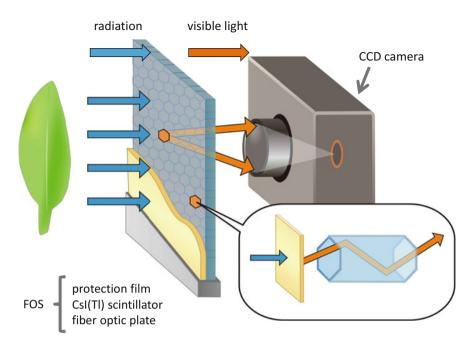
Fig. 19.7 How to make an image by real-time radioisotope imaging system. The radiation from the nuclides in a sample is converted to visible light by FOS containing scintillator. The CCD-camera catches the light sequentially
