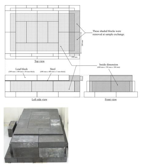
Fig. 19.1 The lead shield employed for detecting the low level of radiation
