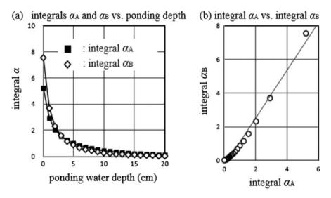
Fig. 15.9 Relationship between integral  $\alpha$  and ponding depth at A and B
