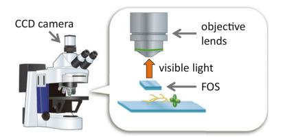
**Fig. 19.9** Microscope installed with the RRIS. The radiation from the nuclides in a sample was converted to visible light by FOS and CCD camera captured the light passed through the objective lends
