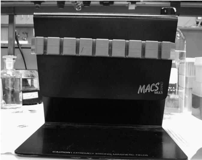
Fig. 4. Magnet stand used for the micro-bead selection.
