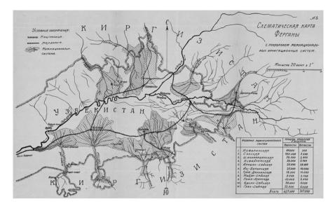
**Fig. 9.5** Schematic map of the Fergana Valley [Skhematiceskaya karta Fergany s pokazaniem mezhnatsionalnykh irrigatsionnykh sistem] showing the Soviet Union's trans-boundary irrigation system and the irrigated areas in Kyrgyzstan (107,000 dessiatines, one dessiatine equals 1.0925 ha) and Uzbekistan (427,000 dessiatines) in 1925 (Source: Bulaevskii 1925)
