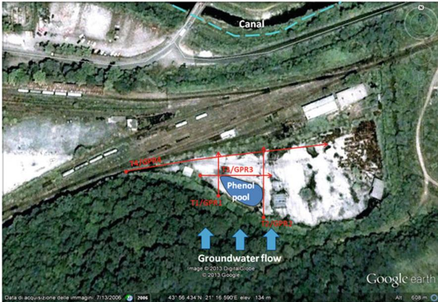
**Fig. 5** Location of the Kablova factory waste disposal area embedding the “phenol pool.” The location of ERT surveys (T1, T2, and T3) and expected groundwater flow are indicated. Copyright 2013 Digital Globe, 2013 Google (modified)
