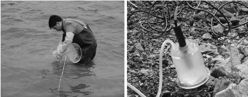
**Fig. 9.8** The left photograph shows a cylindrical sediment oxygen demand (SOD) chamber being prepared for insertion in the sediment bed, and the right photograph shows the on-shore chamber to which water is pumped from the SOD chamber for continuous monitoring of the dissolved oxygen by the probe inserted in the top of the on-shore chamber (photos by Cheng Liu)
