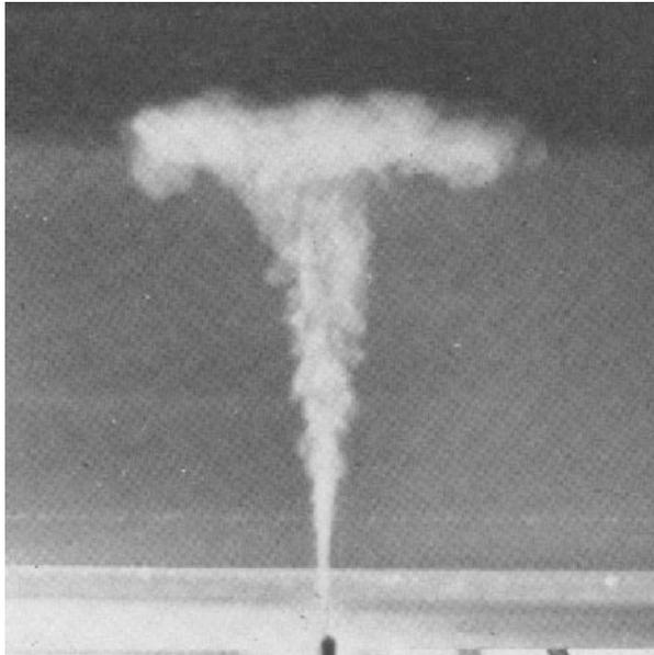
**Fig. 8.53** Buoyant jet trapped beneath the surface in stratified fluid
