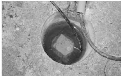
Fig. 4.70 A ground sound wave probe installed on a dam
