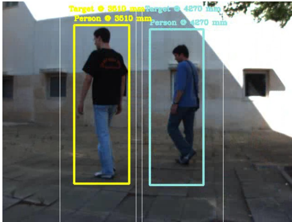
Fig. 15. The output of the system is depicted in the image as different bounding boxes from the Lidar. Between 0 and 2 meters, the bounding box of the related object is red; between 2 and 4 meters, it is yellow, and beyond 4 meters, it is light blue.
