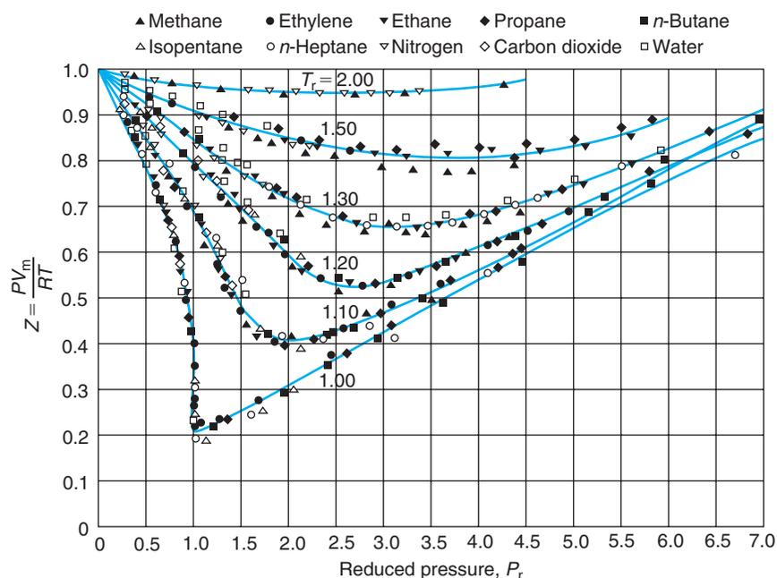
**Figure 1.9 The Compression Factor as a Function of Reduced Pressure and Reduced Temperature for a Number of Gases.** From G.-J. Su, *Ind. Eng. Chem.*, **38**, 803 (1946). Used by permission of the copyright holder.
