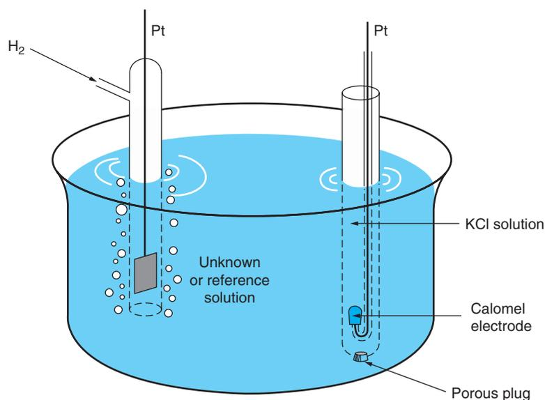
Figure 8.10 A Cell for the Measurement of pH.
