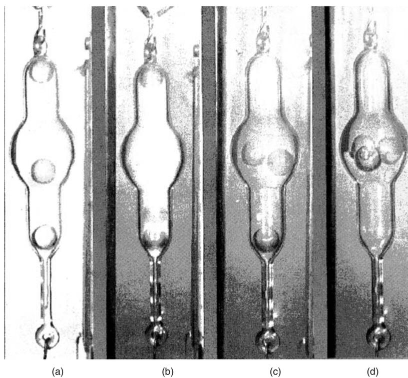
**Figure 1.6 Liquid–Gas Equilibrium near the Critical Point.** (a) At a temperature slightly above the critical temperature. The density of the fluid depends slightly on height, due to gravity. (b) At the critical temperature, and showing the scattering of light known as critical opalescence. (c) and (d) At subcritical temperatures, showing a definite meniscus. From J. V. Sengers and A. L. Sengers, *Chem. Eng. News*, June 10, 1968, p. 104. Used by permission of the copyright holder.
