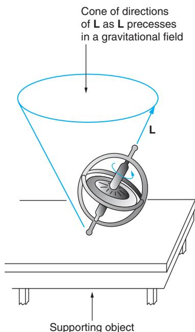
**Figure E.3 A Simple Gyroscope.** If a torque is placed on a gyroscope, as by supporting one end of the gyroscope in a gravitational field, the gyroscope will precess, which means that its axis of rotation will move around a cone with a vertical axis.
