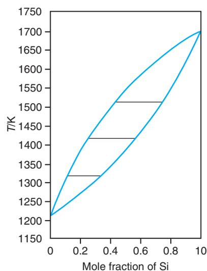
**Figure 6.6** The Solid-Liquid Temperature-Composition Phase Diagram of Silicon and Germanium. Since both the solid and liquid phases are nearly ideal solutions, this diagram resembles the liquid-vapor phase diagram of an ideal liquid solution. From C. D. Thurmond, *J. Phys. Chem.*, **57**, 827 (1953).
