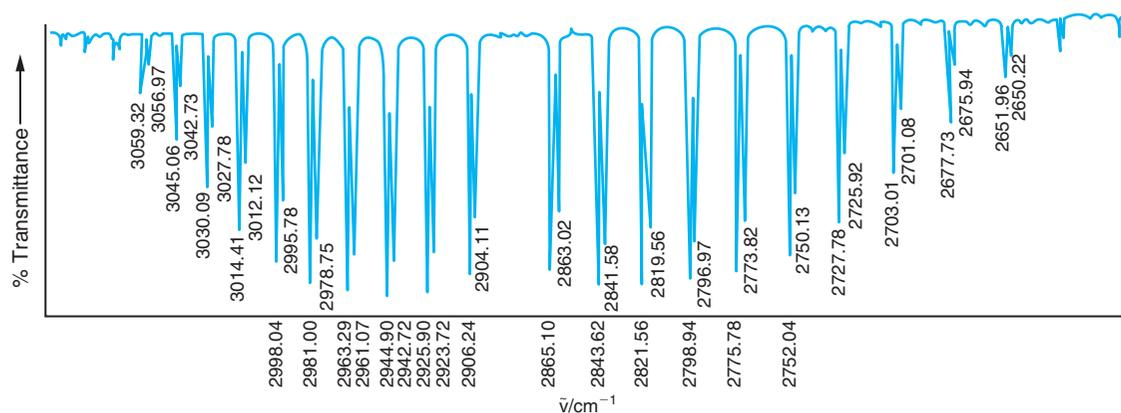
**Figure 23.9** The Fundamental Band of the Vibration–Rotation Spectrum of HCl. The resolution of the spectrum is sufficient to show the lines for  $\text{H}^{35}\text{Cl}$  and  $\text{H}^{37}\text{Cl}$ . The  $^{35}\text{Cl}$  is the more abundant isotope of chlorine, and produces the more intense lines. From N. L. Alpert, W. E. Keiser, and H. A. Szymanski, *IR Theory and Practice of Infrared Spectroscopy*, 2nd ed., Plenum Press, New York, 1970.
