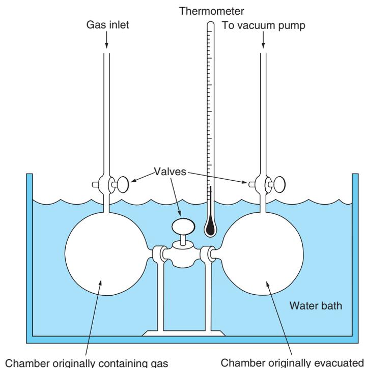
**Figure 2.5** The Apparatus for the Joule Experiment (Schematic).
