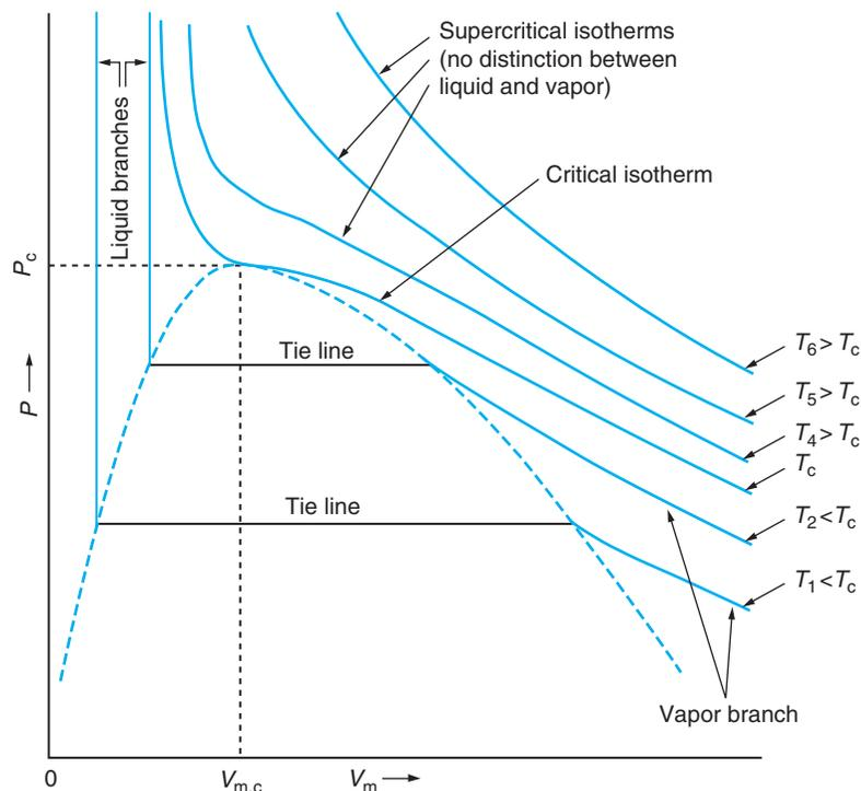
Figure 1.5 Isotherms for a Typical Pure Substance (Schematic).
