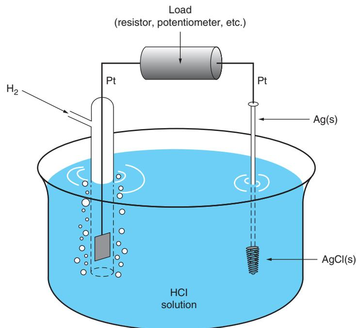
Figure 8.2 An Electrochemical Cell.
