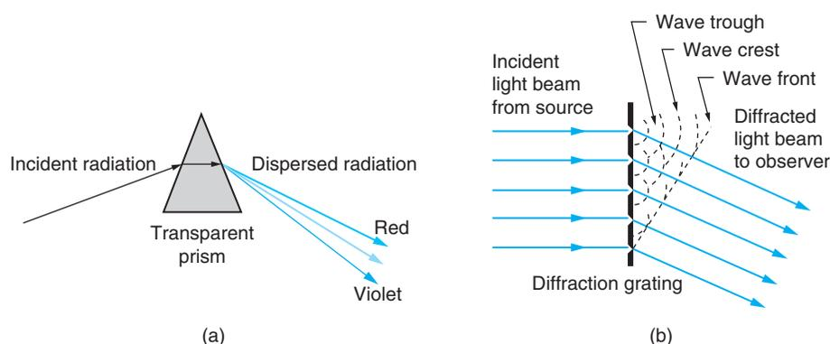
**Figure 23.1** The Dispersion of Electromagnetic Radiation. (a) Prism. Since the refractive index depends on wavelength, different wavelengths are refracted through different angles. (b) Transmission grating. Since constructive interference is necessary to give the diffracted beam, different wavelengths are diffracted through different angles.
