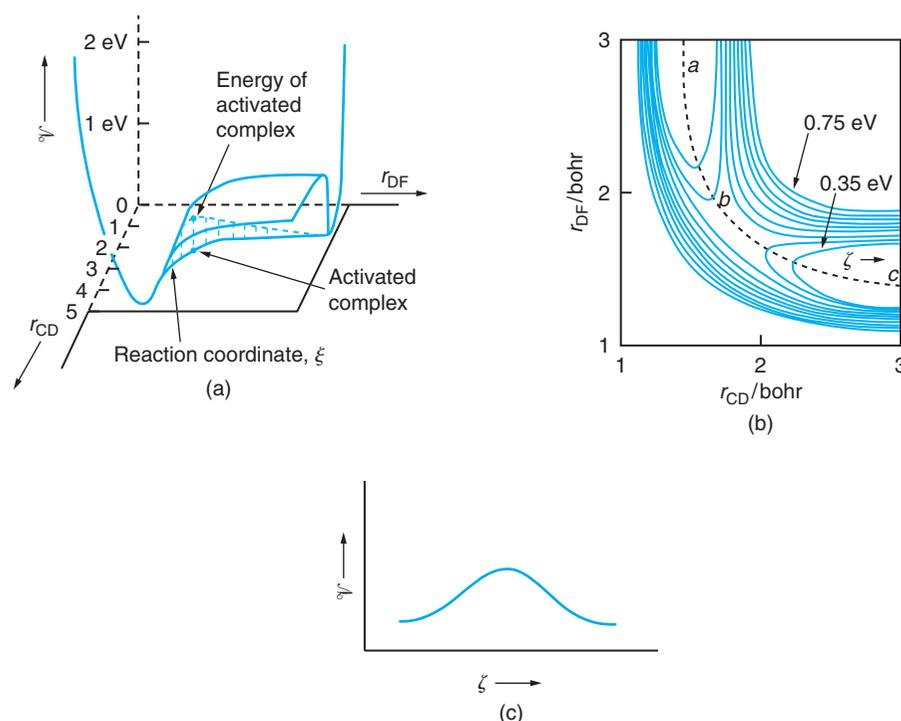
**Figure 26.1 Potential Energy Surface of H<sub>3</sub> for Linear Geometry.** (a) Perspective view of the surface (schematic). (b) Contours of constant potential energy for H<sub>3</sub>. From R. D. Levine and R. B. Bernstein, *Molecular Reaction Dynamics and Chemical Reactivity*, Oxford University Press, New York, 1987, p. 124. (c) Potential energy along the reaction coordinate.
