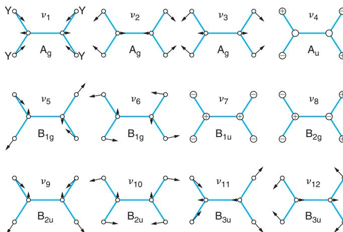
**Figure 23.18** The Vibrational Normal Modes of Ethylene,  $C_2H_4$ . The arrows show the direction of motion of each nuclei in one-half of the period. The length of each arrow is proportional to the amplitude of motion of the nucleus. From G. Herzberg, *Molecular Spectra and Molecular Structure, Vol. II, Infrared and Raman Spectra of Polyatomic Molecules*, Van Nostrand Reinhold, New York, 1945, p. 107.
