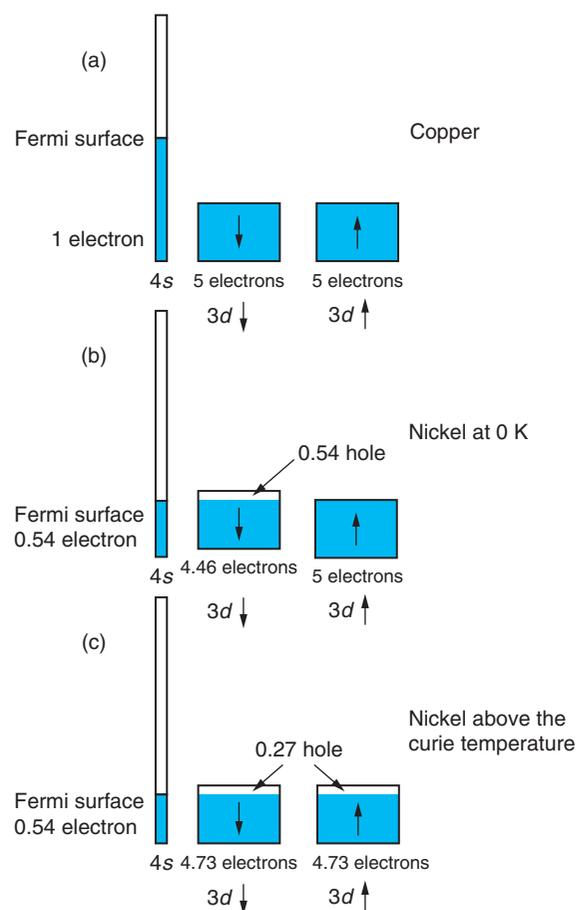
**Figure 28.14 The 4s and 3d Bands of Nickel and Copper.** The vertical axis in each diagram represents the electronic energy. From N. B. Hannay, *Solid-State Chemistry*, Prentice-Hall, Englewood Cliffs, NJ, 1967, p. 38.
