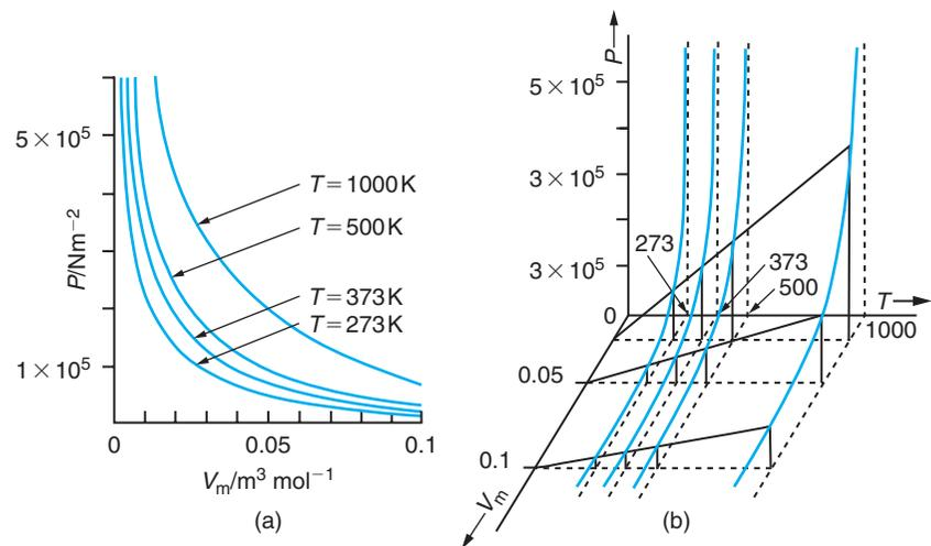
**Figure 1.1** (a) The pressure of an ideal gas as a function of  $V$  at constant  $n$  and various constant values of  $T$ . (b) The pressure of an ideal gas as a function of  $V$  and  $T$  at constant  $n$ .
