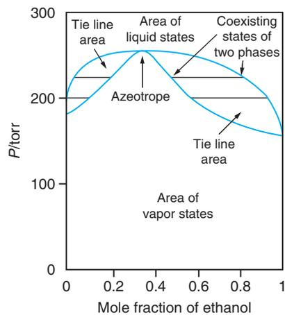
**Figure 6.13** Liquid–Vapor Pressure–Composition Phase Diagram of Ethanol and Benzene, Showing an Azeotrope. Drawn from data in J. Timmermans, *Physicochemical Constants of Binary Systems*, Vol. 2, Interscience Publishers, New York, 1959, p. 61.
