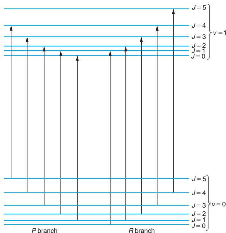
**Figure 23.8 Allowed Transitions Leading to a Vibration–Rotation Spectral Band of a Diatomic Substance.** In the  $R$  branch, the value of  $J$  in the upper level is greater than that in the lower level, and in the  $P$  branch, the opposite is the case. There is no  $Q$  branch, which would correspond to the same value of  $J$  in the upper and lower energy levels.
