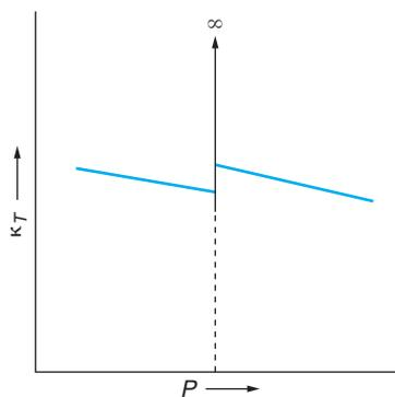
**Figure 5.10 The Isothermal Compressibility as a Function of Pressure at a First-Order Phase Transition (Schematic).** Because of the discontinuity in the molar volume as a function of pressure, there is an infinite spike in the compressibility at the phase transition.
