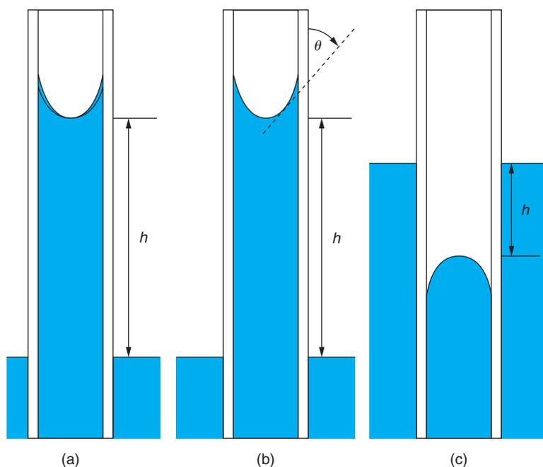
**Figure 5.17** Capillary Rise or Depression of a Liquid in a Tube. (a) A liquid that wets the solid surface. (b) A liquid that partially wets the solid surface. (c) Capillary depression of mercury in a glass capillary.
