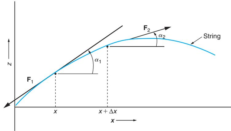
**Figure E.1** The Position of a Flexible String and the Forces on a Segment of the String. This arbitrary conformation of the string as a function of length along the string is used to describe the forces on a small segment of the string.
