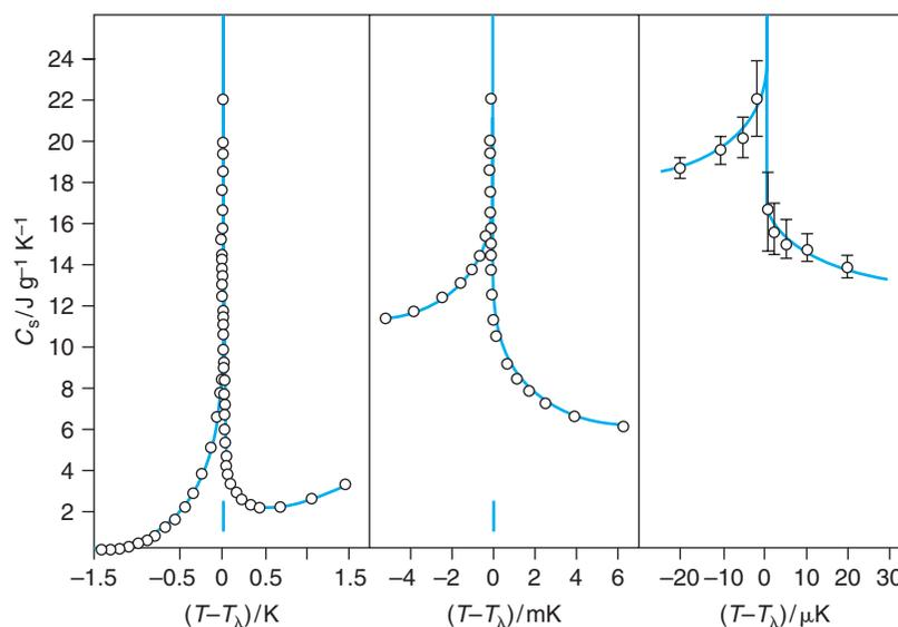
**Figure 5.13** The Heat Capacity of Helium Near the Lambda Transition. The heat capacity appears to become infinite, as in a first-order phase transition, but it rises smoothly instead of showing a spike at one point as does a first-order phase transition.
