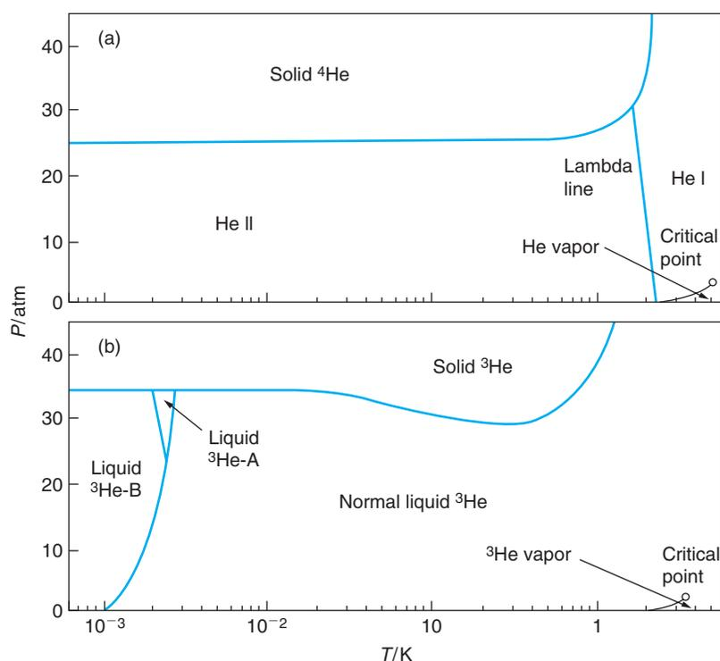
**Figure 5.4** The Low-Temperature Phase Diagrams of <sup>3</sup>He and <sup>4</sup>He. From P. V. E. McClintock, D. J. Meridith, and J. K. Wigmore, *Matter at Low Temperatures*, Wiley, New York, 1984, p. 18.
