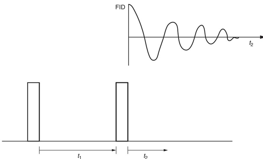
Figure 24.10 The Pulse Sequence for the COSY Experiment.
