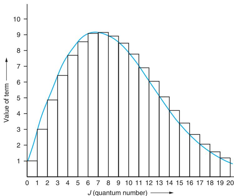
**Figure 25.4** A Graphical Representation of the Rotational Partition Function (Drawn for CO at 298.15 K). This figure is analogous to Figure 25.2 for the translational partition function. The area under the bar graph is equal to the rotational partition function for a diatomic molecule, and the area under the curve is equal to the integral approximation to the rotational partition function.
