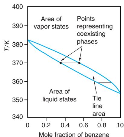
**Figure 6.3** The Liquid-Vapor Temperature-Composition Phase Diagram of Benzene and Toluene at 1.000 atm. Drawn from data of M. A. Rosanoff, C. W. Bacon, and F. W. Schulze, *J. Am. Chem. Soc.*, **36**, 1993 (1914).
