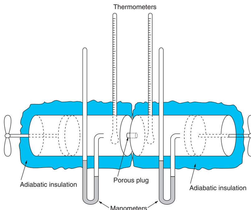
Figure 2.8 The Apparatus for the Joule–Thomson Experiment (Schematic).
