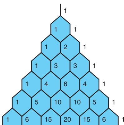
**Figure 24.2** Diagram to Find the Splittings in the ESR Spectrum of the Benzene Negative Ion,  $\text{C}_6\text{H}_6^-$ . The use of this diagram requires that all of the splitting constants are equal. Otherwise the lines will not coincide, and there will be more than seven lines.
