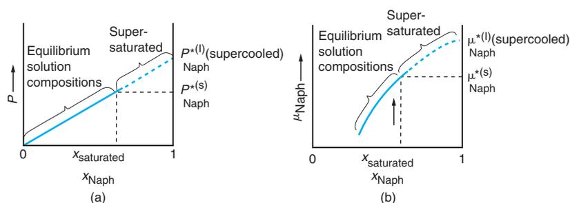
Figure 6.8 Naphthalene in an Ideal Solution (Schematic). (a) The vapor pressure as a function of composition. (b) The chemical potential as a function of composition.
