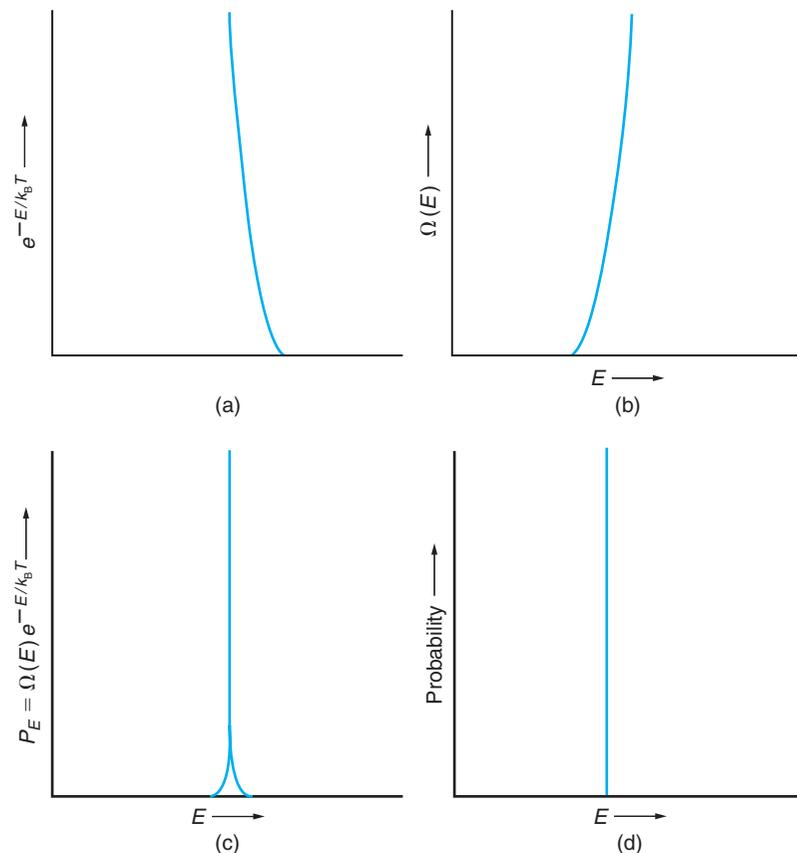
**Figure 27.2 The Probability of System States and Levels.** (a) Probability distribution of system states in the canonical ensemble as a function of energy (schematic). (b) The degeneracy of system energy levels as a function of energy (schematic). (c) The canonical probability of system energy levels as a function of energy (schematic). (d) The microcanonical probability of system energy levels as a function of energy (schematic).
