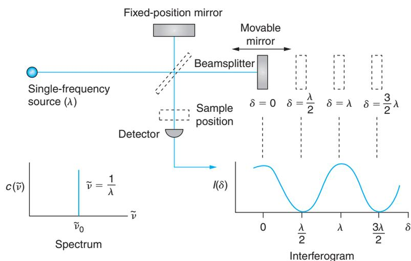
**Figure 23.10 The Radiation Path in a Fourier Transform Infrared Spectrophotometer (Schematic).** If only one wavelength is present, the sinusoidal interferogram at the lower right is observed as the movable mirror in the Michelson–Morley interferometer changes its position. The Fourier transform of this signal is a single sharp line, as shown at the lower left. From W. D. Perkins, *J. Chem. Educ.*, **63**, A5 (1986).
