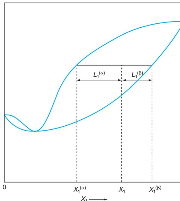
**Figure 6.27** Phase Diagram Illustrating the Lever Rule. The lever rule is similar to the formula for levers,  $F_1L_1 = F_2L_2$ , where the  $F$ 's stand for forces and the  $L$ 's stand for the lengths of the lever arms.
