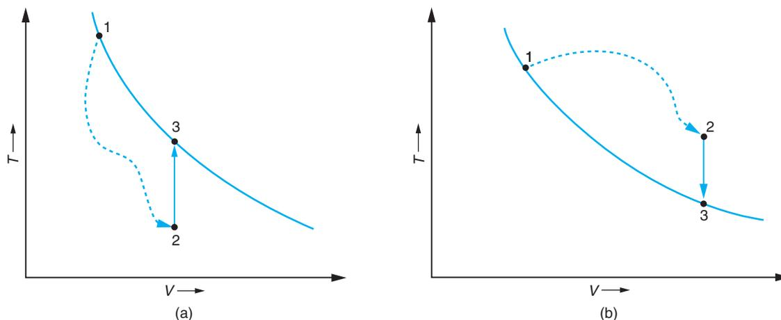
**Figure 3.7 Reversible and Irreversible Adiabats.** (a) Impossible case. An irreversible adiabatic process cannot lead to the low-temperature side of the reversible adiabat. (b) Possible case. The irreversible adiabatic process can lead to the high-temperature side of the reversible adiabat.
