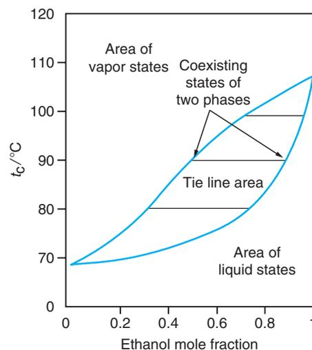
**Figure 6.12 Temperature-Composition Phase Diagram for Diethyl Ether-Ethanol at 1.84 atm.** The lower curve represents the temperature as a function of mole fraction in the liquid, and the upper curve represents the temperature as a function of mole fraction in the vapor. Drawn from data in J. Timmermans, *Physicochemical Constants of Binary Systems*, Vol. 2, Interscience Publishers, New York, 1959, p. 401.
