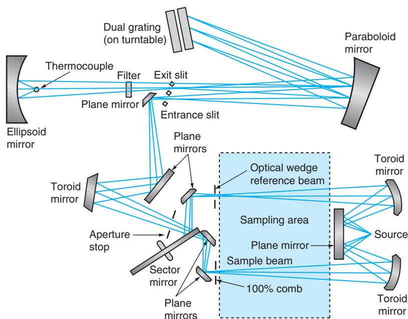
**Figure 23.3 Schematic Diagram of a Filter-Grating, Double-Beam Infrared Spectrophotometer.** This diagram shows a scanning instrument. The wavelength passed is determined by the angular position of the grating, which is mounted on a turntable, and is rotated automatically by a motor. Courtesy of Perkin-Elmer Corporation.
