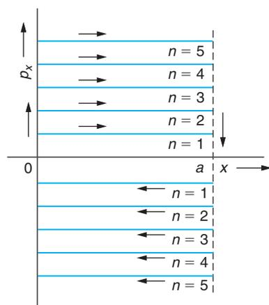
**Figure 27.3** Several Trajectories in a Two-Dimensional Phase Space for a Particle in a Hard One-Dimensional Box.
