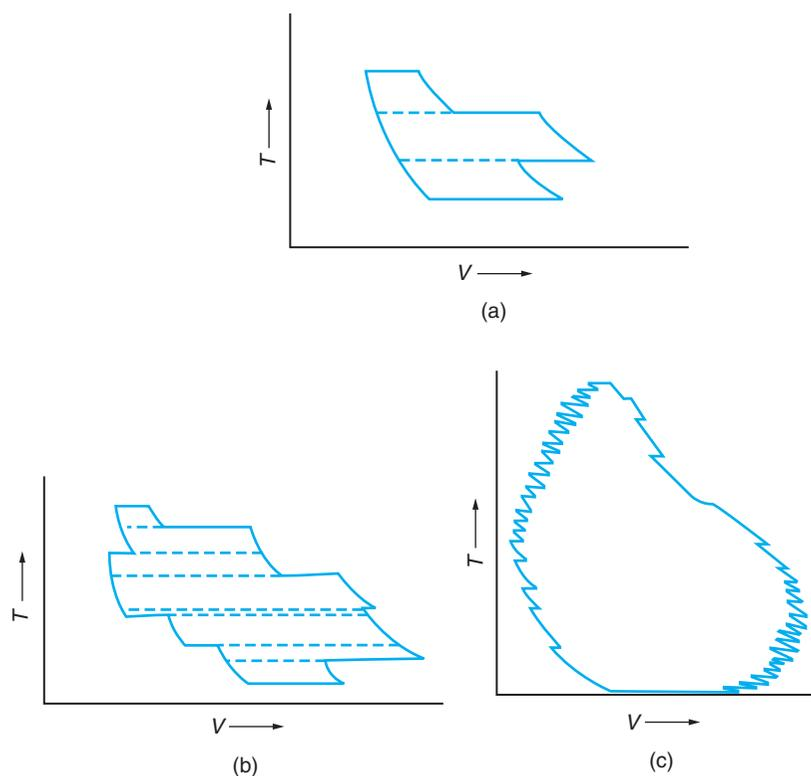
**Figure 3.5 Reversible Cycles of Isotherms and Adiabats.** (a) A cycle equivalent to three Carnot cycles. (b) A cycle equivalent to eight Carnot cycles. (c) A cycle equivalent to a large number of Carnot cycles.
