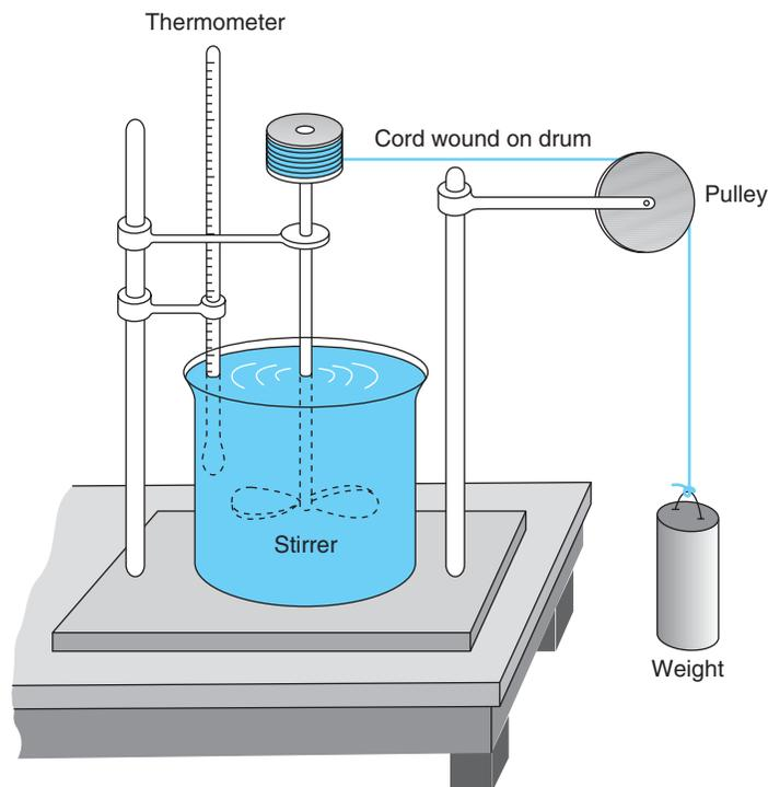
Figure 2.4 Joule's Apparatus for Determining the Mechanical Equivalent of Heat (Schematic).
