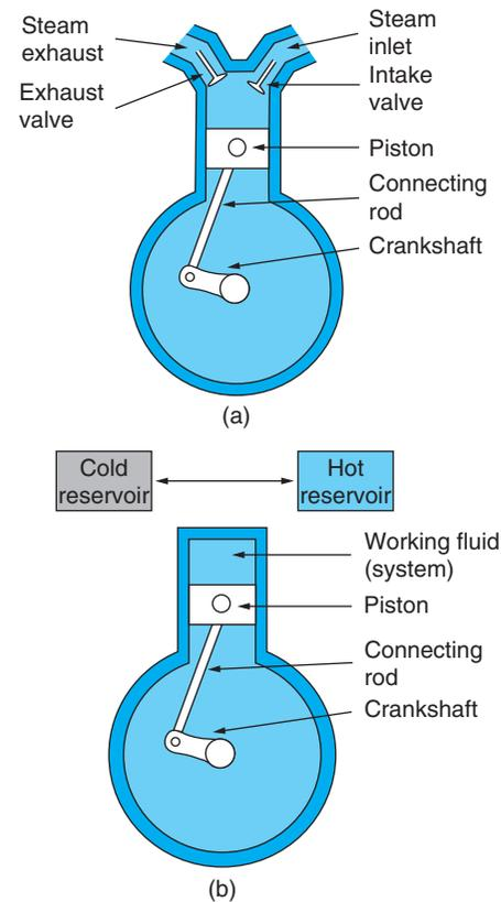
**Figure 3.1 Comparison of a Simple Steam Engine and a Carnot Engine (Schematic).**
