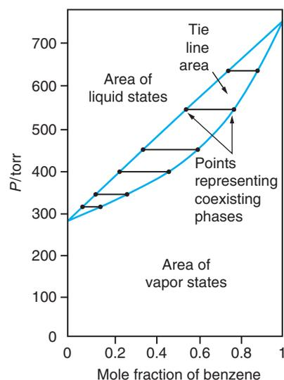
**Figure 6.2** The Liquid–Vapor Pressure–Composition Phase Diagram of Benzene and Toluene at 80°C. Drawn from data of M. A. Rosanoff, C. W. Bacon, and F. W. Schulze, *J. Am. Chem. Soc.*, **36**, 1993 (1914).
