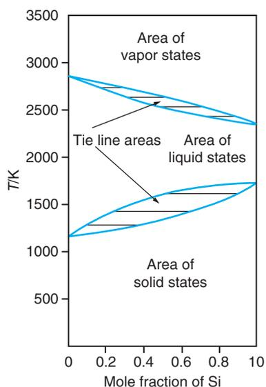
Figure 6.7 The Solid-Liquid and Liquid-Vapor Phase Diagram of Silicon and Germanium (Schematic).
