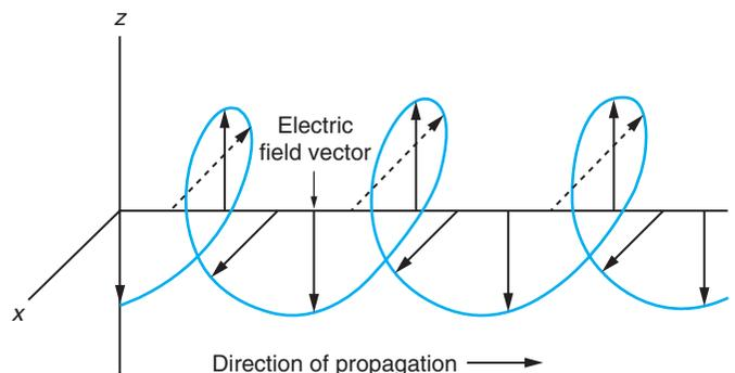
**Figure 23.21** Circularly Polarized Light from Plane-Polarized Light. The circularly polarized light corresponds to the electric field vector moving in a helical pattern.
