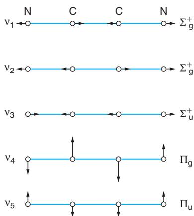
**Figure 23.14 The Vibrational Normal Modes of Cyanogen,  $\text{C}_2\text{N}_2$ .** The arrows show the directions of motion of the nuclei during half of the period of vibration, and the lengths are proportional to the amplitudes of the nuclear oscillations. From G. Herzberg, *Molecular Spectra and Molecular Structure, Vol. II, Infrared and Raman Spectra of Polyatomic Molecules*, Van Nostrand Reinhold Co., New York, 1945, p. 181.
