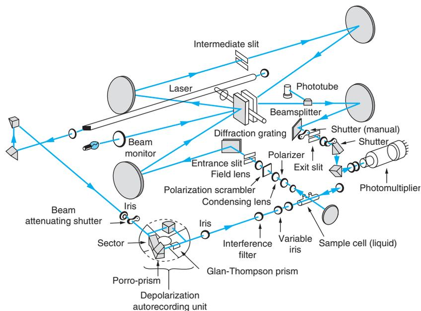
**Figure 23.17 Schematic Diagram of a Laser Raman Spectrophotometer.** In the diagram, there are two distinct beams: the incident beam, and the scattered beam at right angles to the incident beam. Courtesy of Jeol, Ltd.
