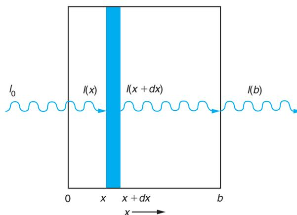
**Figure 23.4 Absorption of Light in a Thin Slab.** The attenuation of the light due to the absorbing substance in the thin slab is assumed to be proportional to the concentration of the substance and to the thickness of the slab.
