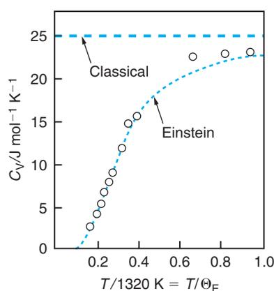
**Figure 28.7 The Heat Capacity of Diamond Fit to the Einstein Crystal Model Result.** The horizontal line corresponds to the law of Dulong and Petit. From J. S. Blakemore, *Solid State Physics*, 2nd ed., W. B. Saunders, Philadelphia, 1974, p. 121.
