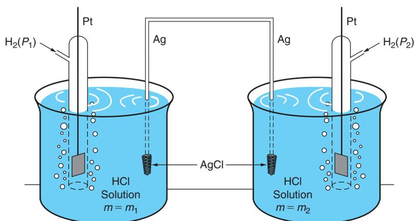
Figure 8.9 A Double Cell Equivalent to a Concentration Cell.
