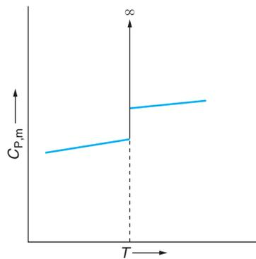
**Figure 5.9 The Constant-Pressure Heat Capacity as a Function of Temperature at a First-Order Phase Transition.** Because of the discontinuity in the entropy as a function of temperature, there is an infinite spike in the heat capacity at the phase transition.
