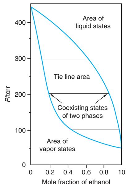
**Figure 6.11 Pressure-Composition Phase Diagram for Diethyl Ether-Ethanol at 20°C.** The lower curve shows the pressure as a function of mole fraction in the vapor, and the upper curve shows the pressure as a function of mole fraction in the liquid. Drawn from data in J. Timmermans, *Physicochemical Constants of Binary Systems*, Vol. 2, Interscience Publishers, New York, 1959, p. 401.
