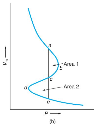
**Figure 5.15** The Pressure and the Molar Volume for a Fluid Obeying an Equation of State Such as the van der Waals Equation (Schematic). (a) The pressure as a function of molar volume. (b) The molar volume as a function of pressure.
