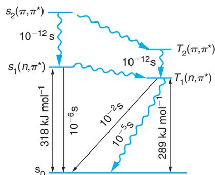
**Figure 23.15 Some Energy Levels of the Benzophenone Molecule.** The wavy arrows represent radiationless transitions, and the straight arrows represent emissions of photons. The times shown are relaxation times for the transitions. Data from D. L. Pavia, G. M. Lampman, and G. S. Kriz, Jr., *Introduction to Organic Laboratory Techniques*, 2nd ed., Saunders College Publishing, Philadelphia, 1982, p. 364.
