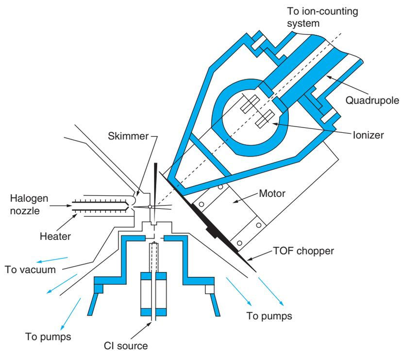
**Figure 13.22 A Crossed-Molecular Beam Apparatus (Schematic).** From R. D. Levine and R. B. Bernstein, *Molecular Reaction Dynamics and Chemical Reactivity*, Oxford University Press, New York, 1987, p. 234.
