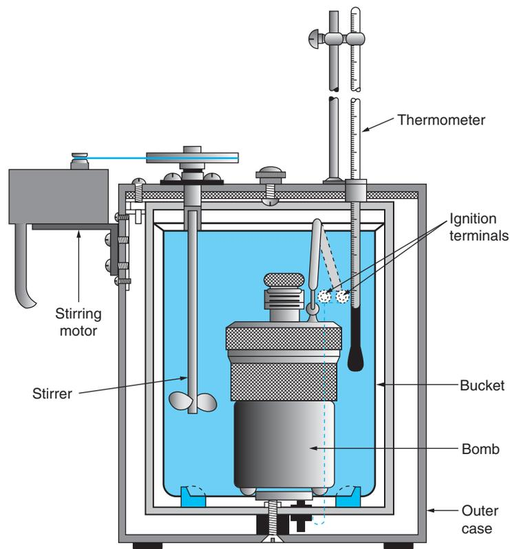
Figure 2.12 A Bomb Calorimeter. (Courtesy of the Parr Instrument Co.)
