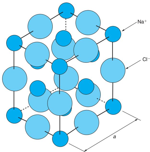
Figure 28.1 The Sodium Chloride Unit Cell.
