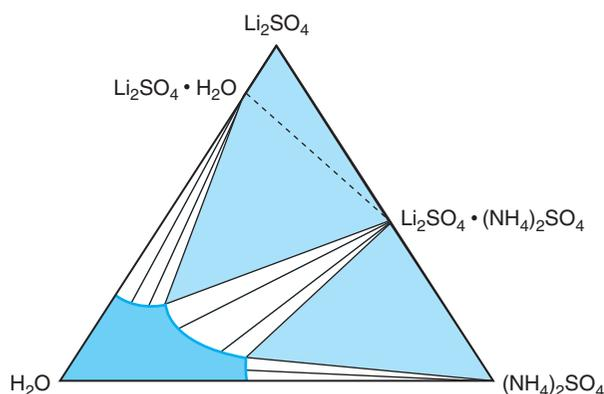
**Figure 6.25** Concentration–Concentration Phase Diagram of Lithium Sulfate, Ammonium Sulfate, and Water at 30°C and 1.000 atm. Pure lithium sulfate and ammonium sulfate are solid at this temperature.
