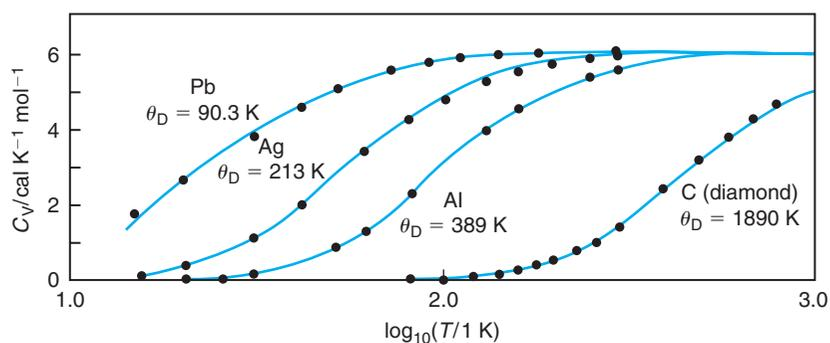
**Figure 28.9 The Heat Capacity of Several Elements as a Function of Temperature, with Debye Curves.** From G. N. Lewis and M. Randall, *Chemical Thermodynamics*, 2nd ed., rev. by K. S. Pitzer and L. Brewer, McGraw-Hill, New York, 1961, p. 56.
