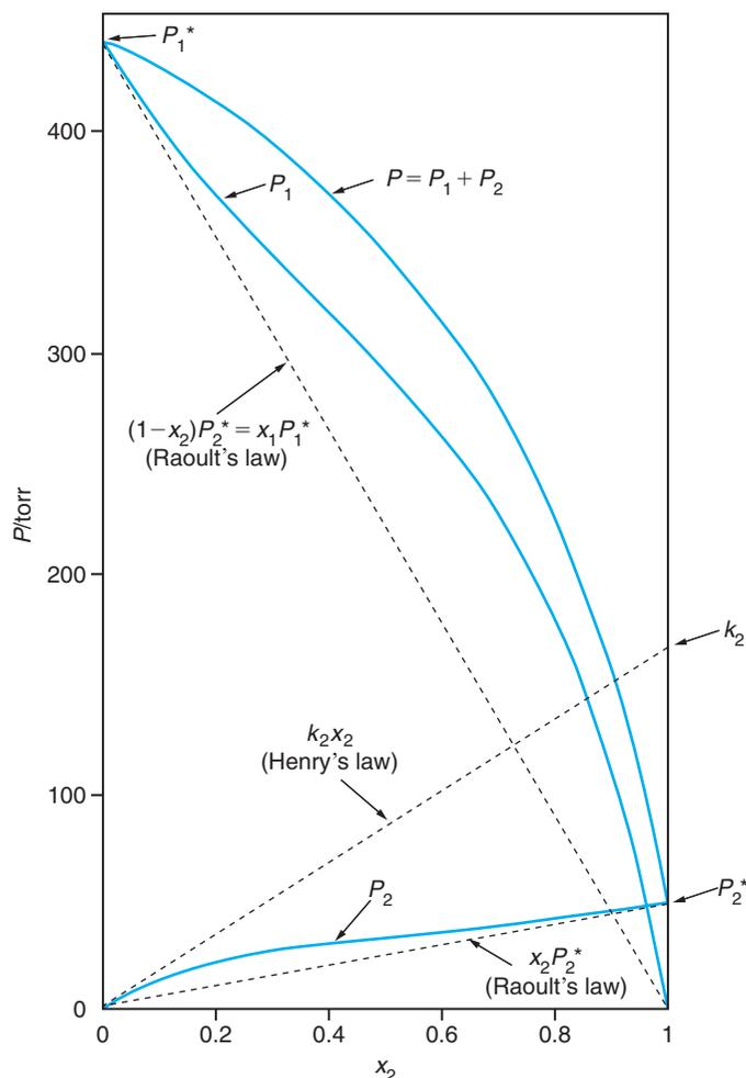
**Figure 6.9** Partial Vapor Pressures of Ethanol (Component 2) and Diethyl Ether in a Solution at 20°C, Showing Positive Deviation from Raoult's Law. Drawn from data of J. Timmermans, *Physicochemical Constants of Binary Systems*, Vol. 2, Interscience Publishers, Inc., New York, 1959, p. 401.
