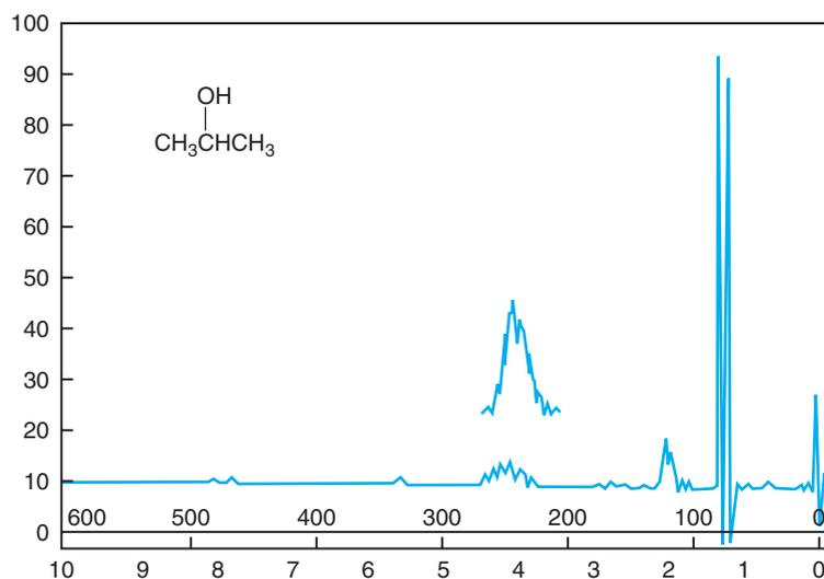
**Figure 24.5** The High-Resolution Proton NMR Spectrum of 2-Propanol Dissolved in Deuterated Chloroform. From Charles J. Pouchert and John R. Campbell, *The Aldrich Library of NMR Spectra*, The Aldrich Chemical Co., 1974, Vol. 1, p. 85.
