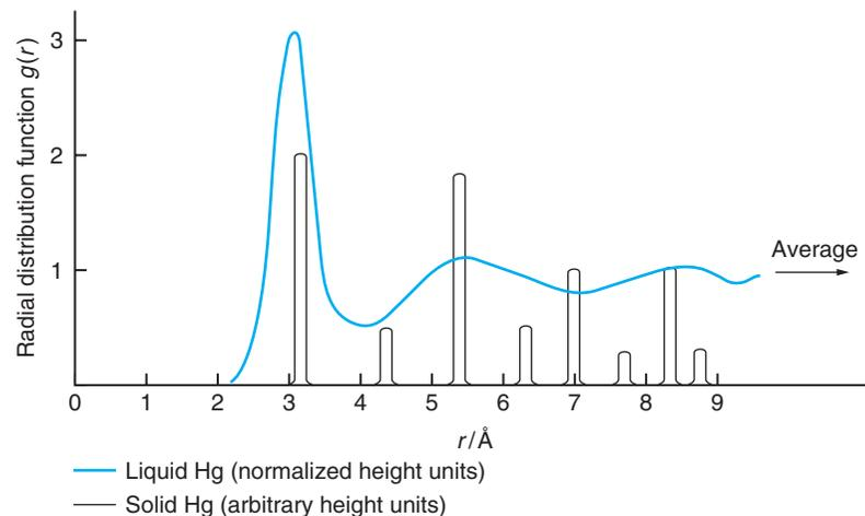
**Figure 28.16 The Radial Distribution Function of Solid and Liquid Mercury.** Since the solid has a lattice structure, the positions of neighboring atoms give narrow “blips” in the radial distribution function. In the liquid, the disorder that is present makes the function into a smooth curve, which shows vestiges of the crystal lattice. From D. Tabor, *Gases, Liquids and Solids*, 2nd ed., Cambridge University Press, Cambridge, England, 1979, p. 197.
