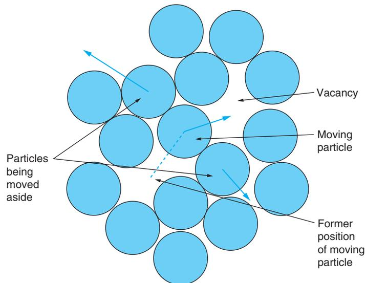
**Figure 28.17 Motion of a Molecule into a Vacancy in a Liquid.** This figure attempts to illustrate the position of maximum potential energy of a molecule moving from one shell of neighbors to another.
