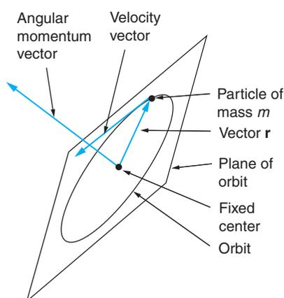
**Figure E.2** Diagram to Illustrate the Definition of the Angular Momentum Vector. The angular momentum vector,  $\mathbf{L}$ , is perpendicular to the vector  $\mathbf{r}$  and the vector  $\mathbf{v}$ , and has magnitude equal to  $m|\mathbf{r}||\mathbf{v}|$ .
