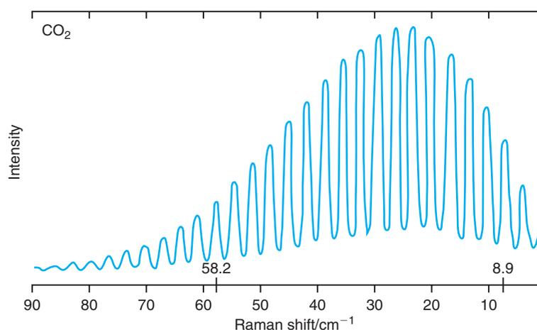
**Figure 23.19 Rotational Raman Spectrum of Carbon Dioxide.** The axis is the difference between the reciprocal wavelength of the incident and that of the scattered radiation. The peak at zero Raman shift is the scattered radiation with no change in energy of the molecules. From L. Claron Hoskins, *J. Chem. Educ.*, **54**, 642 (1977).
