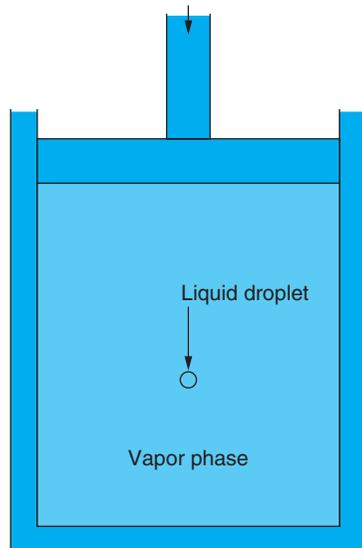
**Figure 5.18** System to illustrate the Pressure Difference in a Spherical Droplet. The droplet is surrounded by the vapor phase, and is assumed to be small enough that it does not immediately settle to the bottom of the vessel.
