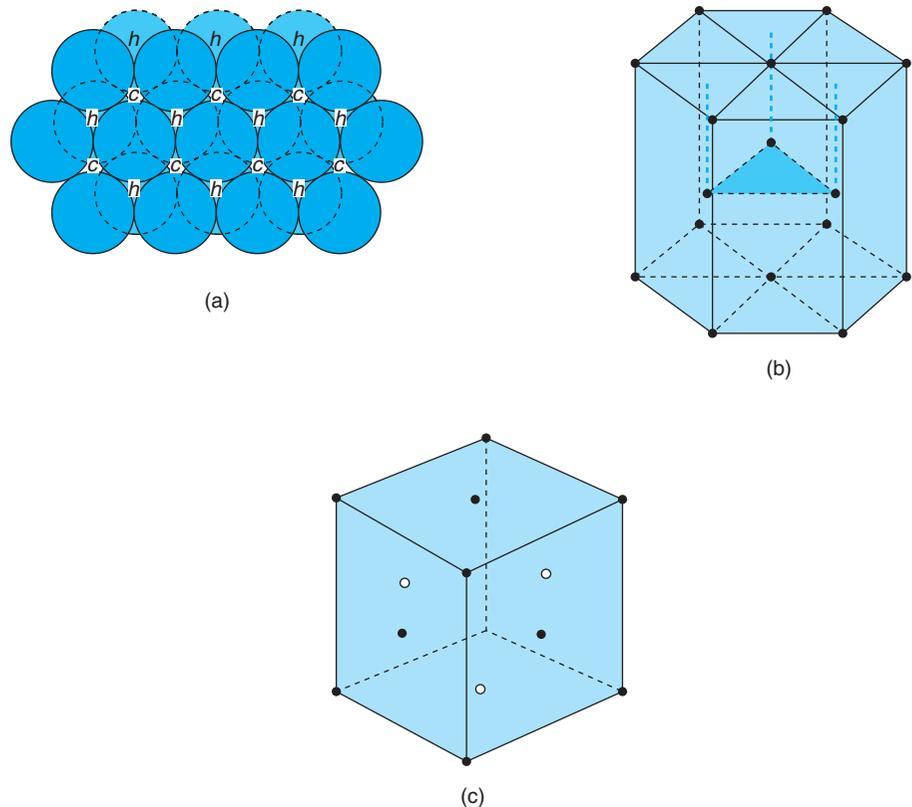
**Figure 28.3 Closest Packing of Spheres.** (a) Layers of spheres. (b) The hexagonal close-packed unit cell. This figure shows that the third layer has each sphere directly over a sphere of the first layer. (c) The face-centered cubic close-packed unit cell. This unit cell is oriented so that the layers of atoms in Figure 28.3a are parallel to a plane that passes through the lattice point at the top rear of the cell, the lower left of the cell, and the lower right of the cell.
