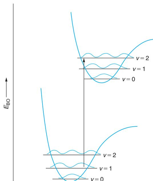
**Figure 23.11** An Electronic Transition According to the Franck-Condon Principle. In the case of this figure, a transition from the  $v = 1$  state of the lower electronic state most likely will lead to the  $v = 2$  state of the upper electronic state.
