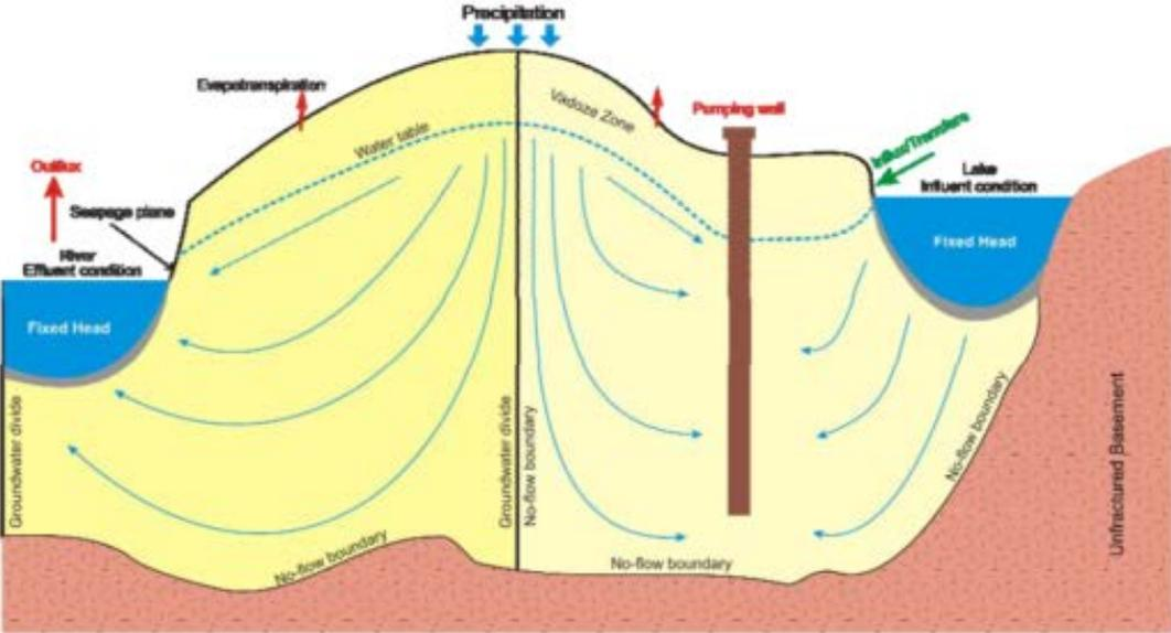
Diagram of regional groundwater flow system representing the physical and hydraulic boundary conditions.
