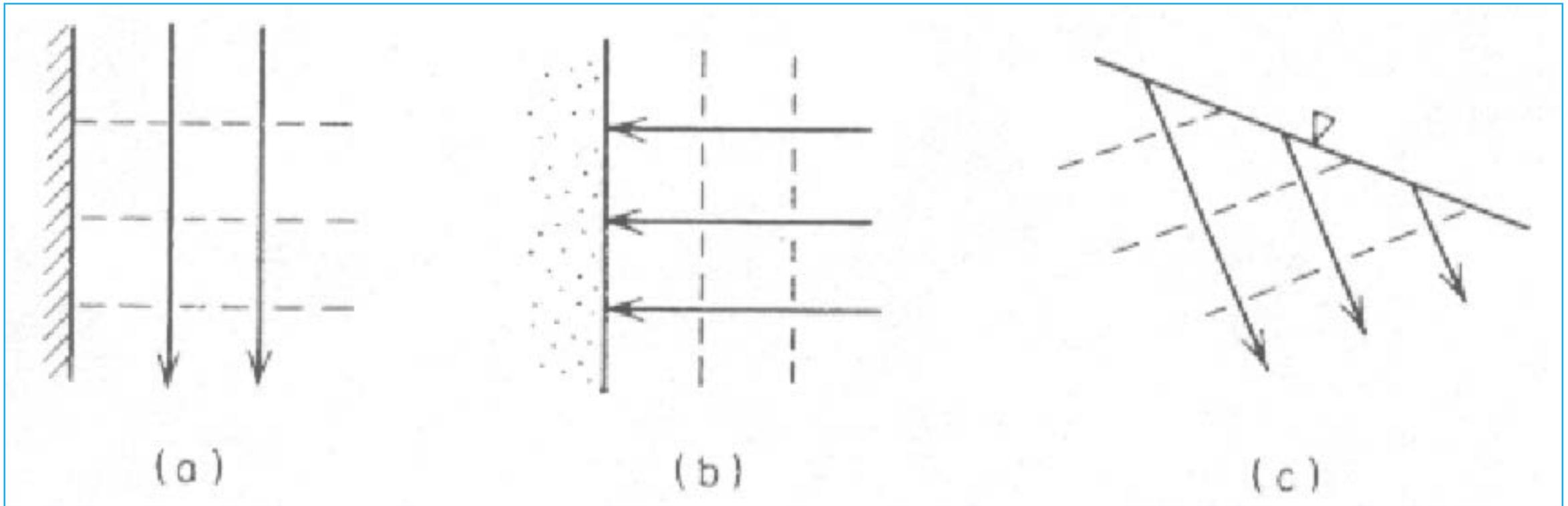
Figure. Groundwater flow in the vicinity of (a) an impermeable boundary, (b) a constant-head boundary, and (c) a water-table boundary (Freeze and Cherry, 1979)
