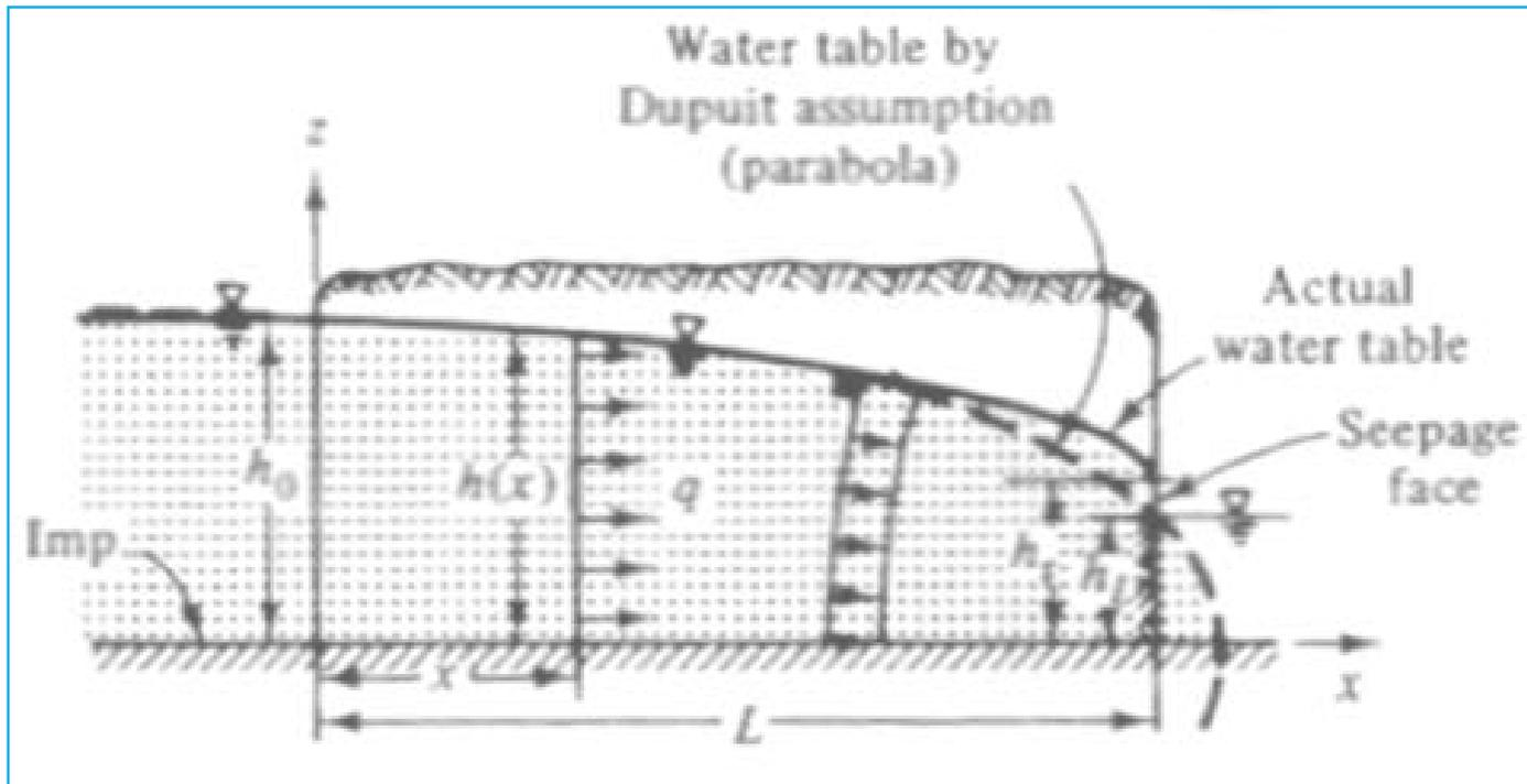
Figure. Steady unconfined flow between two reservoirs (Bear, 1979)
