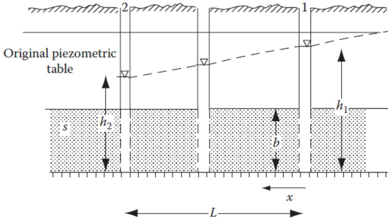
Figure. Confined aquifer with steady-flow condition
