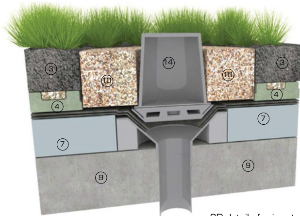
3D detail of rainwater outlet in heavily planted roof
