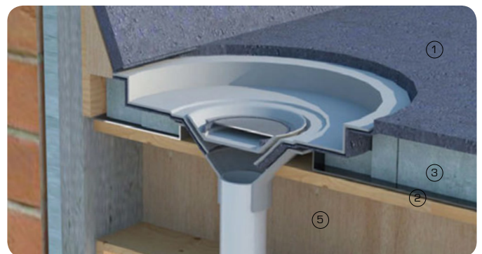
(Below) 3D view showing alternative drain outlet detail on flat timber roof arrangement
