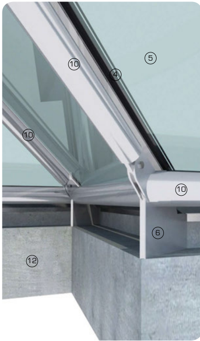
3D view showing bolt fixed glazing with external fold
