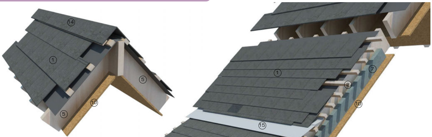
3D view showing slate tiles on unventilated timber roof at ridge
