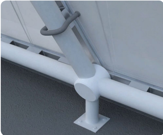
3D detail of cushion to cushion air supply
