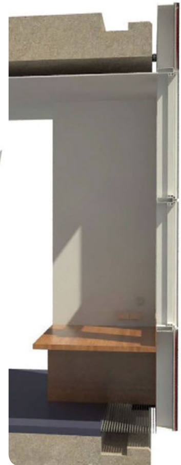
3D section showing unitised panel hung from floor slab
