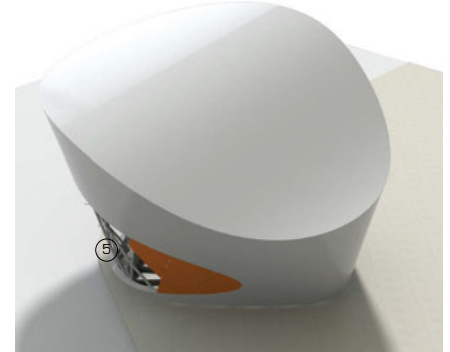
Diagram 6 Glazing panels fixed to diagrid structure using point fixings
