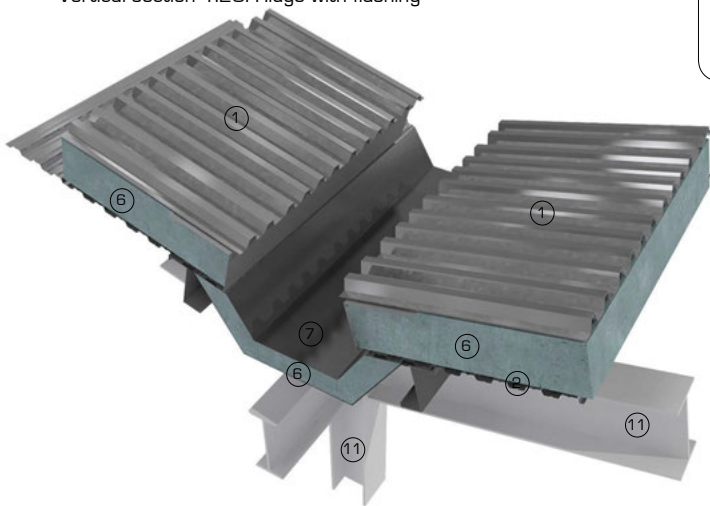
3D detail view through prefabricated valley gutter
