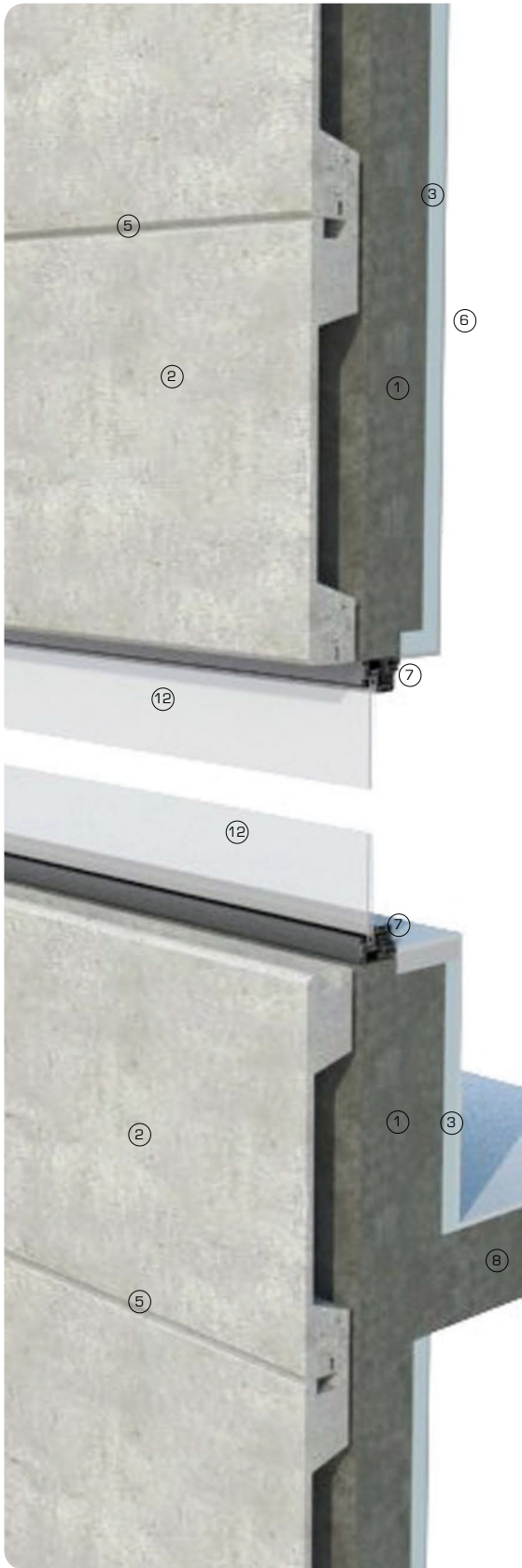
3D detail view showing typical wall assembly for GRC panels with open joints and window
