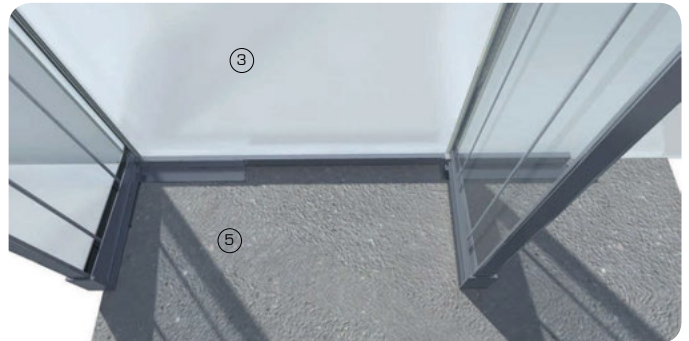
3D view looking up at interior finish at edge of glass beam and concrete base
