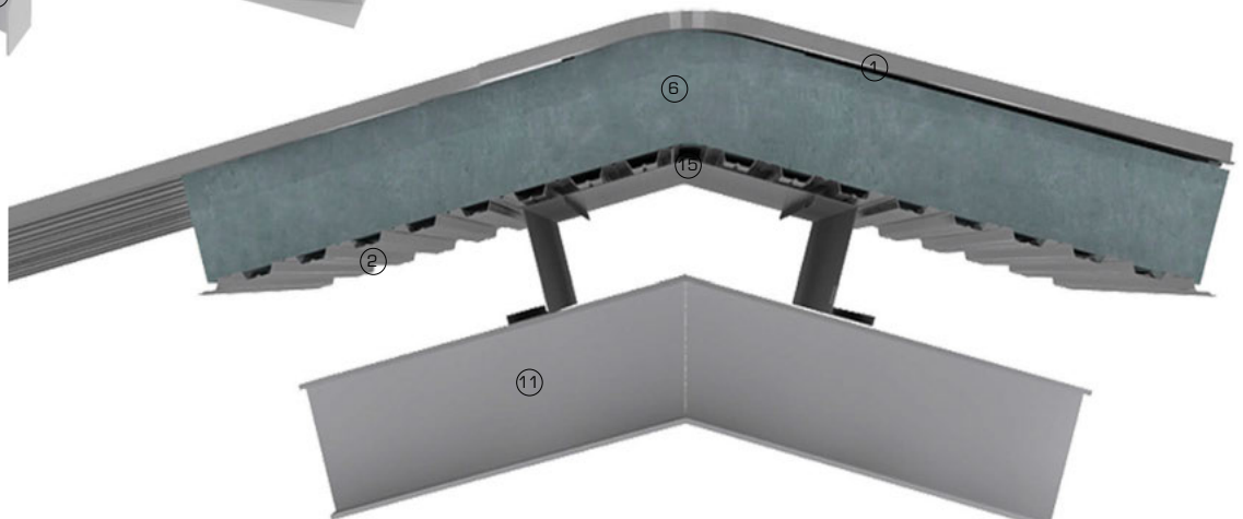
3D detail view through typical ridge construction
