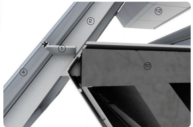
3D detail view showing inclined stick glazing system connection to floor slab
