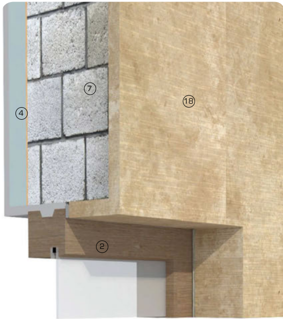
Horizontal sections 1:10. Window opening in concrete block wall illustrating application of insulation to interior or exterior of wall system
