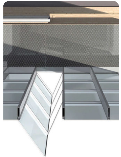
Plan view of twin wall with openable screen
