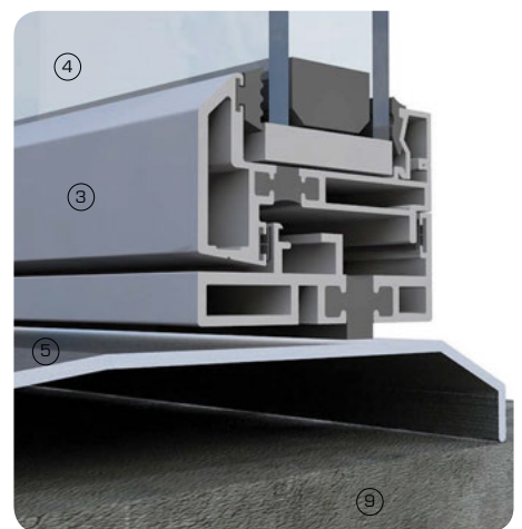
3D detail views showing details aluminium glazing system set in masonry wall at head and cill
