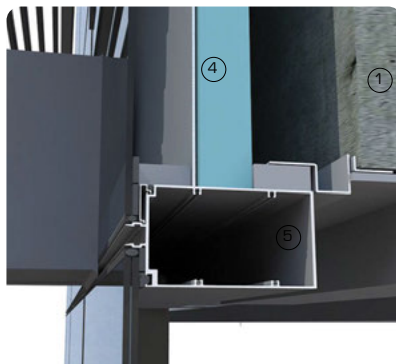
3D detail views showing unitised glazed facade with external mesh panel wall and planters at floor slab interface
