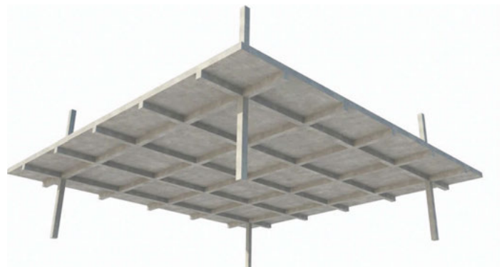
4. Two-way spanning ribbed slab
