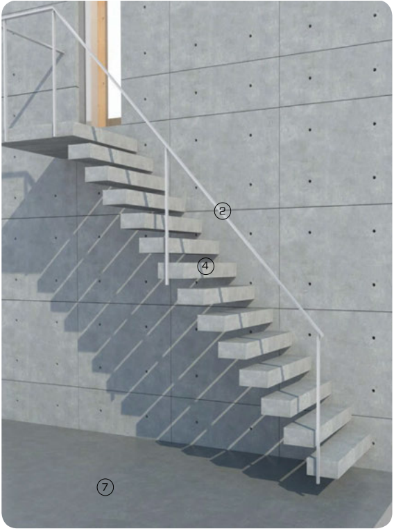
3D view showing cantilevered concrete stair configuration
