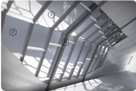
3D view showing tiled rainscreen cladding panels fixed to in-situ cast concrete primary structure
