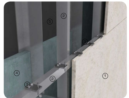
3D detail views showing stone rainscreen cladding panels fixed to in-situ cast concrete primary structure
