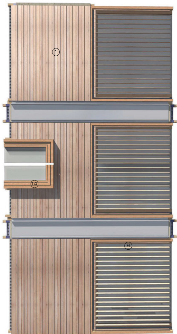
Elevation of timber cladding panels showing relationship with structural frame
