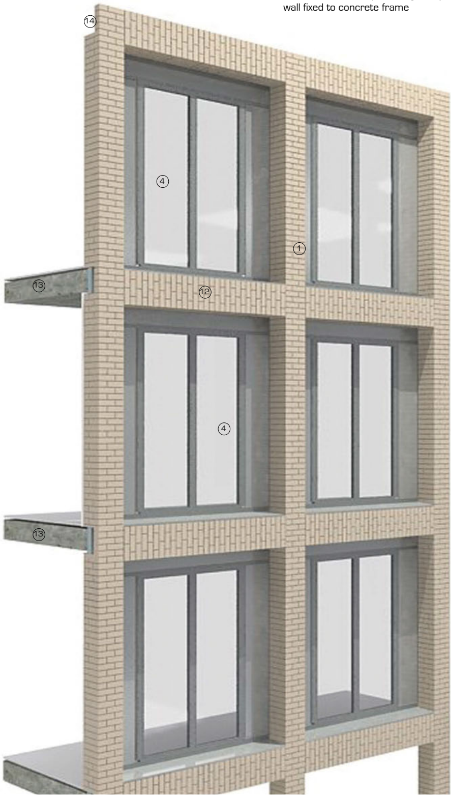
3D view of assembly showing cavity brick wall fixed to concrete frame
