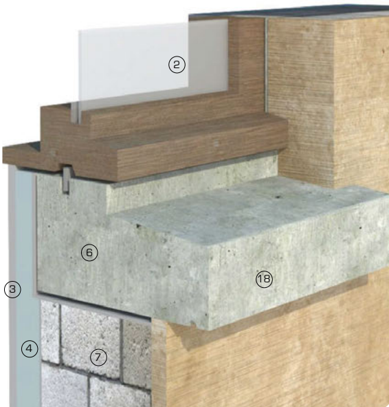
3D detail view showing window opening in typical concrete block wall, with insulation applied interior of wall system
