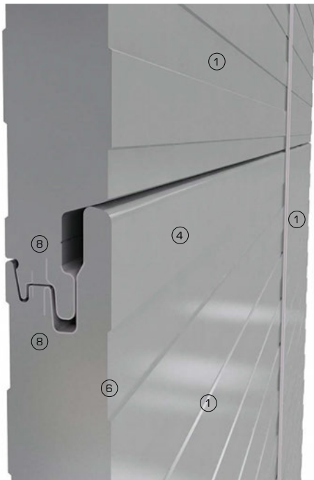
3D detail view showing connection profile for vertical two-way interlocking profiled panels
