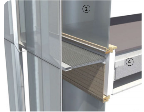
3D section cut through double skin system with openable screen
