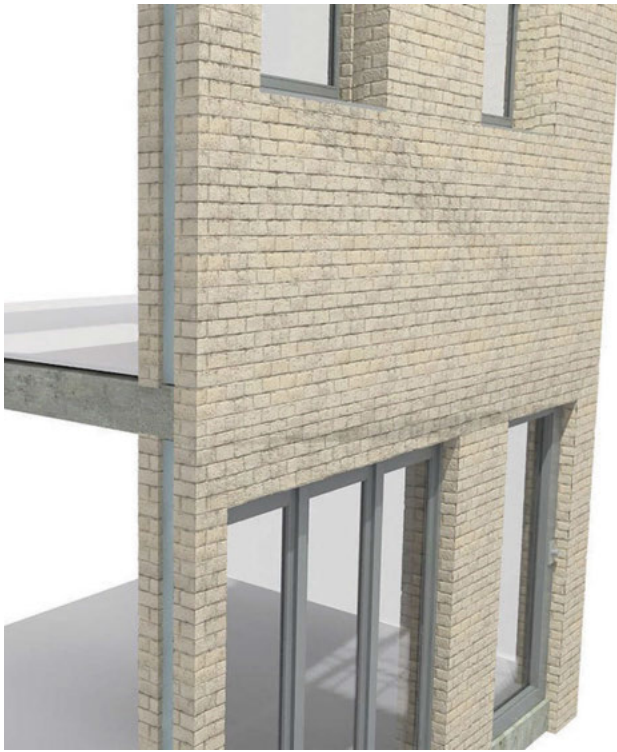
3D views of assembly showing cavity brick wall fixed to concrete frame with window and door openings
