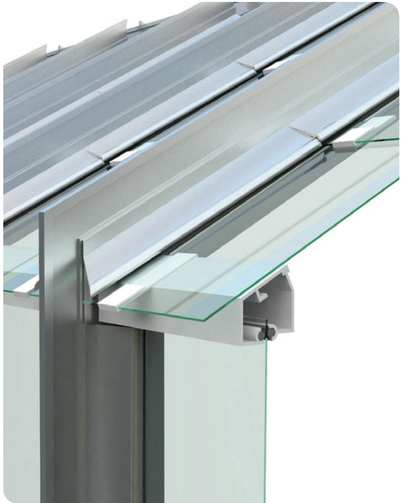
3D view of typical eaves connection
