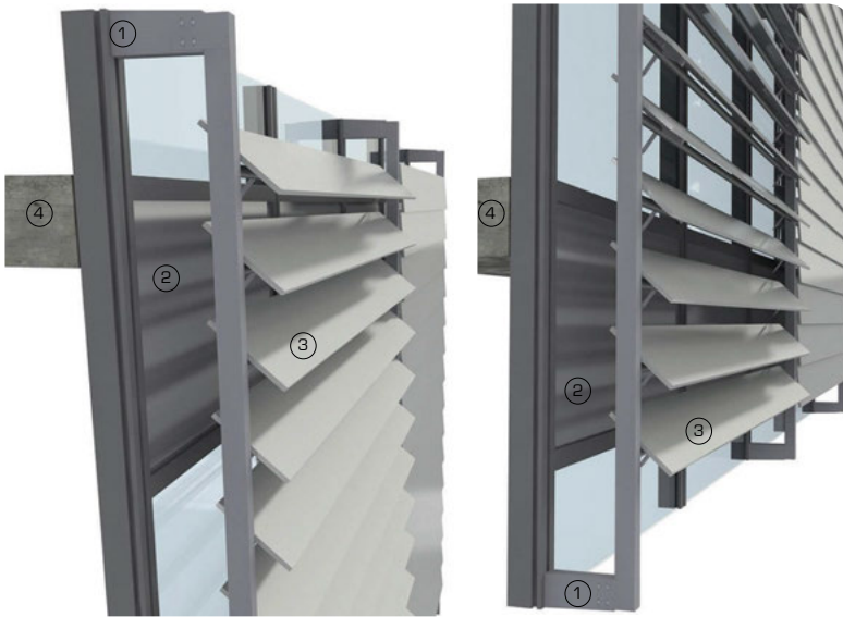
3D detail views showing louvre panel fixing details
