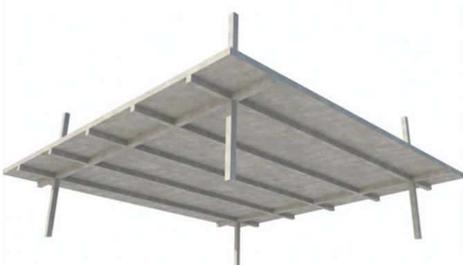
3. One-way spanning ribbed slab
