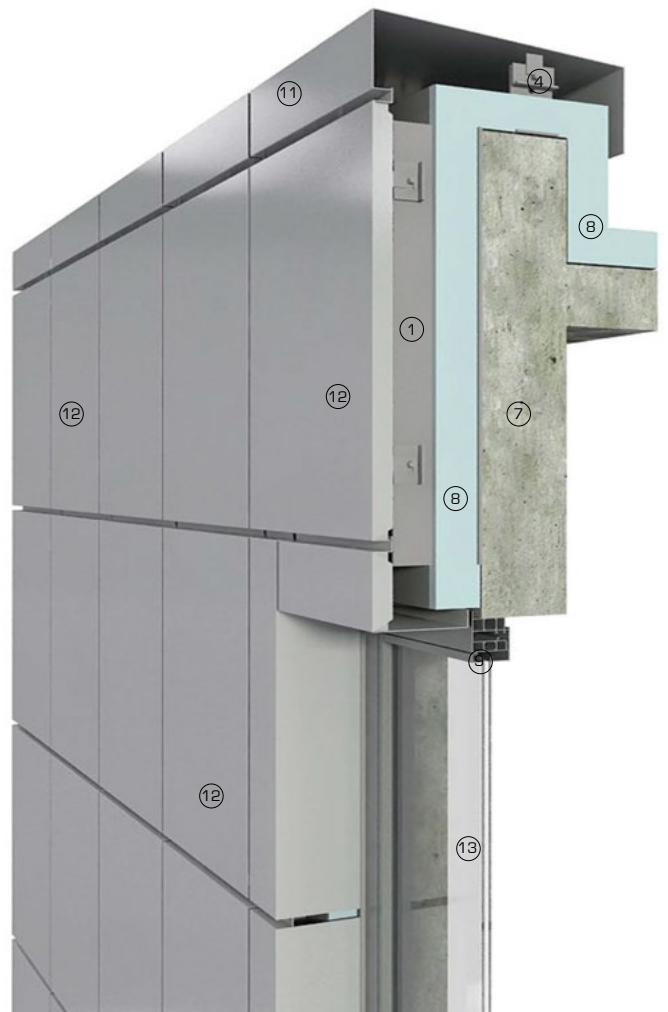
3D detail views showing window and parapet detail in rainscreen wall system
