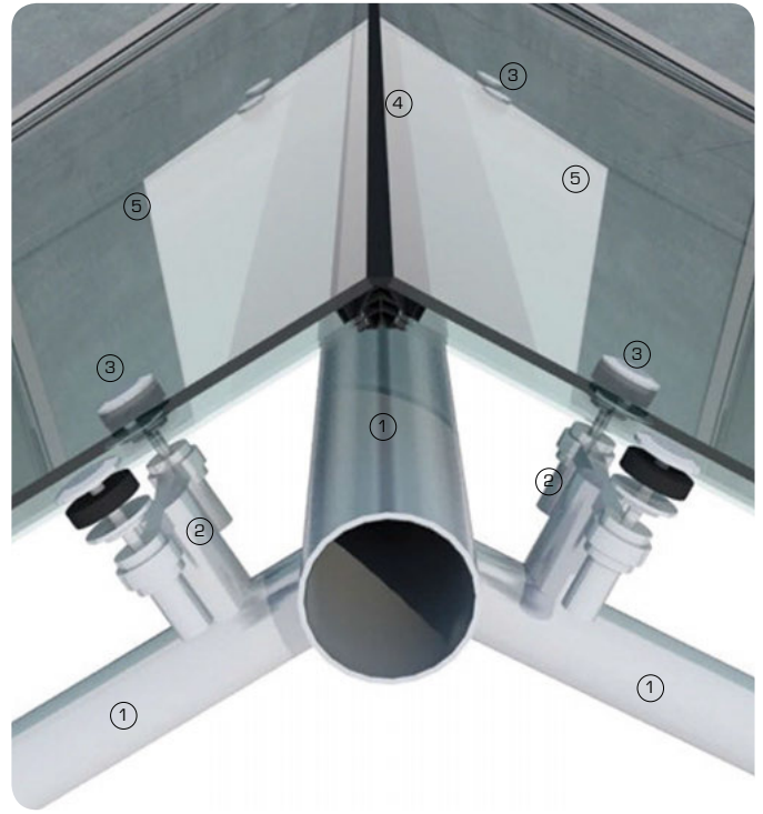
3D view showing bolt fixed glazing with external fold
