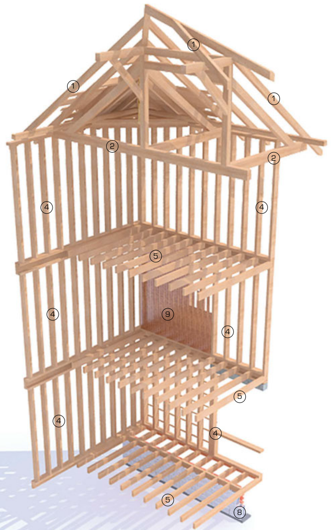
3D cutaway view showing typical timber balloon frame on a masonry base
