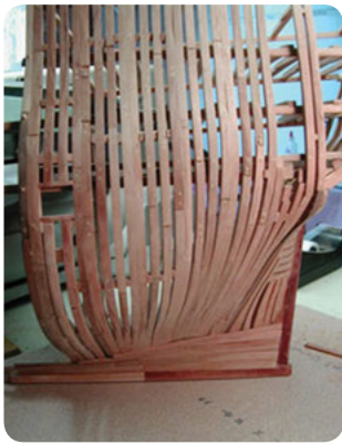
Examples showing a parallel timber technology: the construction of timber sailing ships.
