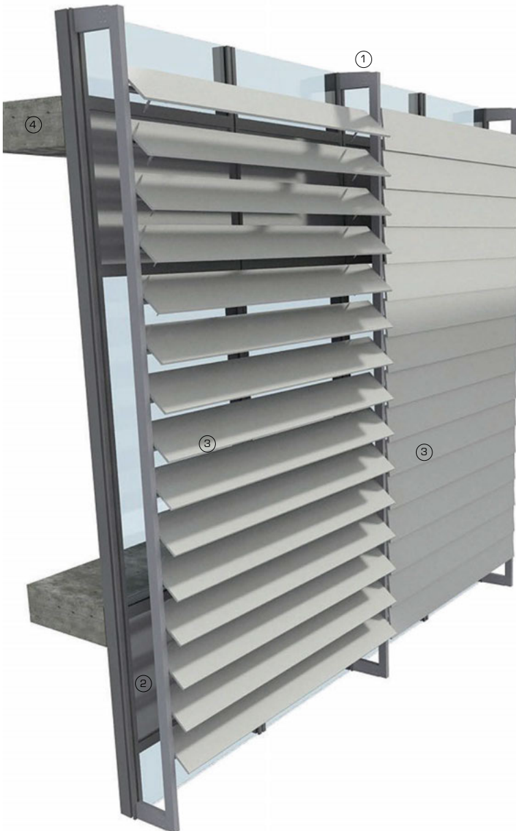
3D view showing metal louvre screen in front of curtain wall system
