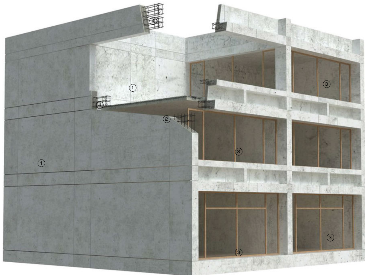
3D cutaway view showing concrete frame and steel reinforcements bars
