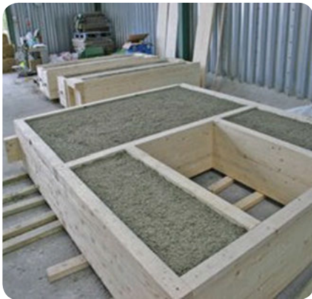
ModCell straw panel being constructed (above) and Modcell hemp (below)
