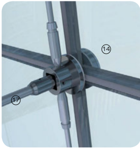
3D detail views showing cable-supported glazing system at glass clamp
