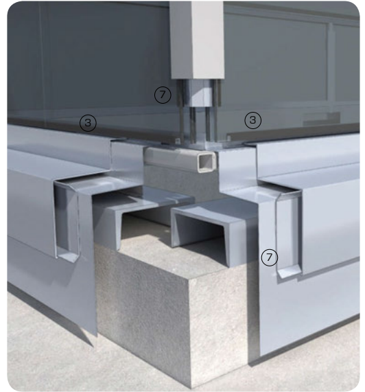
3D cutaway of typical junction with roof
