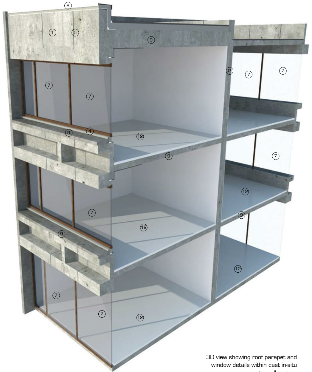
Section 1:25. In-situ cast concrete wall cast in two skins with rigid closed cell insulation between skins
