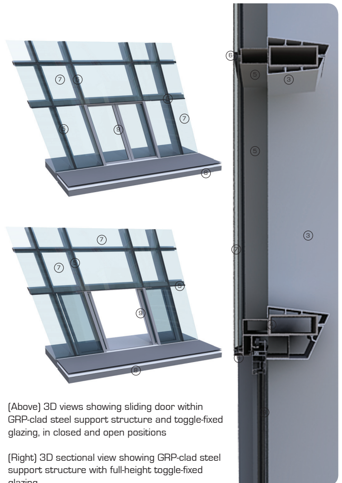
3D sectional view showing GRP-clad steel support structure with full-height toggle-fixed glazing
