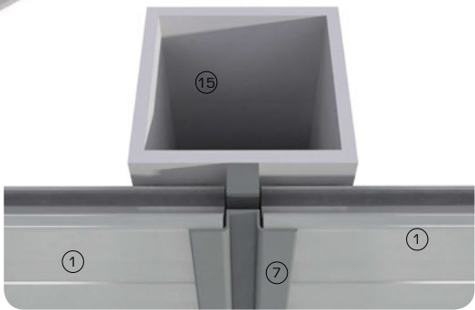
3D detail view showing metal bracket and capping fixed to structural frame
