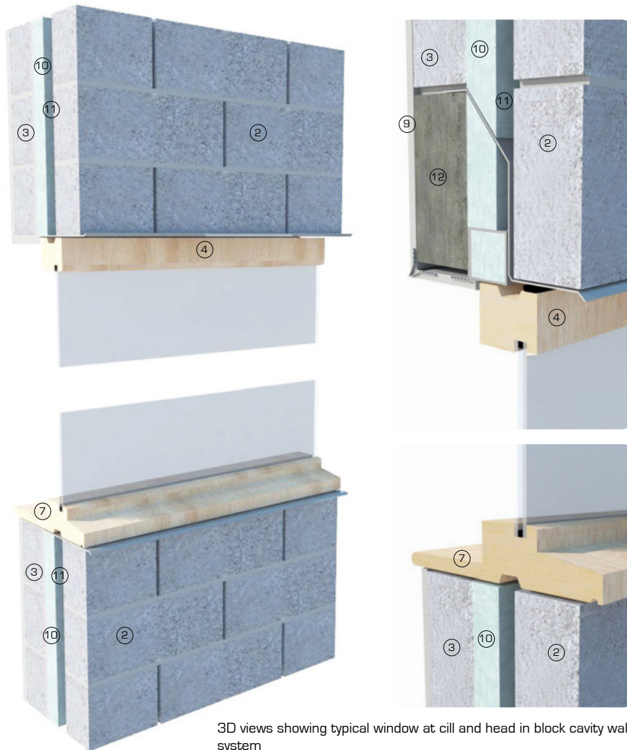
Vertical section 1:10. Typical window at cill and head in block cavity wall system
