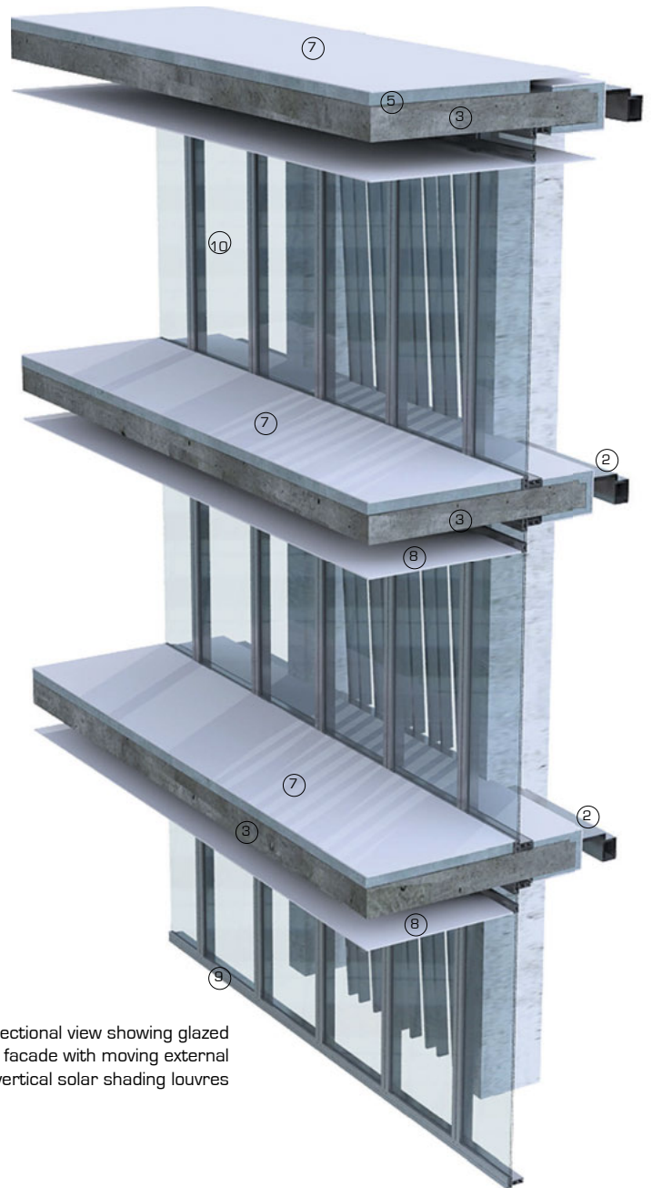
3D internal sectional view showing glazed facade with moving external vertical solar shading louvres at corner condition
