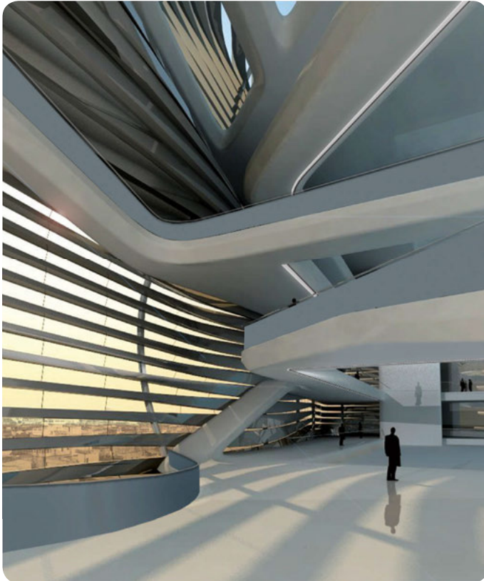
3D internal view showing full-height glazed facade with external GRP cladding over primary steel structure
