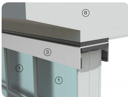
(Above) 3D view showing glass blocks supported by steel box-sections
