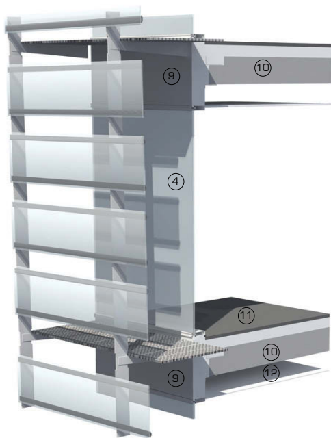
3D view of stick glazed wall with outer glazed screen
