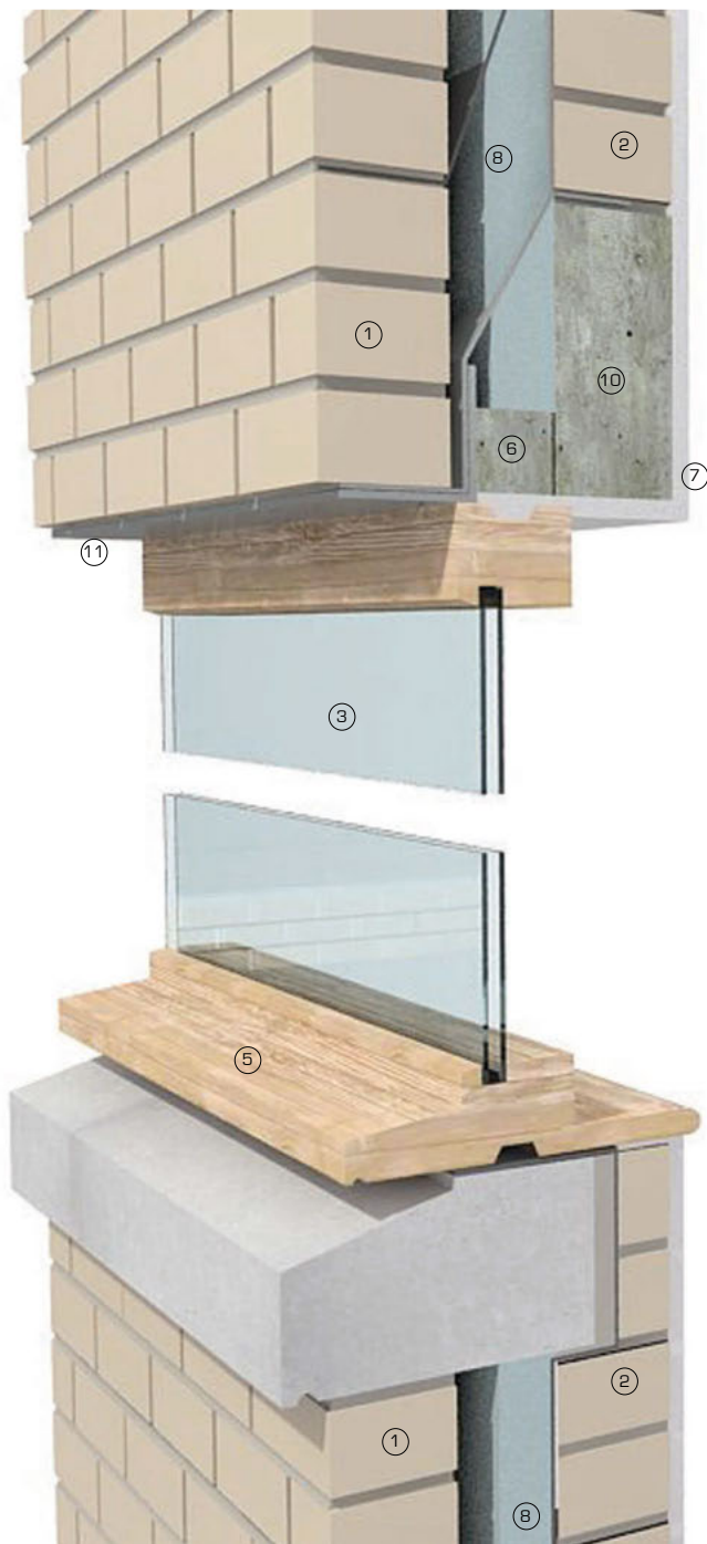
3D view showing typical timber window connections in brick cavity wall
