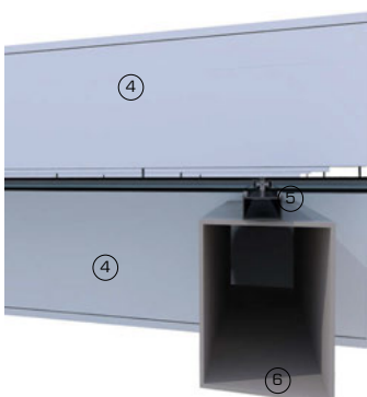
3D exploded views showing toggle-fixed glazed rooflight with GRP-clad structural trusses to form blade-like solar shading louvers and interface with opaque GRP rainscreen roof cladding
