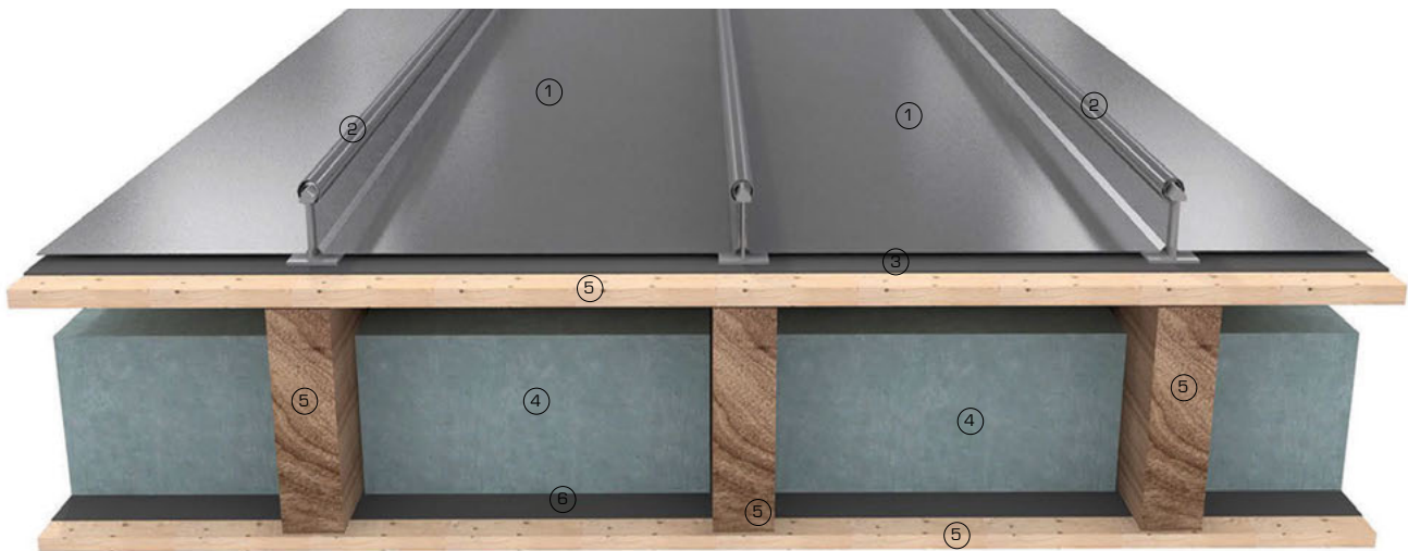
3D sectional view showing section through metal profile roof on timber structure
