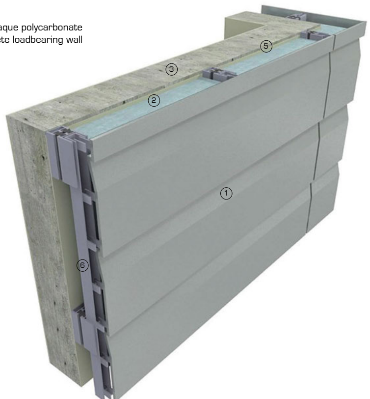
3D detail view showing corner fixing of opaque polycarbonate panels to concrete loadbearing wall
