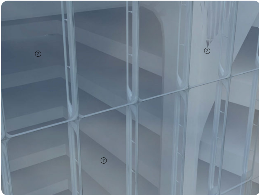
3D views showing cast aluminium glazing frames supporting full-height glazing
