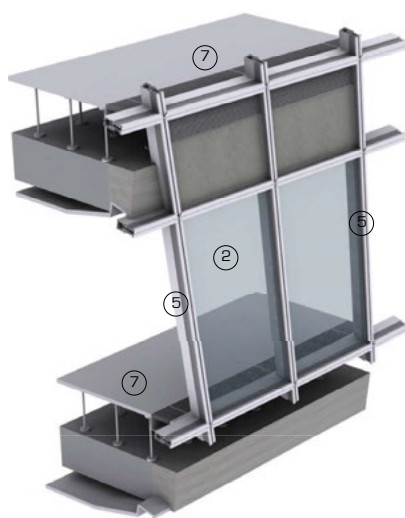
3D views showing unitised double skin glazed facade panel system for twisted facade
