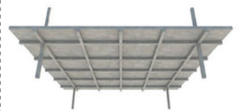
4. Two-way spanning ribbed slab
