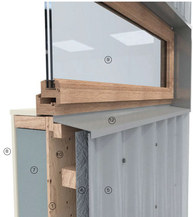
3D detail view showing cutaway through polycarbonate rainscreen
