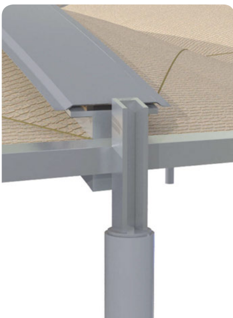
3D detail view showing membrane barrel roof connection to steel support structure
