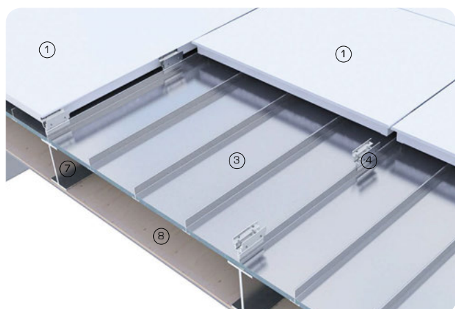
3D detail views showing GRC rainscreen panels fixed to standing seam metal backing and steel primary structure
