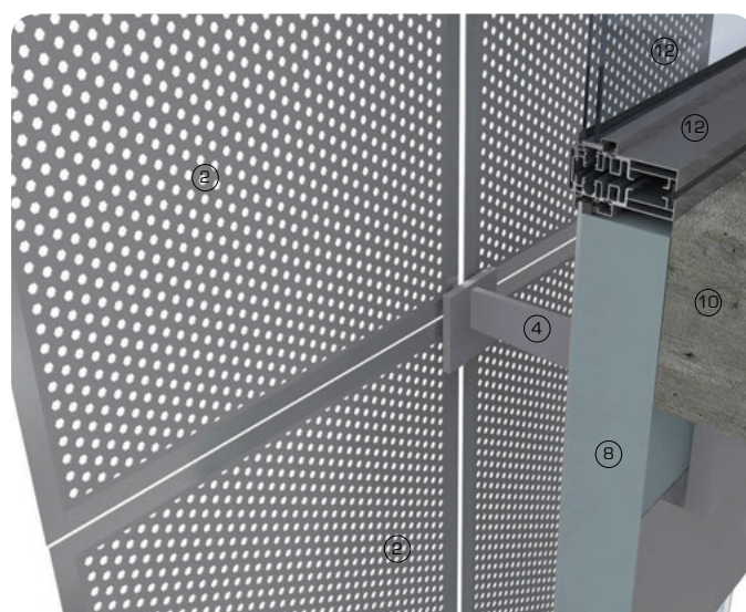
3D detail view showing mesh panel in front of curtain wall glazing
