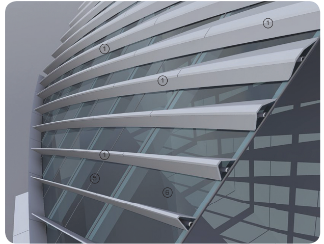
3D overviews showing stick glazed facade supported on steel tube secondary structure with external GRP solar shading louvers
