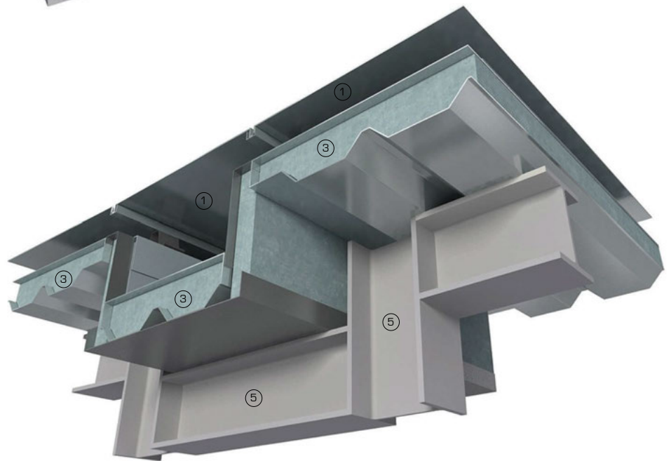
3D detail views showing gutter detail within composite panel arrangement, hidden by rainscreen above
