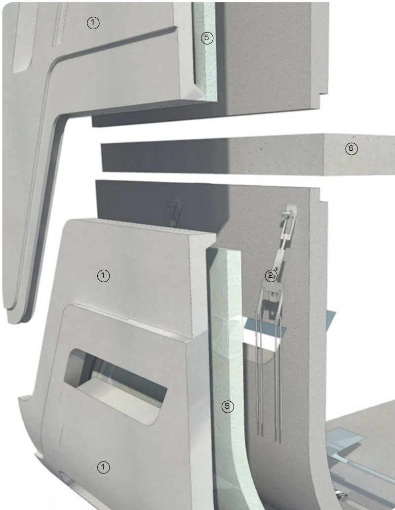
3D exploded, sectional views showing fixing system for large precast concrete cladding panels with structural reinforced concrete wall behind
