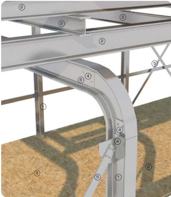
3D detail view showing steel connection plate detail
