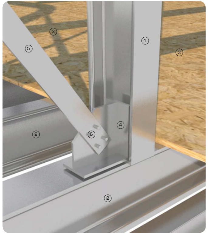
3D detail view showing steel connection plate detail
