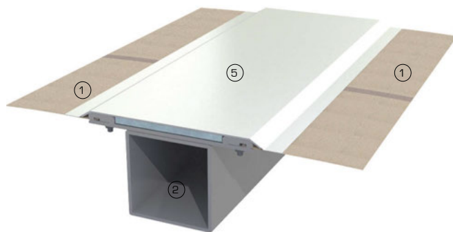
3-D detail of junction between 2 fabric panels
