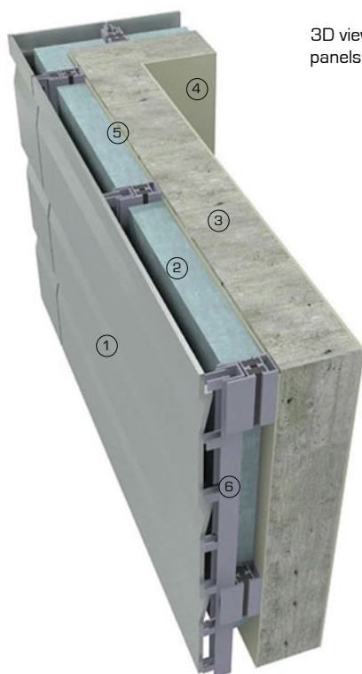
3D detail view showing vertical rail fixing opaque polycarbonate panels to concrete loadbearing wall
