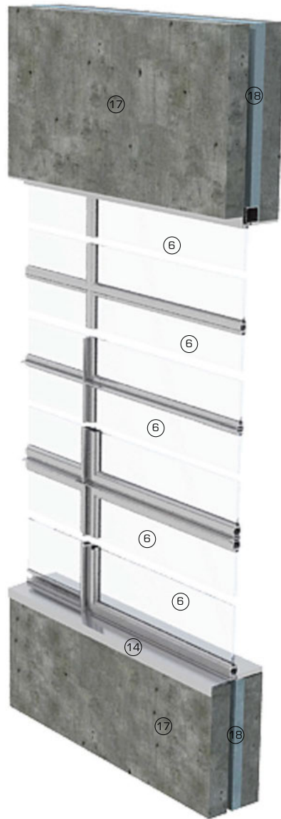
3D view showing rolled steel window embedded within masonry wall construction
