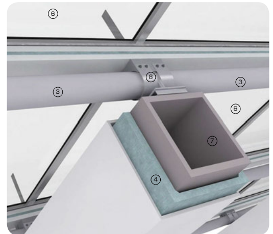
3D detail view showing stick glazed facade supported on steel tube secondary structure with external GRP solar shading louvres
