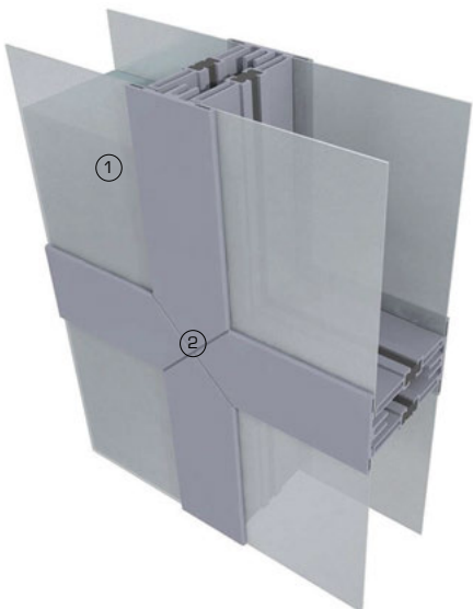
3D detail view showing polycarbonate composite panel construction
