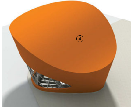
Diagram 4 Joints between panels are filled and coated to form a smooth surface
