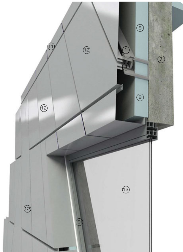
3D view showing basic rainscreen panel system at window opening
