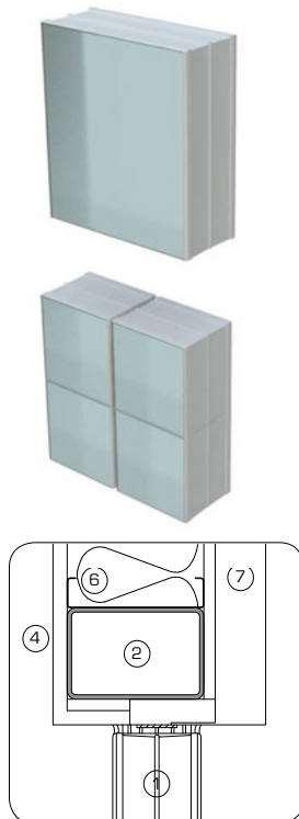
Horizontal section 1:10. Glass blocks supported by box sections
