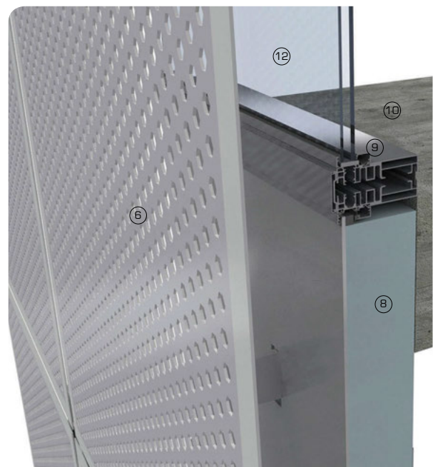
3D detail view showing mesh panel in front of curtain wall glazing
