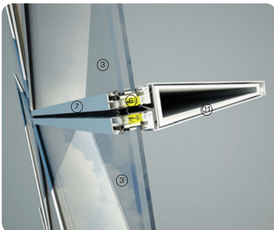
3D sectional detail views showing triangular unitised glazing panels for twisted facade
