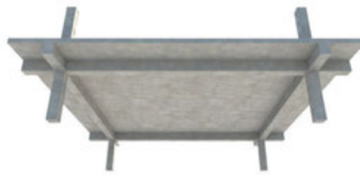
2. Slab with downstand beams
