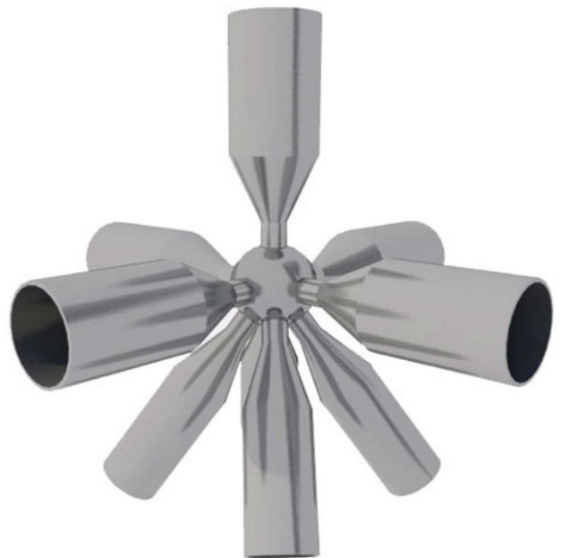
3D views showing typical nodes and chords of a space frame structure
