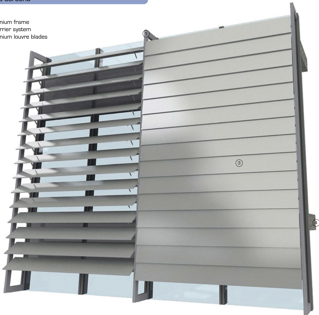
3D view showing metal louvre screen in front of curtain wall system
