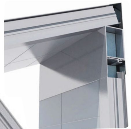
3D view showing typical monopitch GRP rooflight
