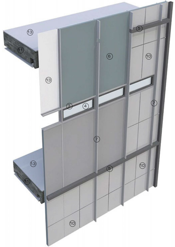
3D cutaway view showing build-up of aluminium glazing system
