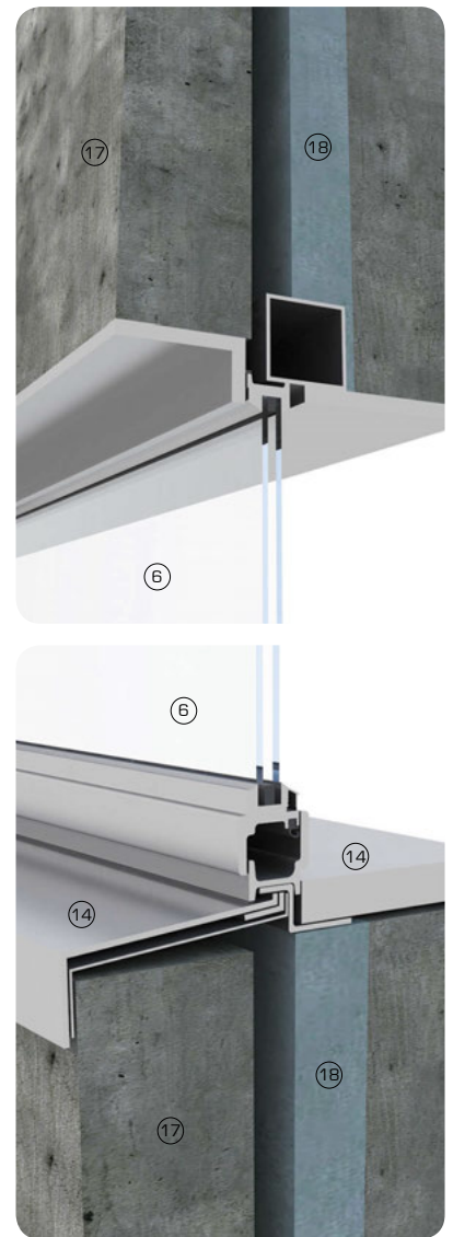
3D detail views showing rolled steel window embedded within masonry wall construction at head and cill conditions
