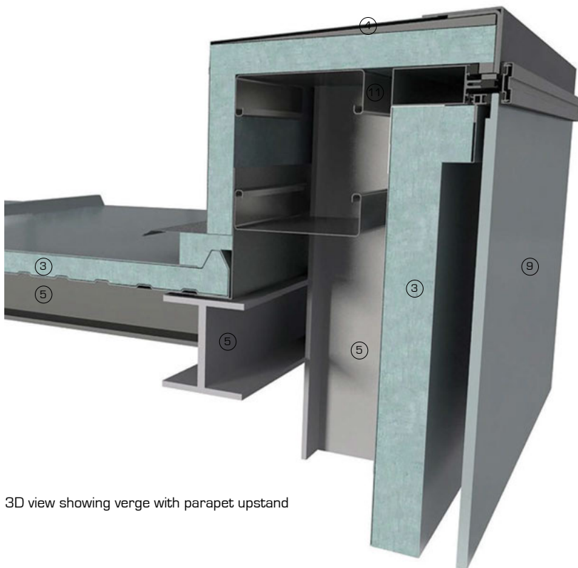
3D detail views showing composite metal panel build-up
