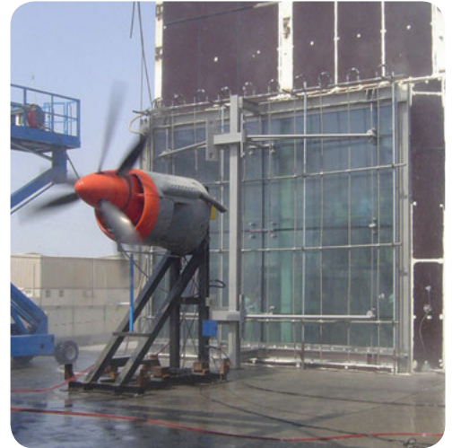
A bolt fixed glazing system has high expected deflections when compared to a framed system.
