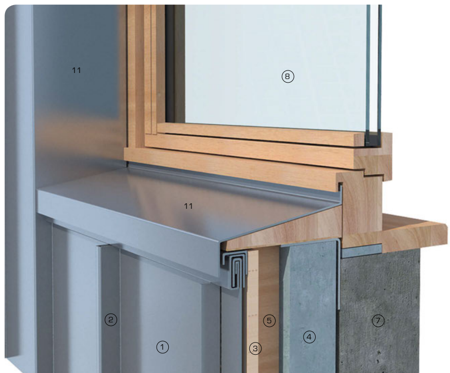
3D detail view showing window cill detail within profiled metal sheet system
