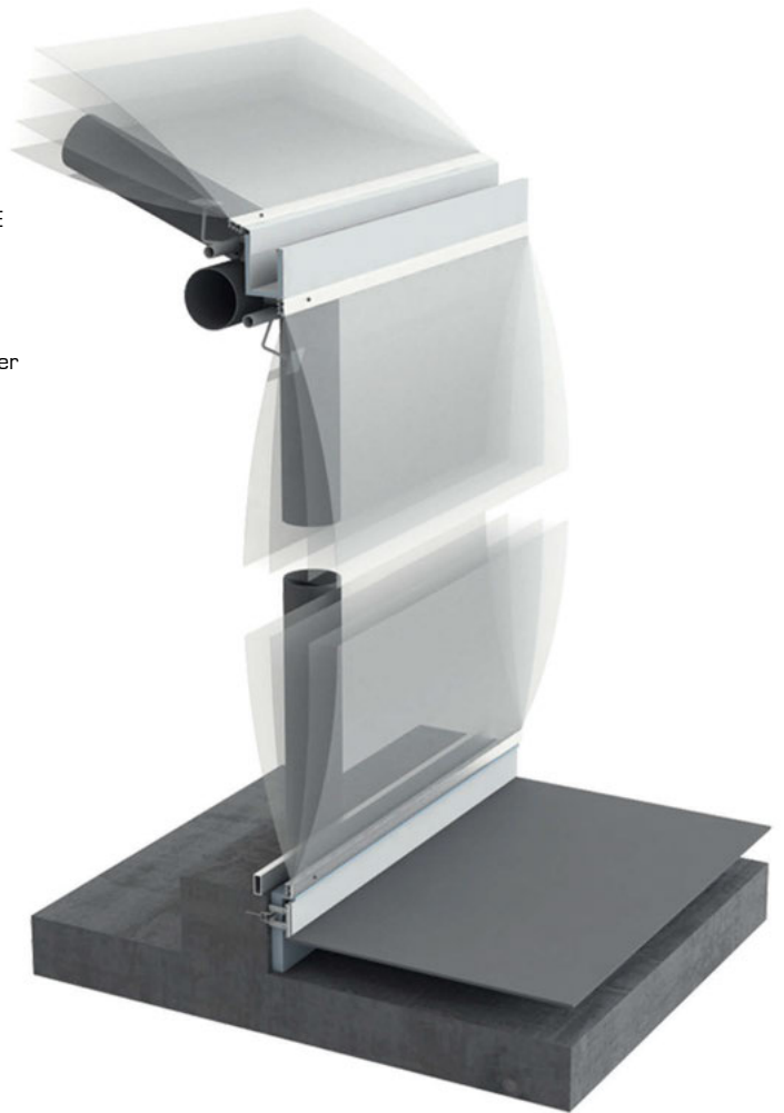
3D sectional views showing ETFE roof and wall panel construction with steel tube support structure
