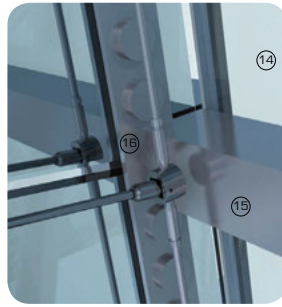
3D detail views showing glass fin-supported glazing system in various configurations
