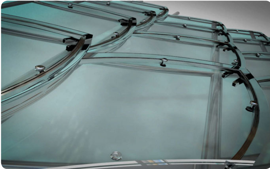
(Right) Working digital model of shingled glazing system supported on steel tubes
