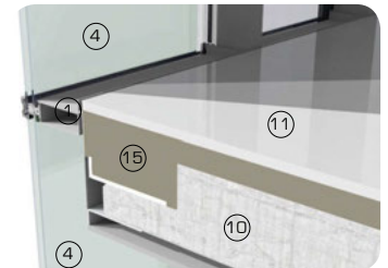
3D detail view showing unitised glazing connection to slab
