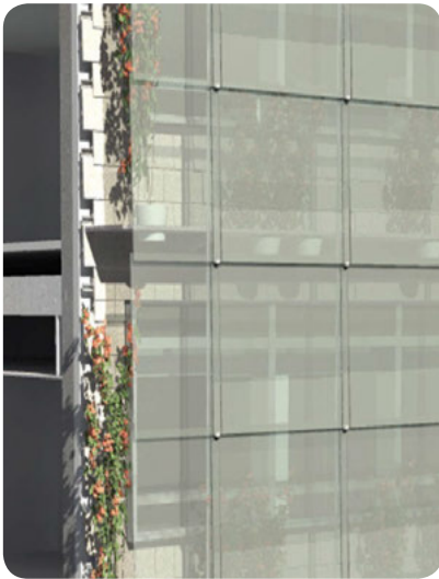
Vertical section 1:20 and 3D views through double skinned facade with plant in cavity
