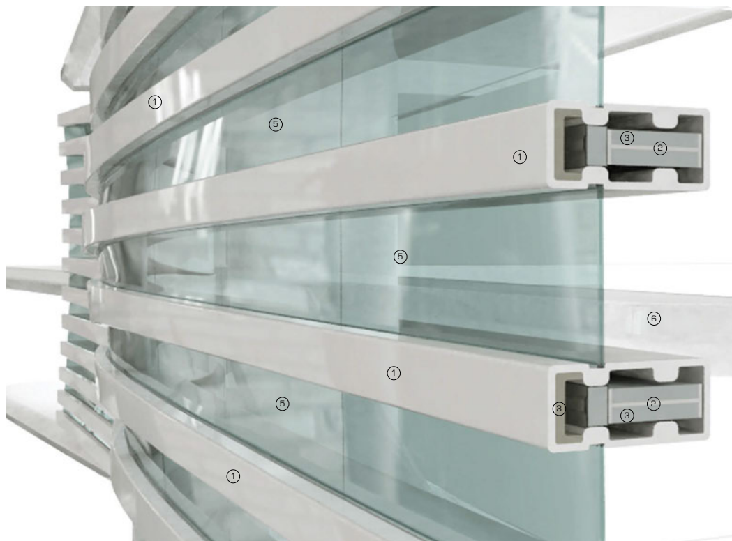
3D sectional detail view showing full-height glazed facade with external GRP cladding over primary steel structure
