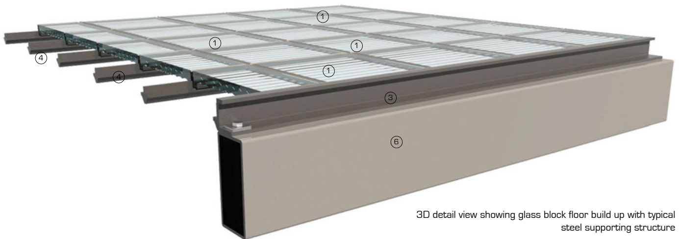
3D overview showing underside of glass block floor build up with typical steel supporting structure
