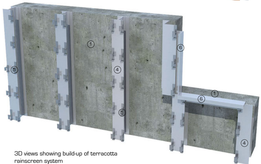
3D detail view showing terracotta rainscreen system at window opening
