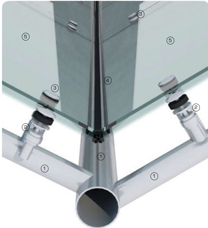
3D view showing bolt fixed glazing with internal fold
