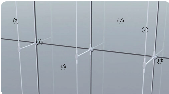
3D detail views showing clamped glazing system fixing method supported on cables
