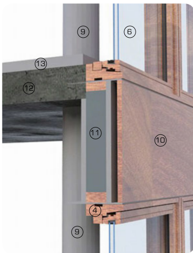
3D detail view showing spandrel panel in timber door and window wall system
