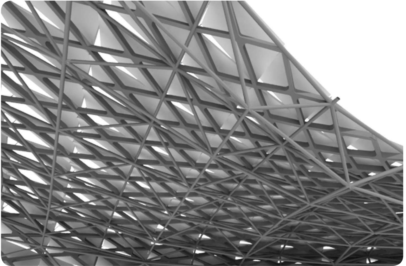
3D views showing GRC rainscreen roof panels in various geometric configurations supported on steel space frame roof truss structure
