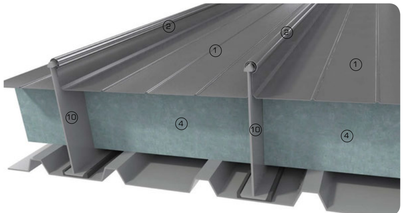
(Below) 3D sectional view showing metal standing seam roof construction
