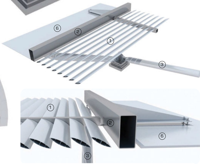
3D views through louvred metal canopy edge and support
