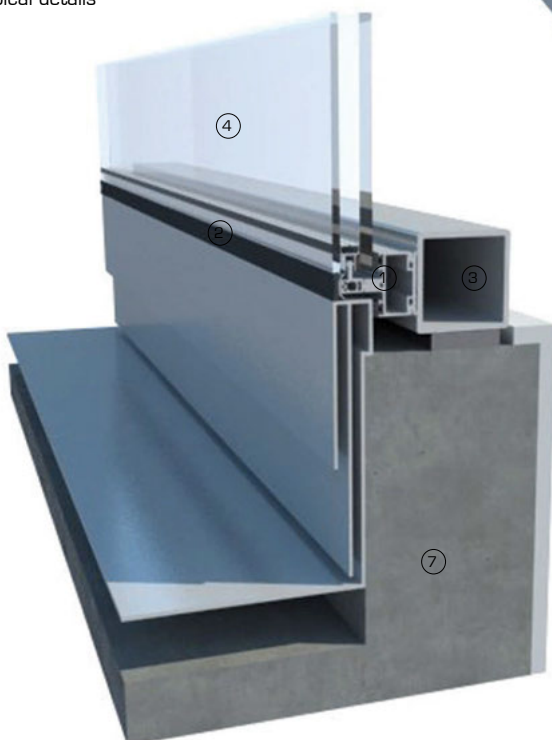
3D view of connection to concrete base
