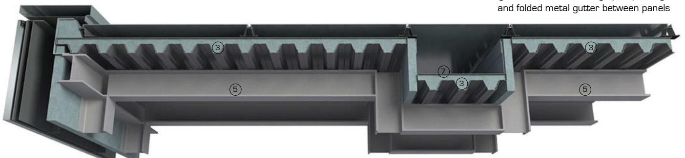
3D view showing vertical section through parapet edge and folded metal gutter between panels
