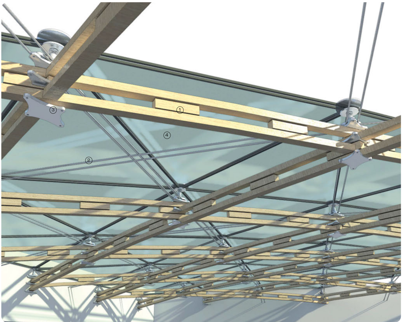
3D views showing timber shell structure with tension cable support and double glazed roof
