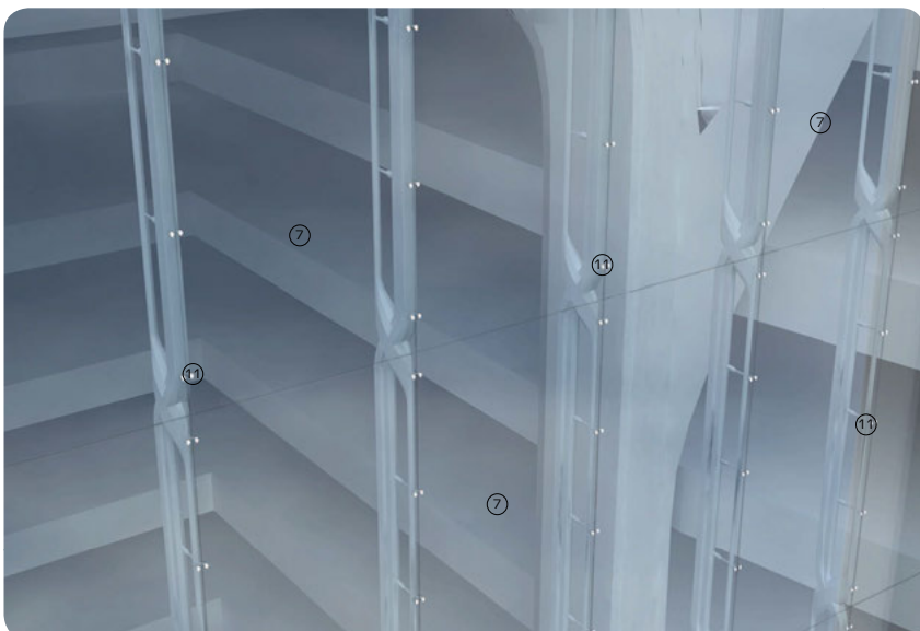
3D view showing cast aluminium glazing frames supporting full-height clamped glazing
