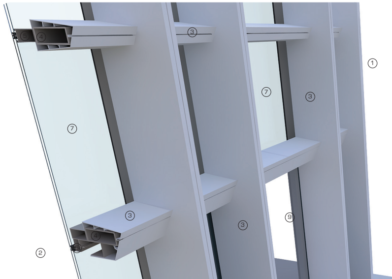
3D sectional view showing GRP-clad steel support structure with full-height toggle-fixed glazing
