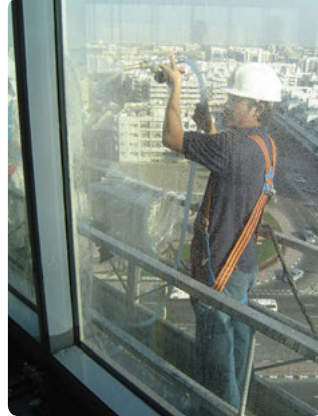
A site-based hose test to check the performance of the tested system when installed in a building.
