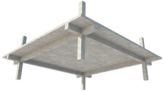
2. Slab with downstand beams
