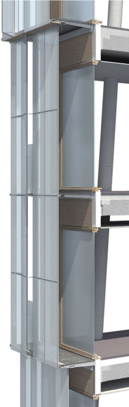
View of vertical section through stepped twin wall facade system
