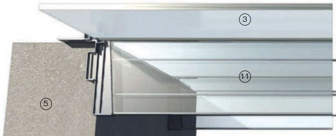
3D detail of connection between glass beam and concrete wall
