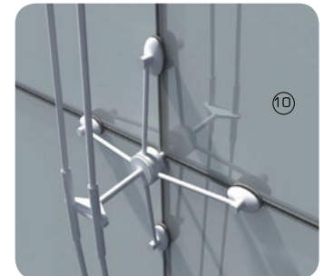
3D detail view showing clamped glazing fixing method
