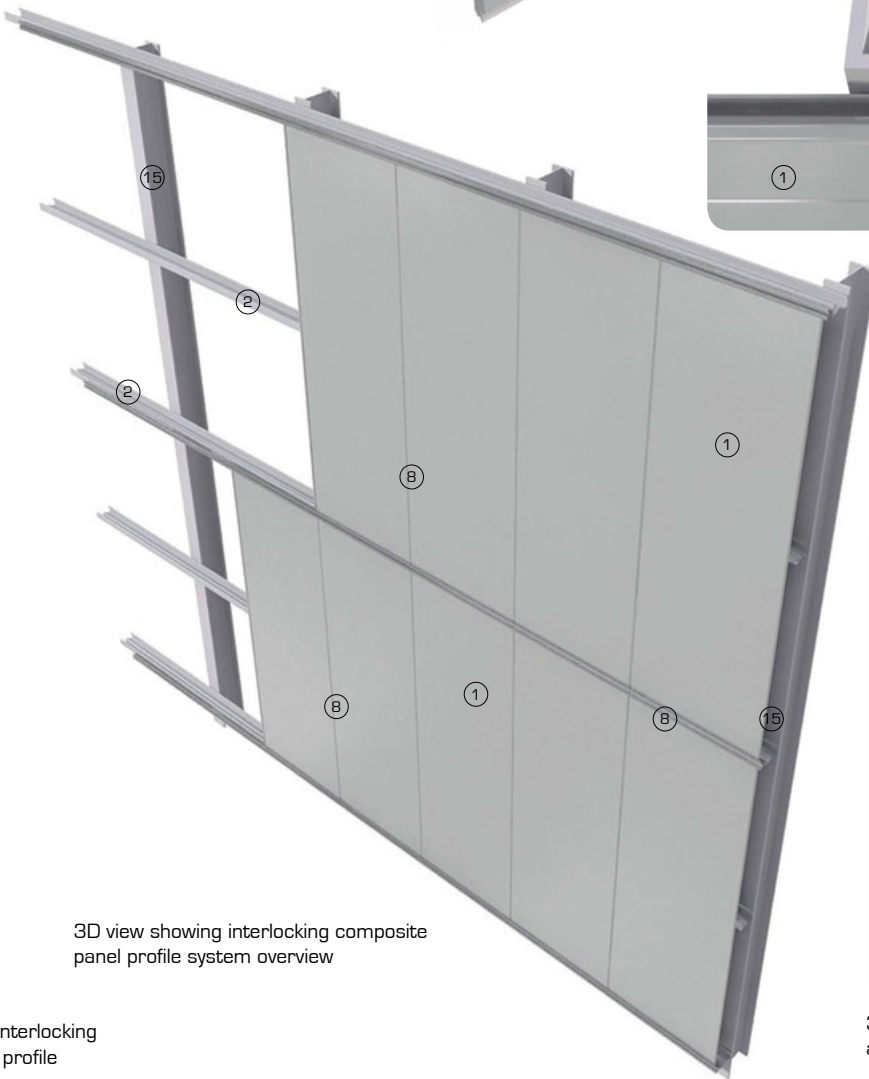
3D detail view showing metal bracket and capping supporting panels
