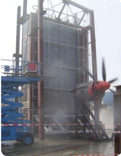
An aero engine generating strong air movement is set in front of a rack of water spray nozzles that simulate wind and rain at different pressures.
