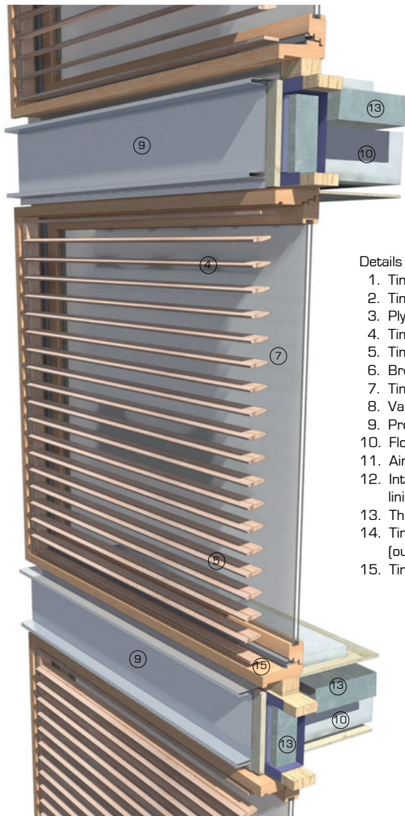
3D view showing timber cladding panel consisting of fixed glazing and louvre screen
