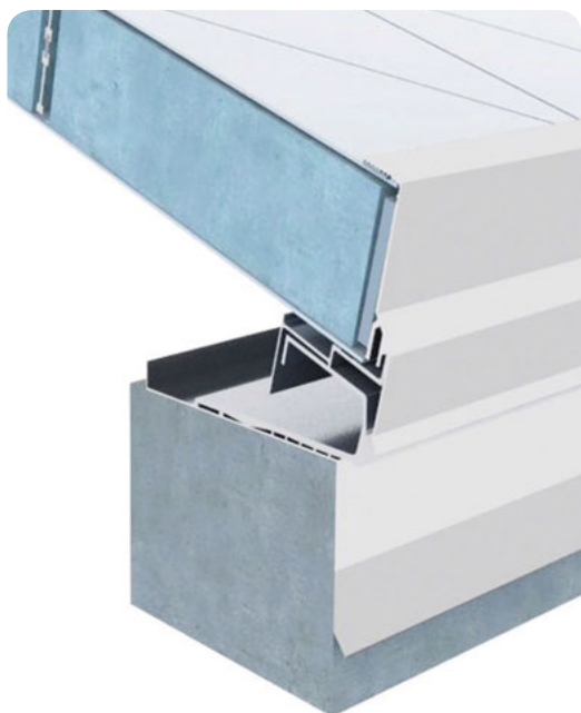
3D detail of junction with external wall
