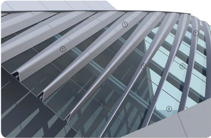
3D overviews showing stick glazed facade supported on steel tube secondary structure with external GRP solar shading louvers
