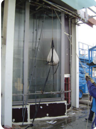
An impact resistance test on a glazed panel.
