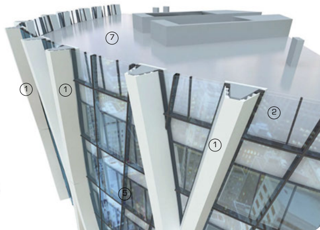
(Left) 3D view showing unitised double skin glazed facade panel system for twisted facade
