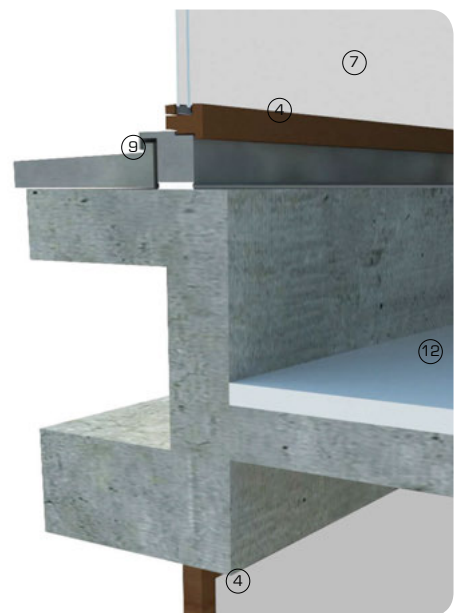
3D view showing roof parapet and window details within cast in-situ concrete wall system
