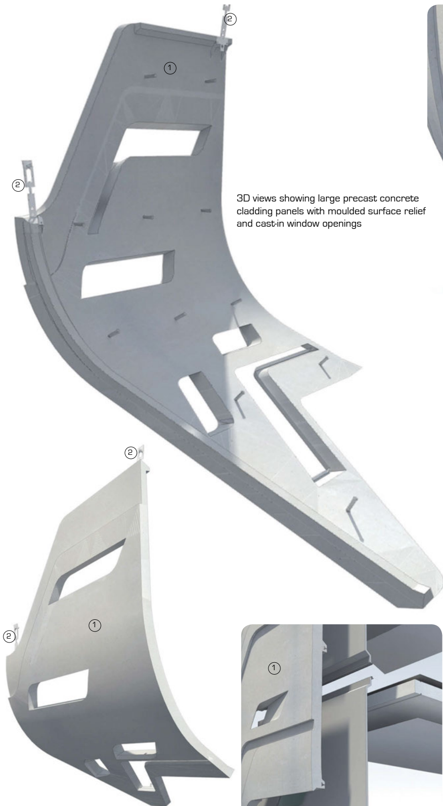
3D sectional views showing fixing system for large precast concrete cladding panels with structural reinforced concrete wall behind
