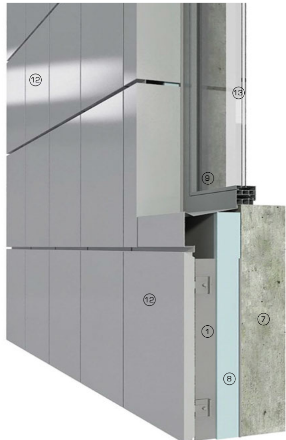
3D detail views showing window and parapet detail in rainscreen wall system
