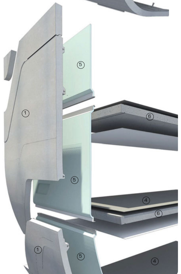
3D exploded, sectional views showing fixing system for large precast concrete cladding panels with structural reinforced concrete wall behind
