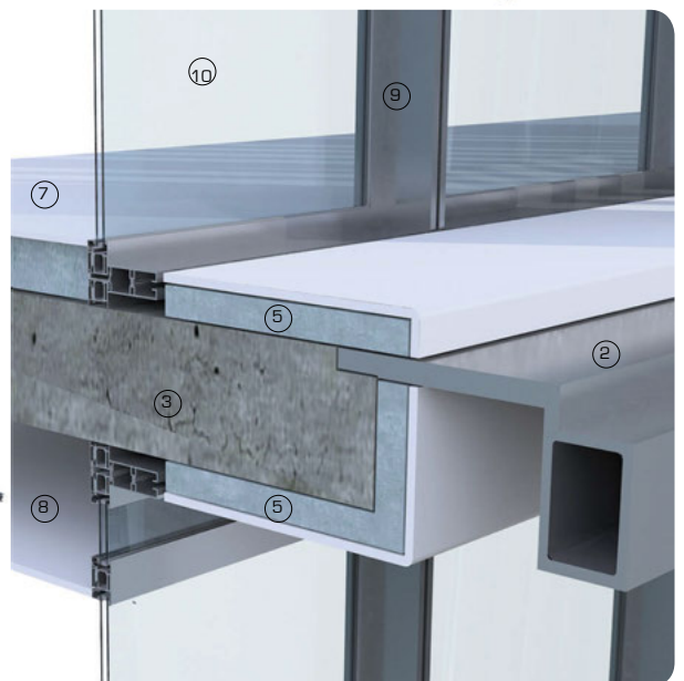
3D detail sectional view showing glazed facade with moving external vertical solar shading louvres
