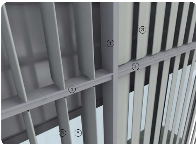
3D detail views showing profiled aluminium louvres and fixing system
