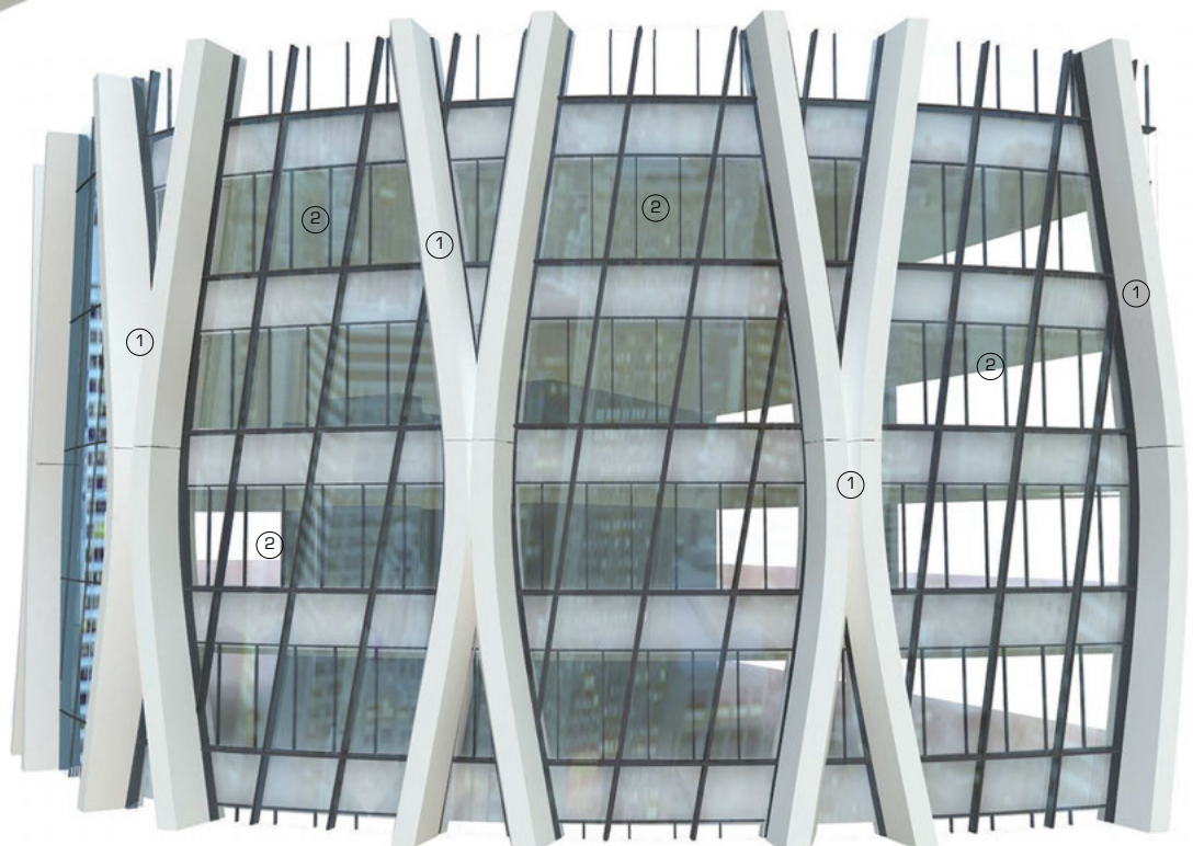
3D detail views showing unitised double skin glazed facade system for twisted facade
