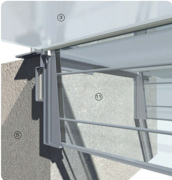
3D detail of connection between glass beam and concrete wall
