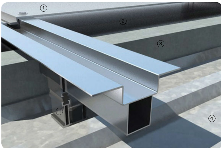
3D view of metal rainscreen roof fixing channel
