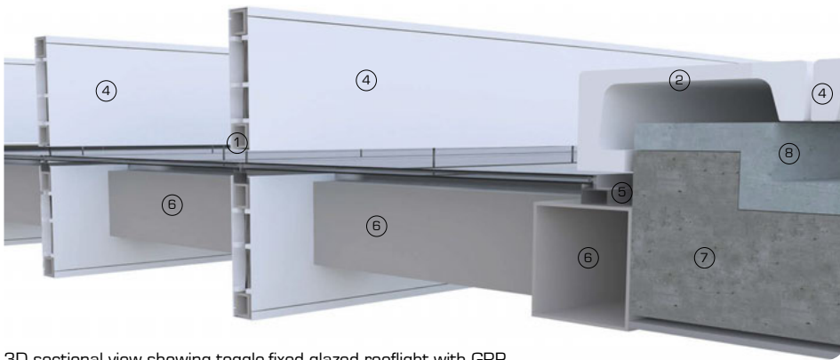
3D sectional views showing underside of toggle-fixed glazed rooflight with GRP-clad structural trusses to form blade-like solar shading louvers
