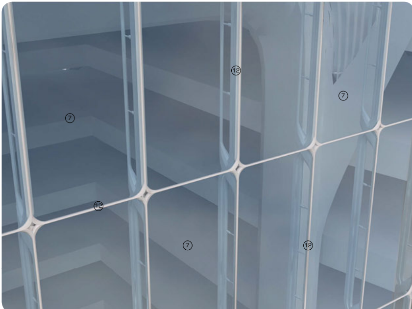
3D views showing cast aluminium glazing frames supporting full-height glazing with cap piece
