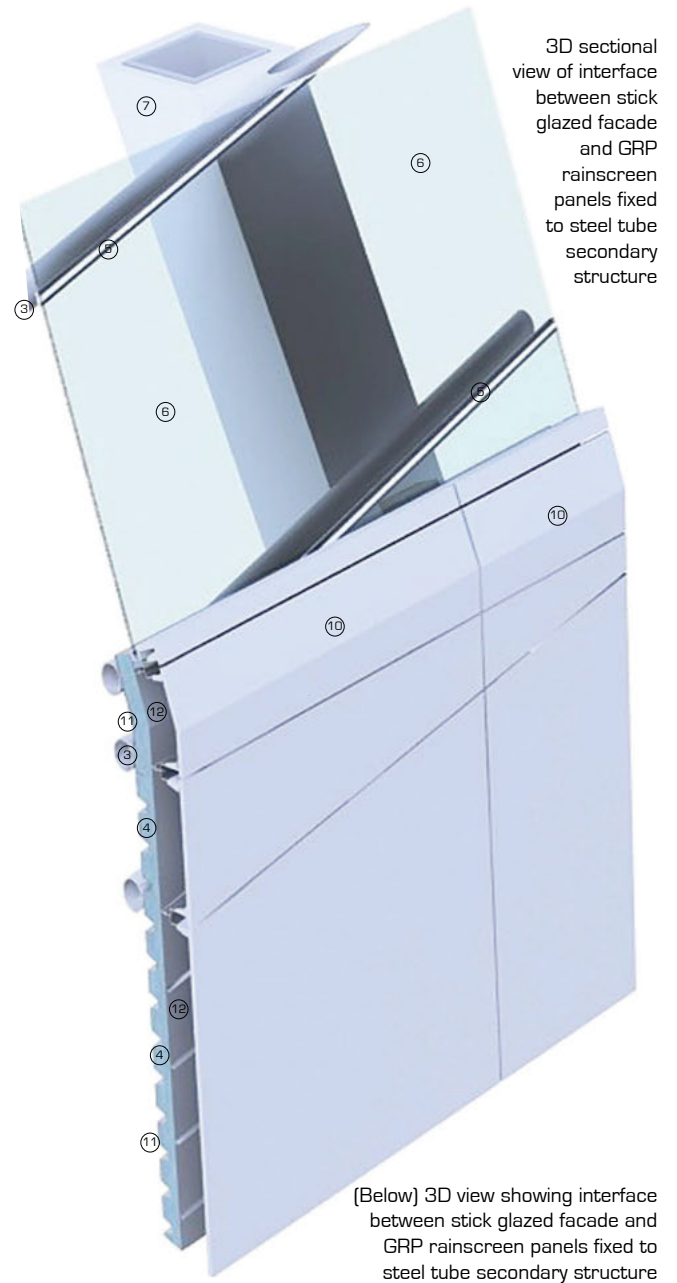
Vertical section. Interface between stick glazed facade and GRP rainscreen panels fixed to steel tube secondary structure
