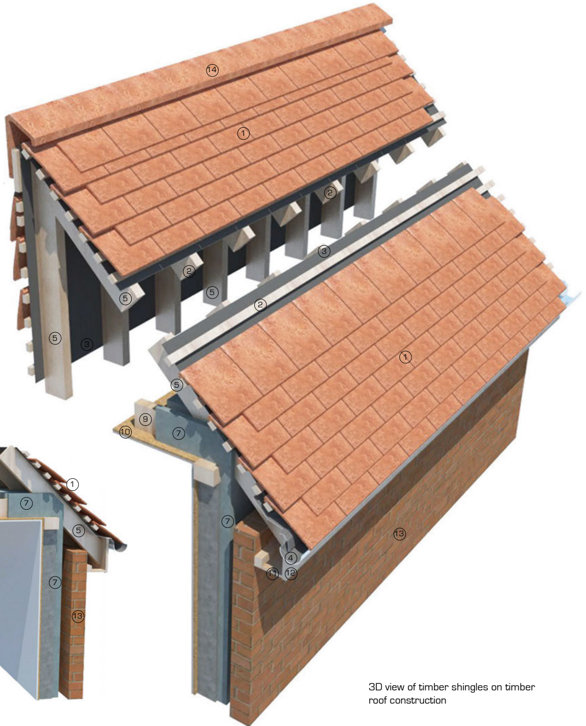
3D view of timber shingles on timber roof construction
