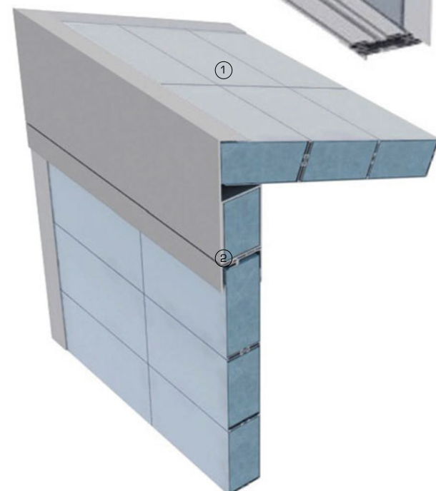
3D view showing typical monopitch GRP rooflight ridge detail
