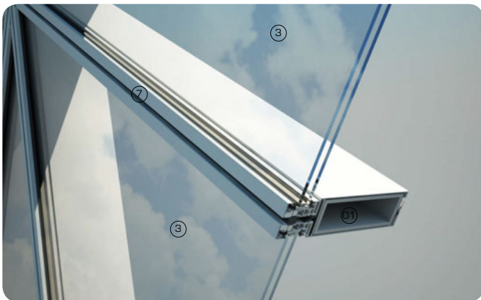
Working digital models of triangular unitised glazing panels for twisted facade
