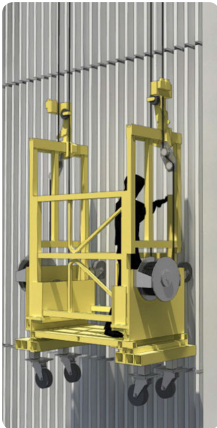
3-D views of typical cleaning cradle on facade
