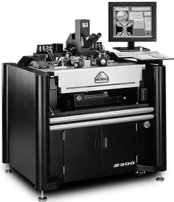
(b) Probe-station (courtesy of Cascade Microtech Inc.)
