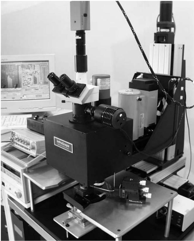
Fig. 5.6. A photograph of an IR microscopy system. A test-fixture is mounted on the thermal chuck beneath the IR microscope. Software on the controlling computer is used to calibrate and capture, compute, and display the temperature [18]. © 2001 SPIE. Reprinted with permission.
