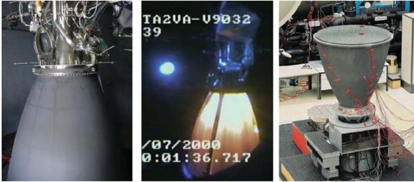
**Figure 7.16** Ceramic nozzle on test bench (left), during the vacuum hot-firing test (middle) and during vibration test (right).
