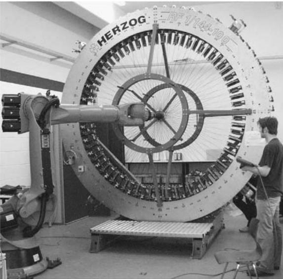
Figure 2.14 Radial overbraiding machine with robot support.
