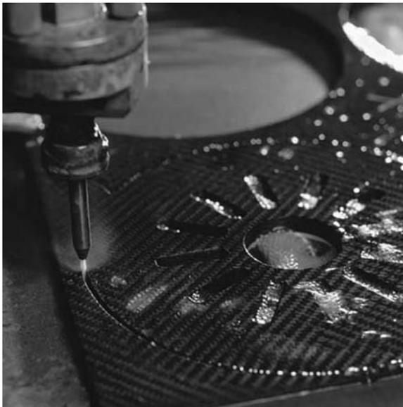
**Figure 16.23** Water jet cutting of the clutch disks at about 3000 bar.
