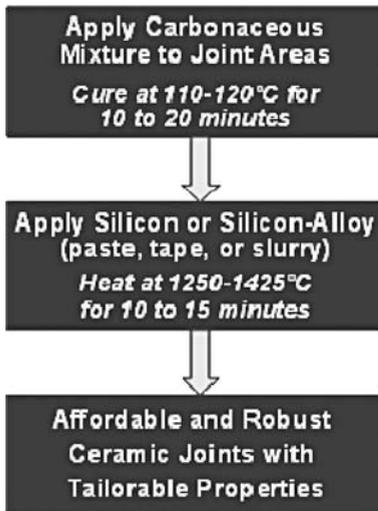
**Figure 13.5** Flow diagram of ARCJoinT ceramic joining technology developed at NASA GRC [4].
