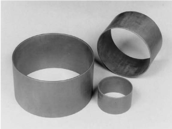
**Figure 6.18** SiC/SiC shaft sleeves for water lubricated journal bearings of large pumps. The outer diameter of these sleeves lies between 100 and 305 mm.
