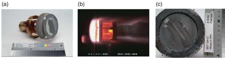
**Figure 13.9** (a) GRABER repaired RCC specimen in ARCjet test holder; (b) photograph during testing; (c) post test photograph [34, 35].
