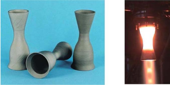
**Figure 7.17** PIP-C/SiC combustion chamber (left) and during hot test (right).
