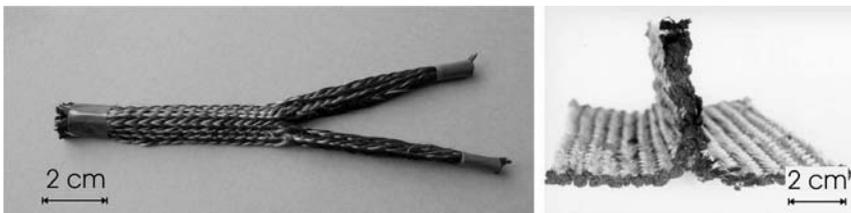
**Figure 2.18** Examples for three-dimensional rotary braided structures.
