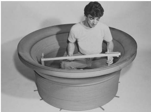
**Figure 14.10** The carbon-carbon nozzle throat of Ariane 5 Solid Rocket Booster [9].
