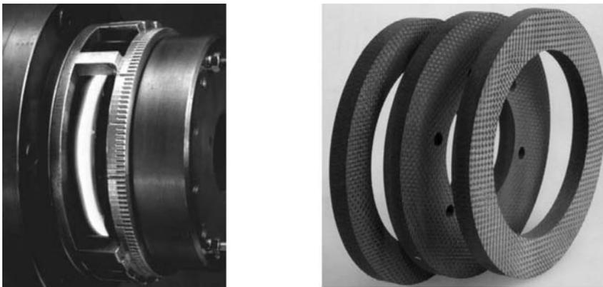
Figure 16.6 Emergency brake system during high energy stop braking (left) and a set of one rotating brake disk and two stationary disks, each made of 2D reinforced C/SiC with an outer diameter of 110mm and a thickness of about 8mm (Mayr Antriebstechnik, Germany).
