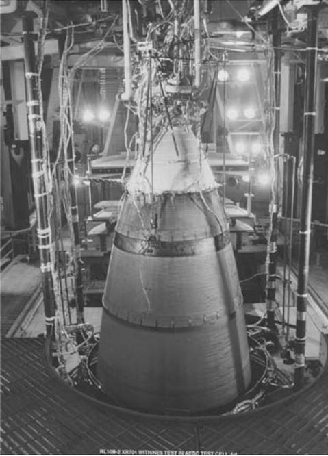
Figure 14.13 Extendible nozzle in production [9].
