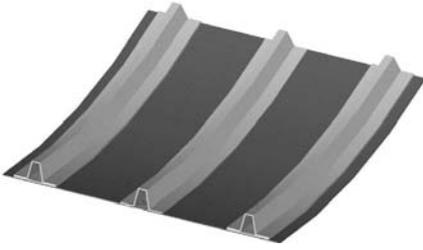
**Figure 2.20** Rib stiffened panel.
