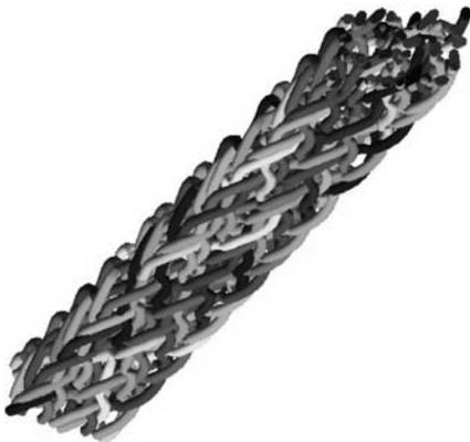
Figure 2.15 Model of a three-dimensional braided structure [31].
