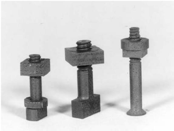
**Figure 6.13** C/SiC screws and nuts, which can be used due to their damage tolerance and notch insensitivity.
