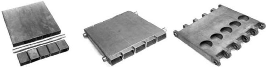
**Figure 5.6** Lightweight C/C-SiC intake ramp demonstrator, manufactured via near-net-shape and *in-situ* joining technique. Left: CFRP single elements manufactured via RTM. Middle: Assembled C/C preform (5 cell body structure, 10 end caps, 2 tubes). Right: Joint C/C-SiC structure after siliconization and final machining (275 mm × 265 mm × 35 mm).
