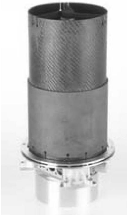
**Figure 5.14** *In-situ* joined C/C-SiC telescope tube ( $\varnothing$  140 mm,  $l$  = 160 mm, wall thickness = 3 mm) for the LCT in the satellite TerraSAR-X (Zeiss Optroniks).
