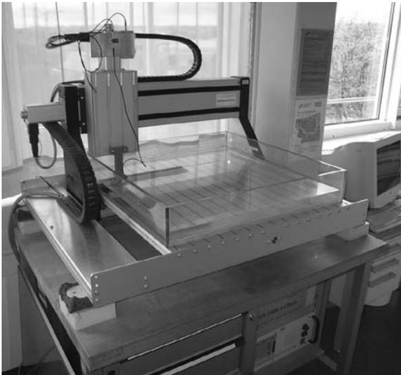
**Figure 11.5** Water-coupled ultrasonic analyzer with water coupling basin.
