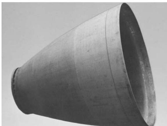
**Figure 14.18** HM7 Sepcarbinox C-SiC exit cone as fabricated and fitted on HM7 (Ariane 4 third stage).
