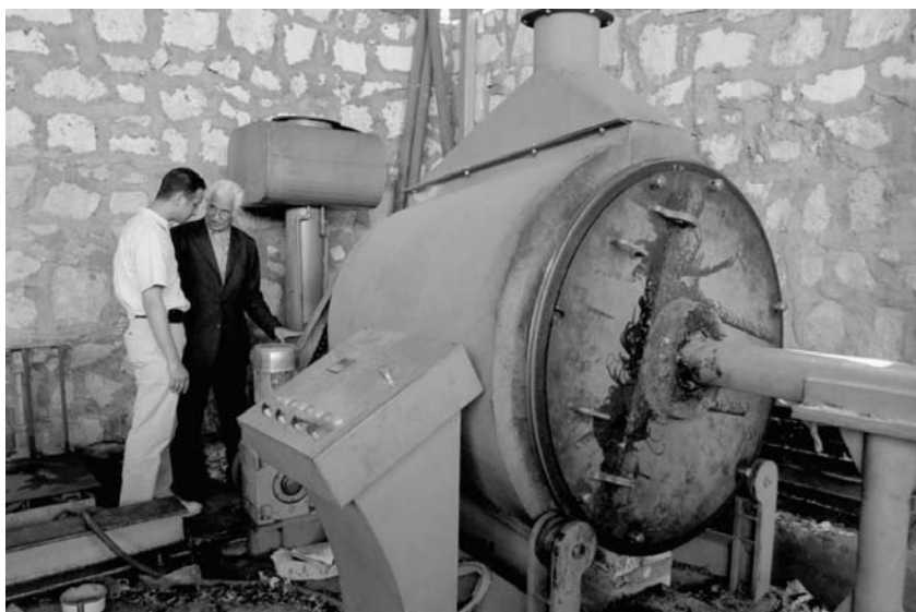
FIGURE 1.13 Horizontal axis mixing and heating furnace.
