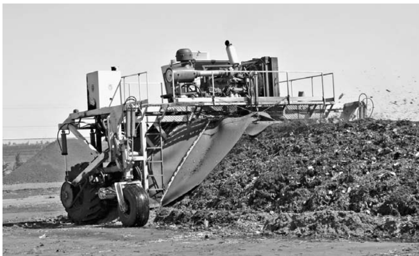
FIGURE 3.21 View of machine used to aerate compost placed in windrows (Courtesy H. Leverenz.)
