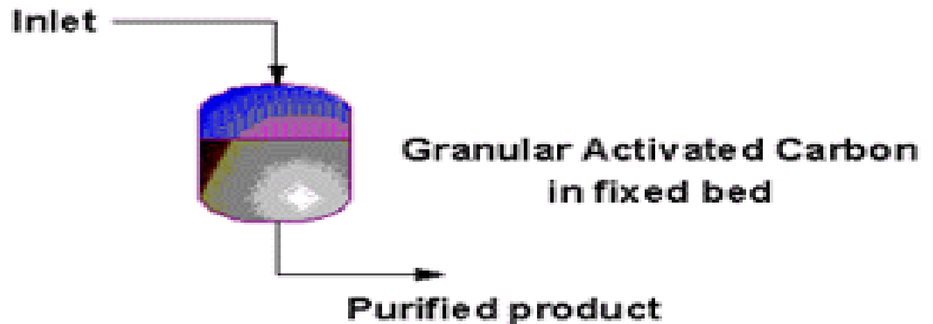
Principle of a granular activated carbon adsorption system
