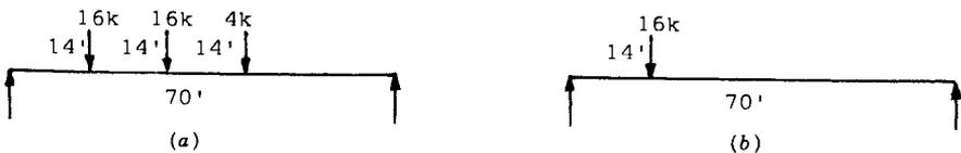
**FIGURE 4-12** Live load arrangement for shear at 14 ft from support: (a) positive; (b) negative.
