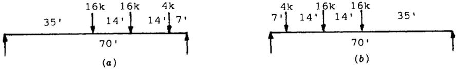
FIGURE 4-13 Live load arrangement for shear at midspan: (a) positive; (b) negative.
