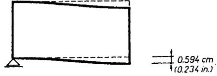
skew. At the ends the bridge is simply supported and has right diaphragms. The intermediate support points are also connected with a skew diaphragm of thickness  $t = 0.3$  m. The concrete structure has a modulus  $E_c = 38,500$  MN/m<sup>2</sup> (5890 ksi), and is loaded symmetrically with two uniformly distributed live loads of 100 kN/m each.
