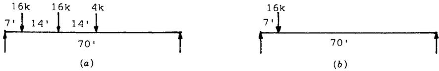
**FIGURE 4-11** Live load arrangement for shear at 7 ft from support: (a) positive; (b) negative.
