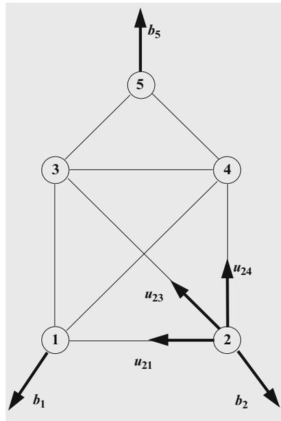
FIGURE 16.1. Sample topology for a two-dimensional structure.
