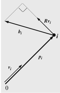
FIGURE 16.2. The  $i$ th summand in (16.6) is the length of  $p_i$  times the length of the projection of  $b_i$  onto the direction given by  $Rv_i$ . This is precisely the torque around an axis at 0 caused by the force  $b_i$  applied at joint  $i$ .
