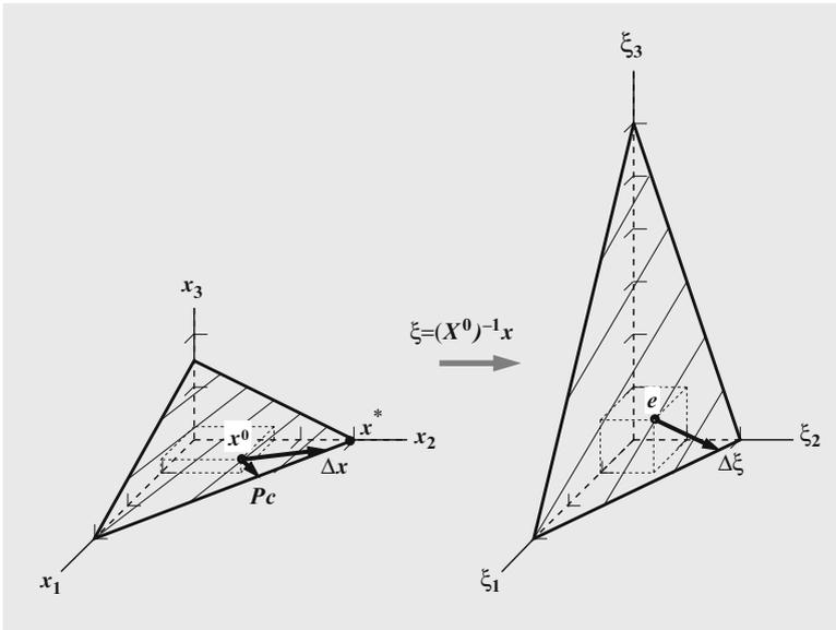
FIGURE 21.2. The effect of affine scaling on projected gradients.
