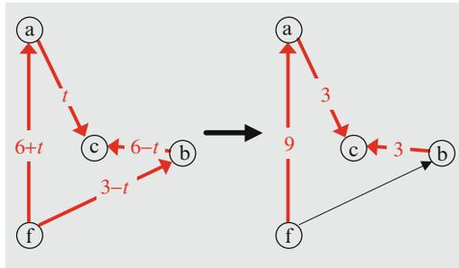
FIGURE 14.7. The cycle produced by including the entering arc with the spanning tree. As the flow  $t$  on the entering arc increases, eventually the flow on arc  $(f,b)$  becomes zero (when  $t = 3$ ). Hence, arc  $(f,b)$  is the leaving arc.
