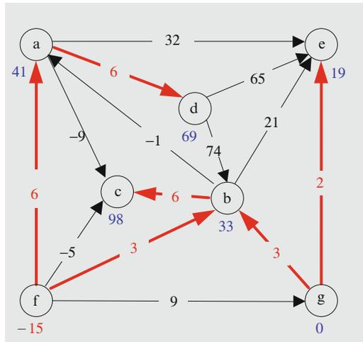
FIGURE 14.6. The *fat arcs* show a spanning tree for the network in Figure 14.1. The numbers shown on the arcs of the spanning tree are the primal flows, the numbers shown next to the nodes are the dual variables, and the numbers shown on the arcs not belonging to the spanning tree are the dual slacks.
