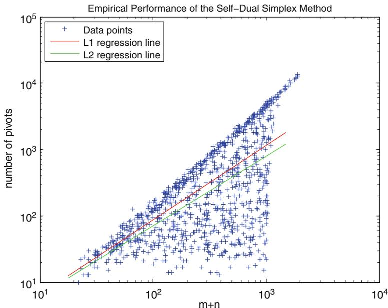
FIGURE 12.4. The parametric self-dual simplex method was used to solve 1,000 problems known to have an optimal solution. Shown here is a log-log plot showing the number of pivots required to reach optimality plotted against  $m + n$ . Also shown are the  $L^1$  and  $L^2$  regression lines.
