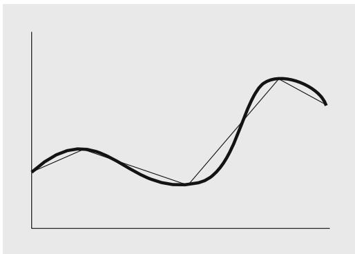
FIGURE 23.3. A nonlinear function and a piecewise linear approximation to it.
