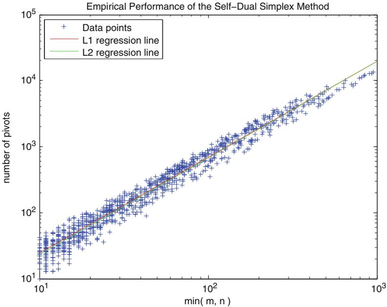
FIGURE 12.5. The parametric self-dual simplex method was used to solve 1,000 problems known to have an optimal solution. Shown here is a log-log plot showing the number of pivots required to reach optimality plotted against  $\min(m, n)$ . In this case, the  $L^1$  and  $L^2$  regression lines are almost exactly on top of each other.
