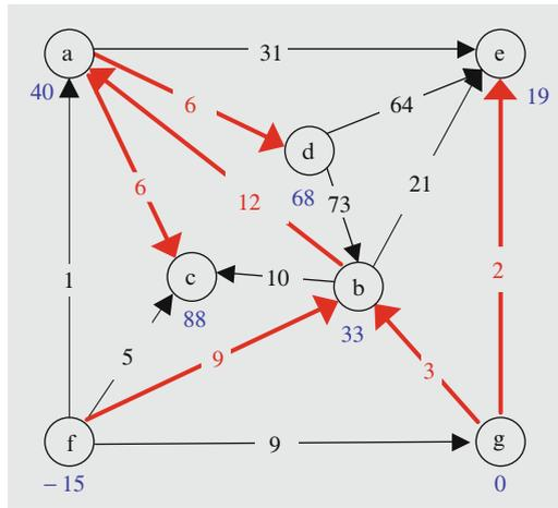
FIGURE 14.12. The tree solution at the end of the third iteration. To get from the spanning tree in Figure 14.11 to here, we let arc  $(f,b)$  enter and arc  $(f,a)$  leave. This tree solution is the *optimal* solution to the problem.
