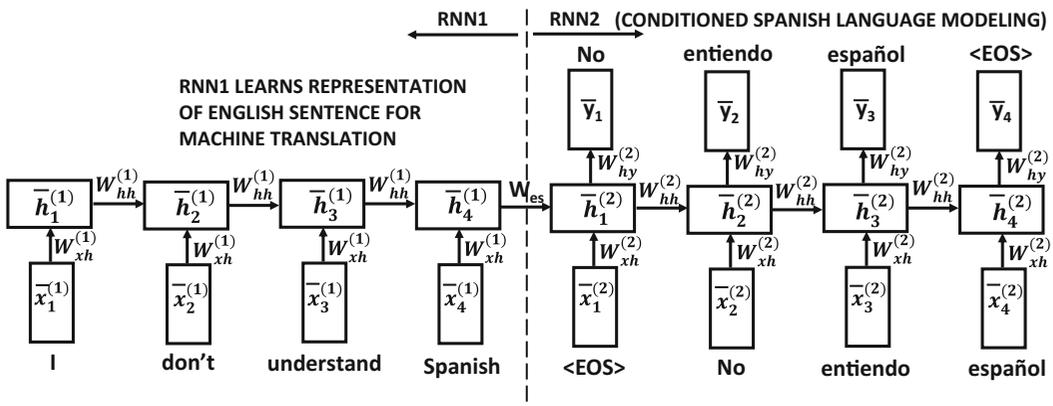
Figure 7.10: Machine translation with recurrent neural networks. Note that there are two separate recurrent networks with their own sets of shared weights. The output of  $\bar{h}_4^{(1)}$  is a fixed length encoding of the 4-word English sentence.
