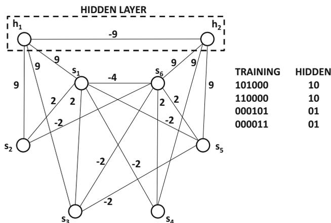
Figure 6.2: The Hopfield network with two hidden nodes
