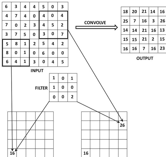
Figure 8.2: An example of a convolution between a  $7 \times 7 \times 1$  input and a  $3 \times 3 \times 1$  filter with stride of 1. A depth of 1 has been chosen for the filter/input for simplicity. For depths larger than 1, the contributions of each input feature map will be added to create a single value in the feature map. A single filter will always create a single feature map irrespective of its depth.
