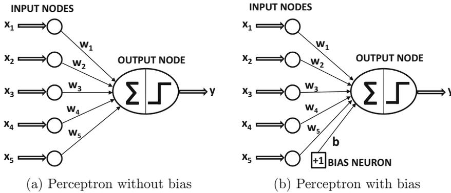
Figure 1.3: The basic architecture of the perceptron
