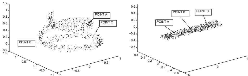
(a) A nonlinear pattern in three dimensions      (b) A reduced data set in two dimensions
