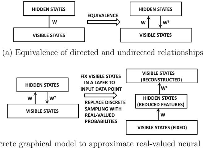
Figure 6.4: Using trained RBM to approximate trained autoencoder
