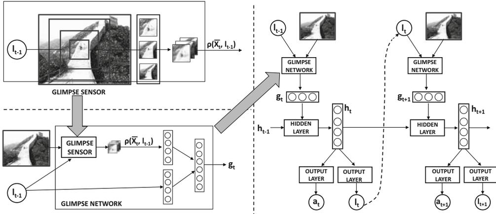
Figure 10.2: The recurrent architecture for leveraging visual attention
