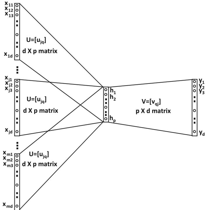
Figure 2.15: Word2vec: The CBOW model. Note the similarities and differences with Figure 2.13, which uses a single set of inputs with a linear output layer. One could also choose to collapse the  $m$  sets of  $d$  input nodes into a single set of  $d$  inputs, and aggregate the  $m$  one-hot encoded inputs in a single context window to achieve the same effect. In such a case, the input is no longer one-hot encoded.
