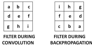
Figure 8.7: The inverse of a kernel for backpropagation
