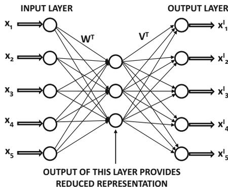
Figure 2.7: A basic autoencoder with a single layer
