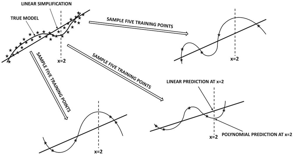
Figure 4.2: **Overfitting with increased model complexity:** The linear model does not change much with the training data, whereas the polynomial model changes drastically. As a result, the inconsistent predictions of the polynomial model at  $x = 2$  are often more inaccurate than those of the linear model. The polynomial model does have the ability to outperform the linear model *if enough training data is provided*.
