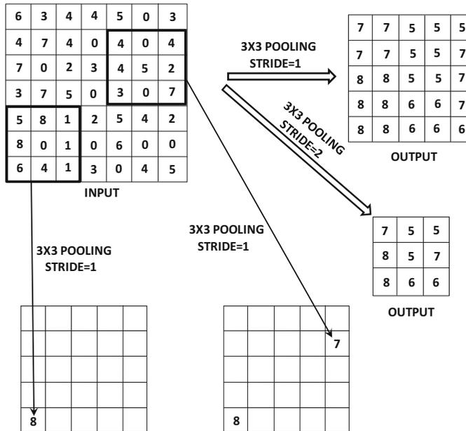
Figure 8.4: An example of a max-pooling of one activation map of size  $7 \times 7$  with strides of 1 and 2. A stride of 1 creates a  $5 \times 5$  activation map with heavily repeating elements because of maximization in overlapping regions. A stride of 2 creates a  $3 \times 3$  activation map with less overlap. Unlike convolution, each activation map is independently processed and therefore the number of output activation maps is exactly equal to the number of input activation maps.
