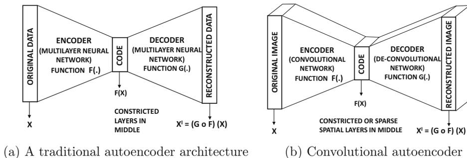
Figure 8.17: A traditional autoencoder and a convolutional autoencoder.
