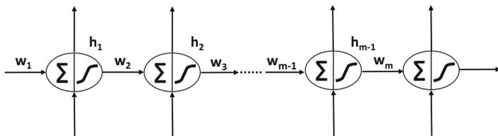
Figure 7.7: The vanishing and exploding gradient problems
