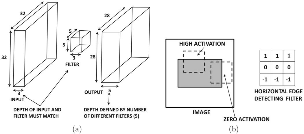
Figure 8.1: (a) The convolution between an input layer of size  $32 \times 32 \times 3$  and a filter of size  $5 \times 5 \times 3$  produces an output layer with spatial dimensions  $28 \times 28$ . The depth of the resulting output depends on the number of distinct filters and not on the dimensions of the input layer or filter. (b) Sliding a filter around the image tries to look for a particular feature in various windows of the image.
