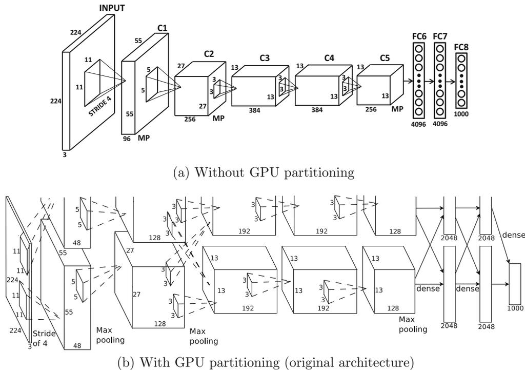
Figure 8.9: The *AlexNet* architecture. The ReLU activations follow each convolution layer, and are not explicitly shown. Note that the max-pooling layers are labeled as MP, and they follow only a subset of the convolution-ReLU combination layers. The architectural diagram in (b) is from [A. Krizhevsky, I. Sutskever, and G. Hinton. Imagenet classification with deep convolutional neural networks. *NIPS Conference*, pp. 1097–1105. 2012.] ©2012 A. Krizhevsky, I. Sutskever, and G. Hinton.
