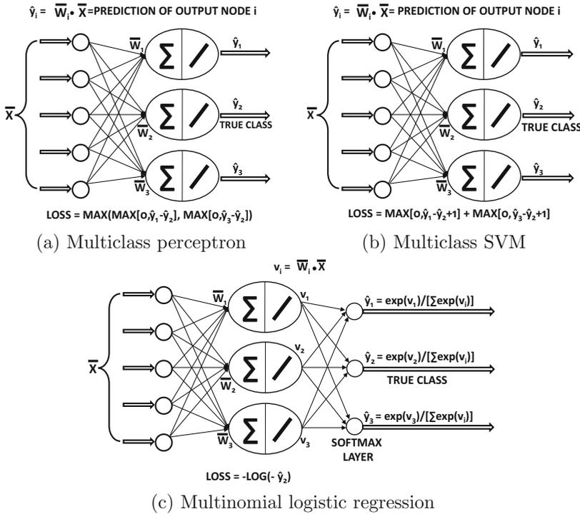
Figure 2.5: Multiclass models: In each case, class 2 is assumed to be the ground-truth class.
