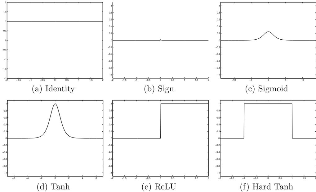
Figure 1.10: The derivatives of various activation functions
