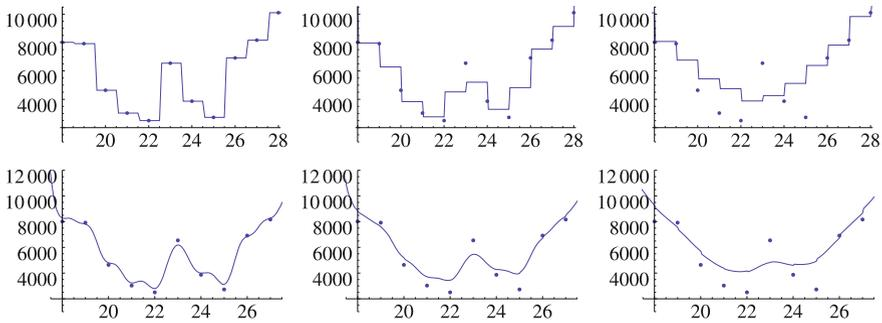
**Fig. 8.19** Comparison of the  $k$ -nearest neighbor method (upper row) with  $k = 1$  (left),  $k = 2$  (middle) and  $k = 6$  (right), to its distance weighted variant (lower row) with  $\alpha = 20$  (left),  $\alpha = 4$  (middle) and  $\alpha = 1$  (right) on a one-dimensional dataset
