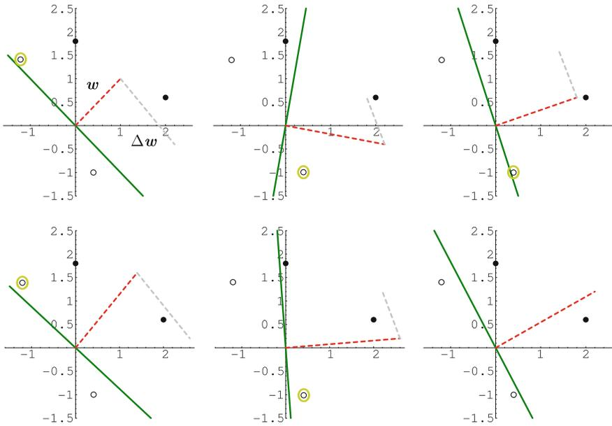
**Fig. 8.10** Application of the perceptron learning rule to two positive (•) and two negative (◦) data points. The *solid line* shows the current dividing line  $w x = 0$ . The *orthogonal dashed line* is the weight vector  $w$  and the *second dashed line* the change vector  $\Delta w = x$  or  $\Delta w = -x$  to be added, which is calculated from the currently active data point surrounded in *light green*
