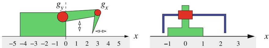
**Fig. 10.2** By moving both of its joints, the crawling robot in the *left* of the image can move forward and backward. The walking robot on the *right side* must correspondingly move the frame *up* and *down* or *left* and *right*. The feedback for the robot’s movement is positive for movement to the *right* and negative for movement to the *left*
