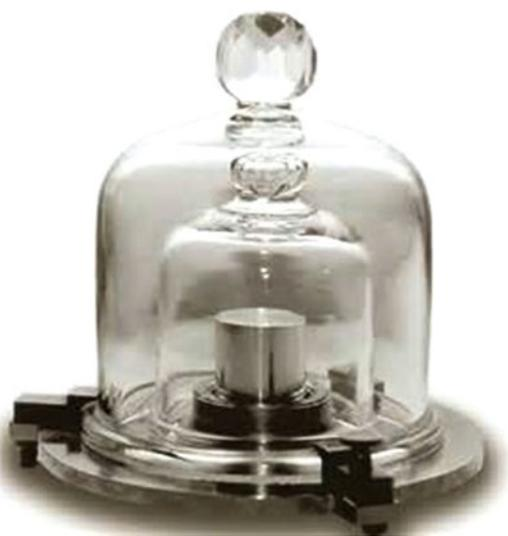
**Figure 1.27** Standard kilogram of platinum-iridium, kept under vacuum in Paris ([https://en.wikipedia.org/wiki/Kilogram#International\\_prototype\\_kilogram](https://en.wikipedia.org/wiki/Kilogram#International_prototype_kilogram))
