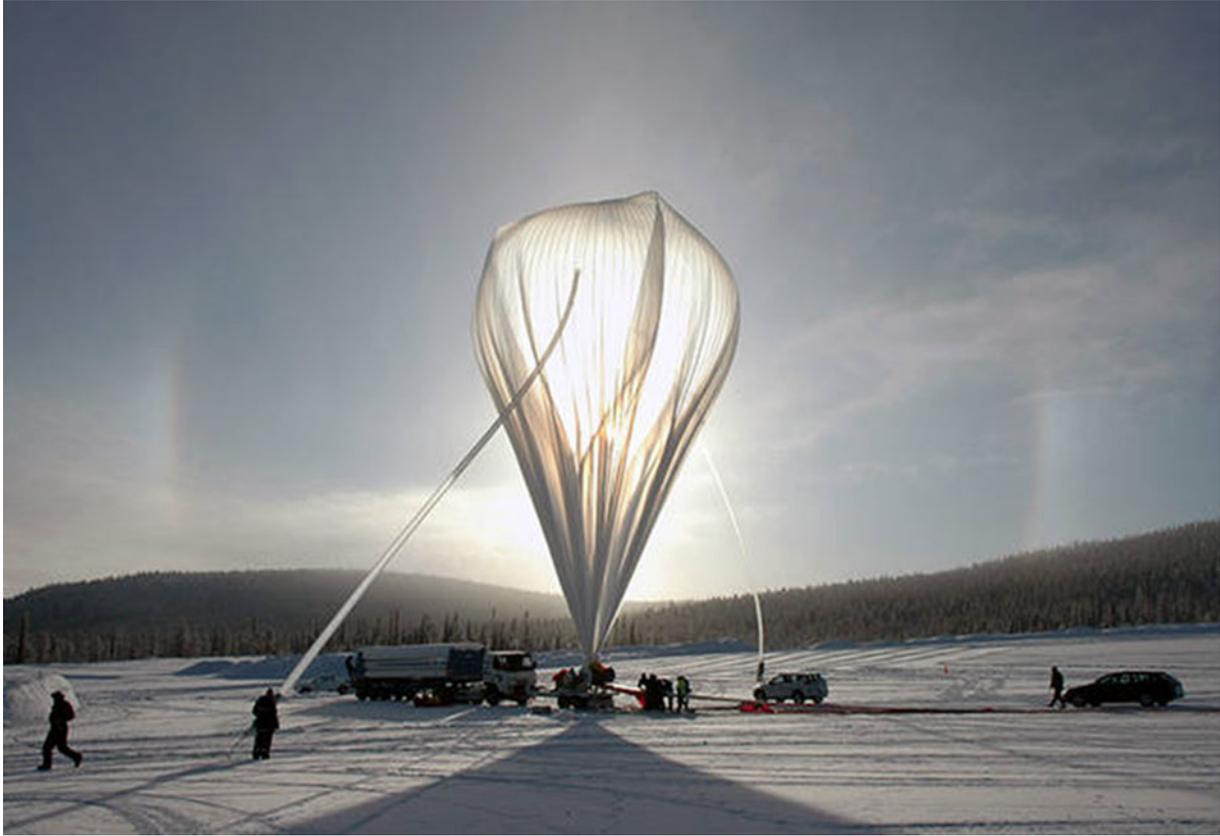
**Figure 7.7** Start of a helium-filled research balloon for the investigation of the higher stratosphere. The balloon is filled only with a low He-pressure. With increasing height the external pressure decreases and the balloon inflates, increasing its volume and the buoyancy (SSC/DLR) (<http://www.eskp.de/turmhohe-forschungsballoons-messen-ozonschicht/>)
