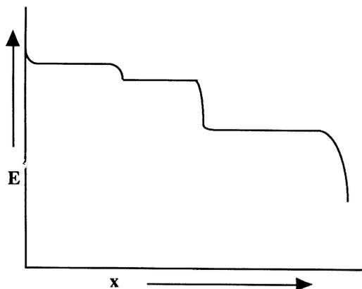
**Fig. 10.6** Schematic equilibrium discharge curve of an electrode that undergoes a series of multiphase reactions in which the residual value of  $F$  is 0
