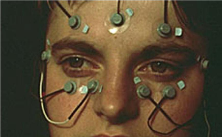
**Fig. 5.1** Example of electro-oculography (EOG) eye movement measurement. Courtesy of Metro-Vision, Pénchenies, France (<http://www.metrovision.fr>). Reproduced with permission
