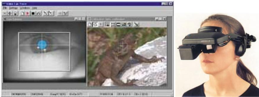
**Fig. 5.6** Example of head-mounted video-based eye tracker. Courtesy of IOTA AB, EyeTrace Systems, Sundsvall Business & Tech. Center, Sundsvall, Sweden (<http://www.iota.se>). Reproduced with permission
