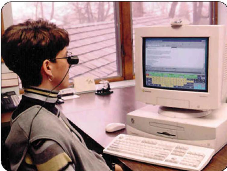
**Fig. 24.2** Example of eye typing interface. Courtesy of Prentke Romich Company, Wooster, OH <http://www.prentrom.com/access/hm2000.html>. Reproduced with permission
