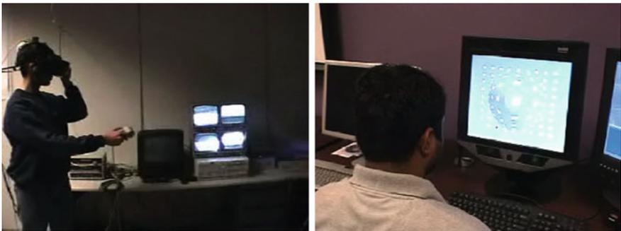
**Fig. 19.1** Head-mounted and desktop (binocular) eye trackers
