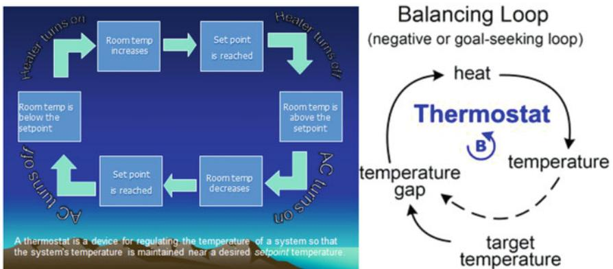
Fig. 1.6 Temperature control system in a room
