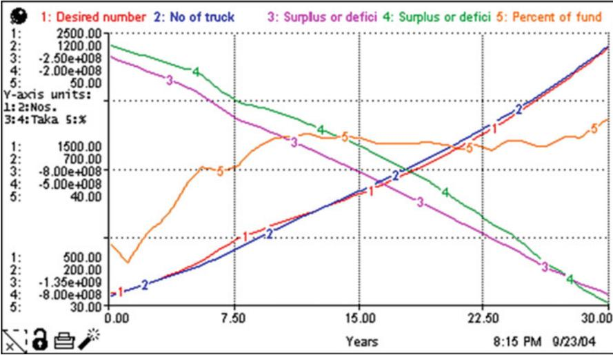
**Fig. 12.6** Simulated desired number of trucks, number of trucks used, surplus or deficit budget, surplus or deficit budget for collection and percent of fund available for collection for a time horizon of 30 years
