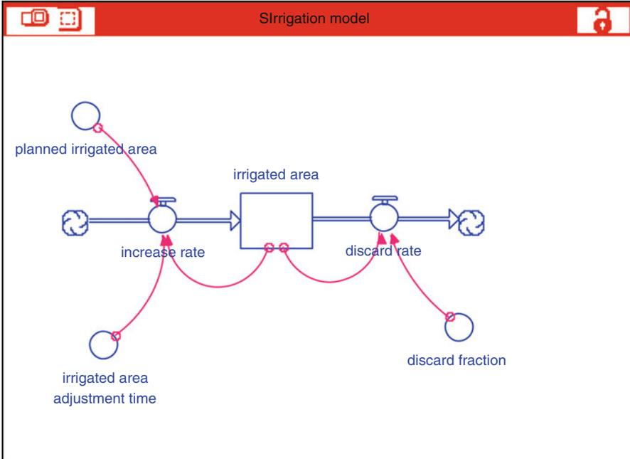
**Fig. 2.6** Stock–flow diagram of the irrigation model
