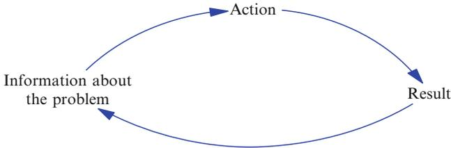
**Fig. 1.4** Closed loop system concept
