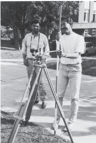
Fig. 3.6 Tension being applied with the aid of a ranging rod to a steel band suspended in catenary
