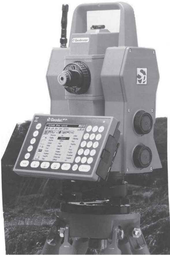
Fig. 3.32 Robotic surveying system by Spectra-Precision
