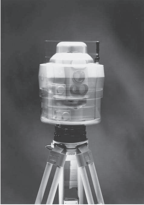
Fig. 3.29 Geodimeter, rotating automatically in its search for the reflector pole
