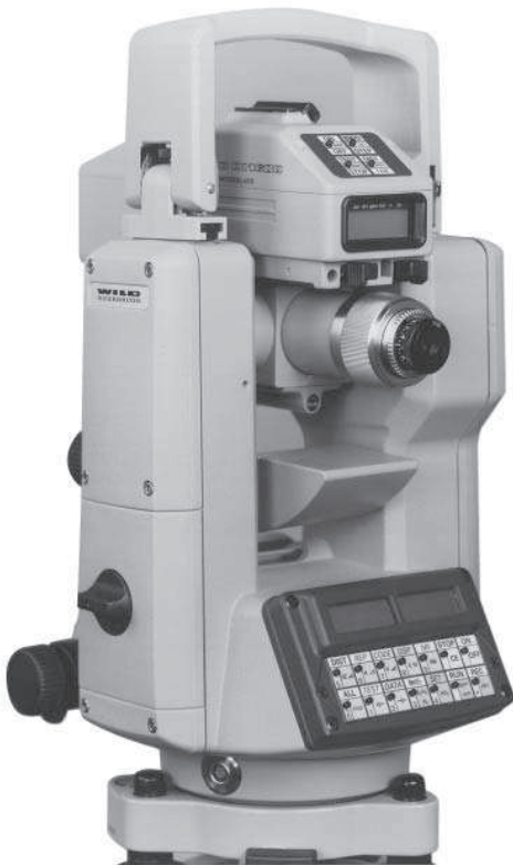
Fig. 3.12 (a) Wild DI 1600 E.D.M (b) Wild DI 1600 top-mounted on the telescope of the Wild T 1000 Electronic theodolite
