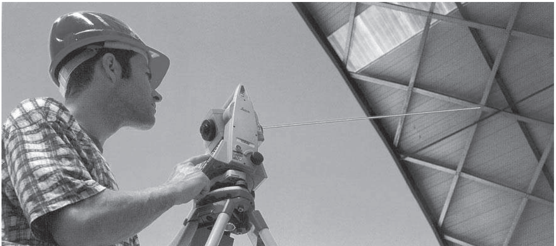
Fig. 3.30 Reflectorless surveying (Courtesy of Leica)
