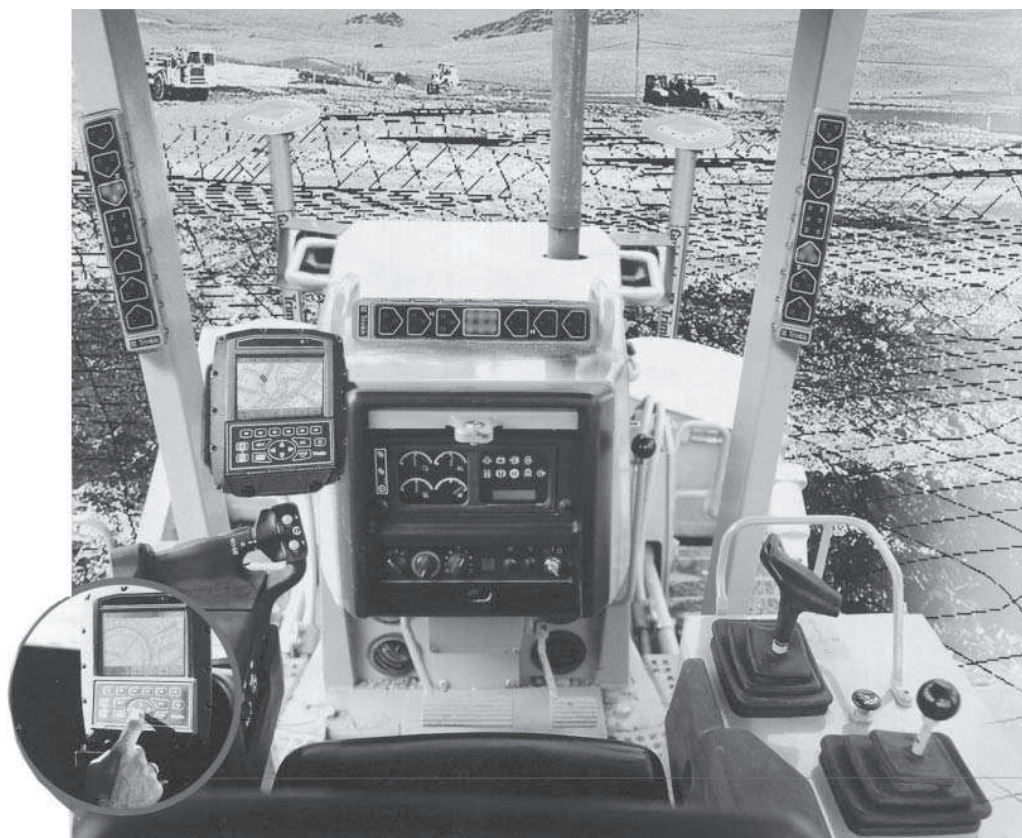
Fig. 7.25 'Site vision GPS' machine guidance by Trimble, showing 2 GPS antennae and the in-cab control system
