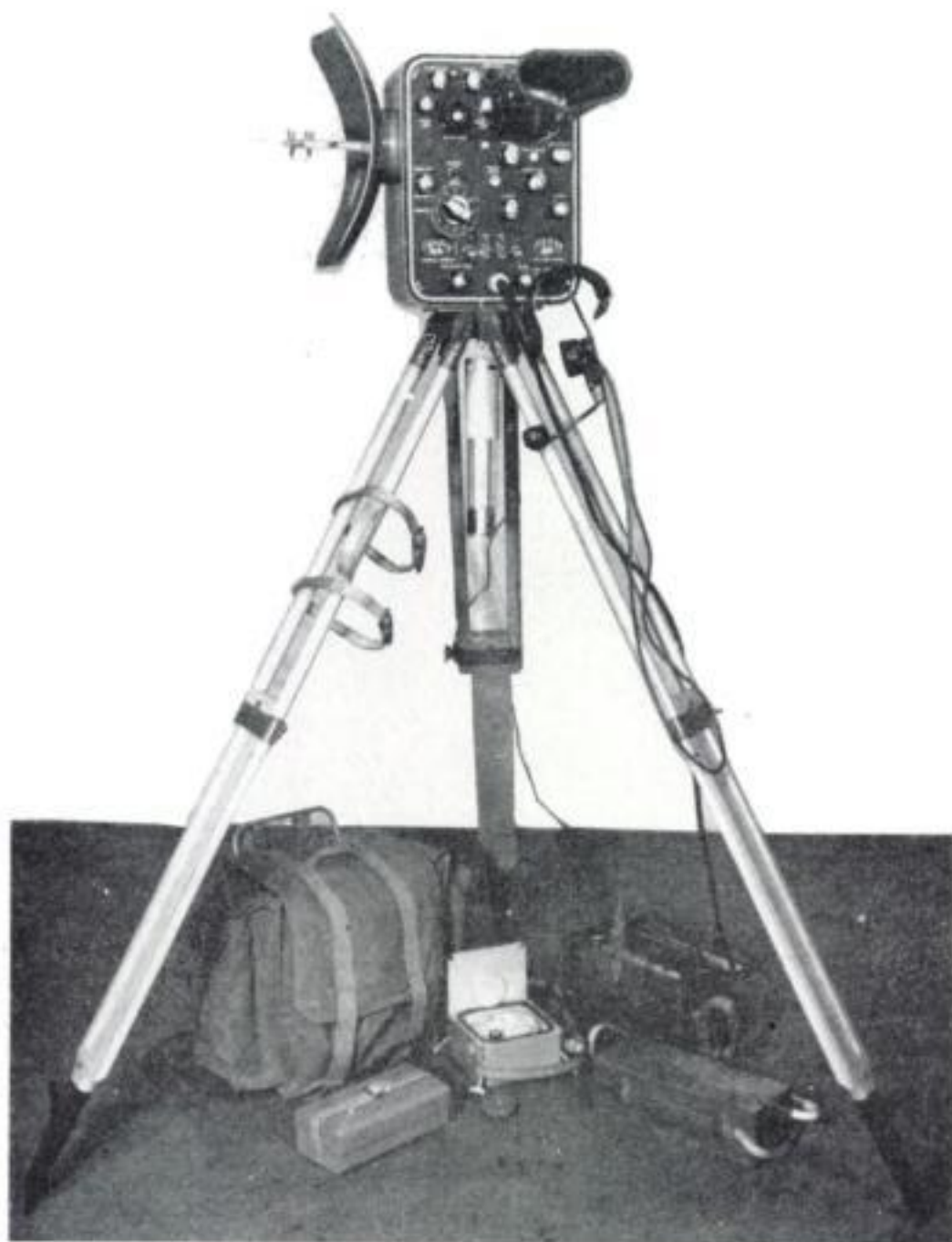
FIG. 3.8 THE TELLUROMETER MODEL MRA-2 (M/S COOKE, TROUGHTON & SIMMS LTD.)
