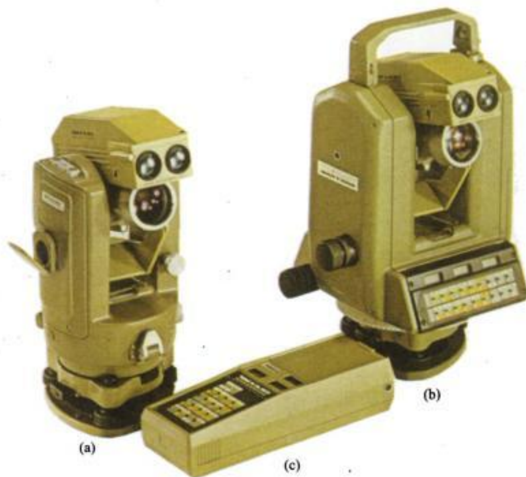
FIG. 3.10. WILD DI 1000 DISTOMAT FITTED TO WILD OPTICAL AND ELECTRONIC THEODOLITES
