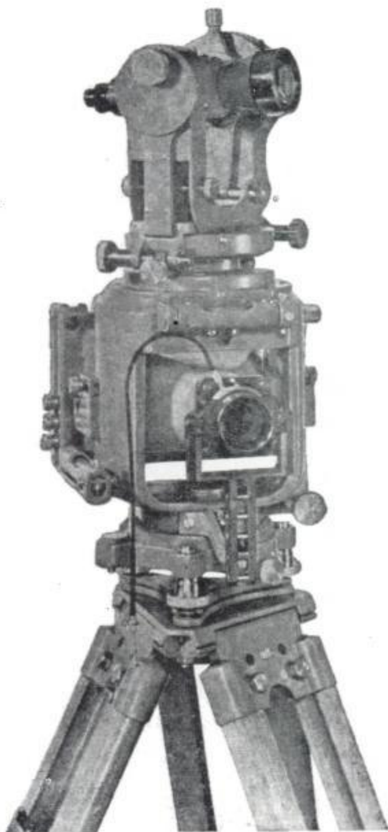
FIG. 2.3. PHOTO-THEODOLITE BY M/S WILD HEERBRUGG LTD. (BY COURTESY OF MANUFACTURERS)
