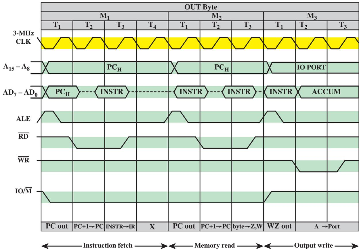
**Figure 19.9 Timing Diagram for Intel 8085 OUT Instruction**
