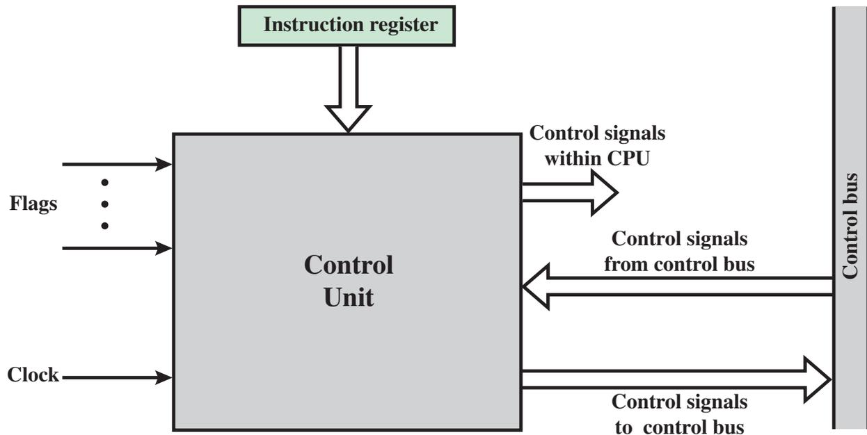
**Figure 19.4 Block Diagram of the Control Unit**
