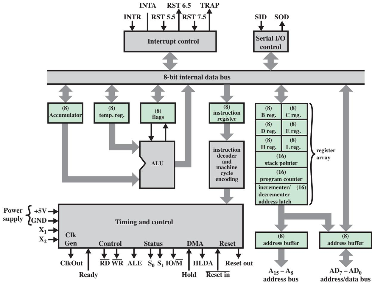
**Figure 19.7 Intel 8085 CPU Block Diagram**
