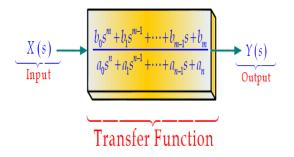
Block diagram representation of a transfer function
