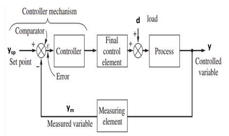
The general equation for closed block diagram
