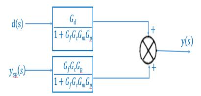
The denominator of the transfer functions;  $1 + G_f G_c G_p G_m$  is equal to 1 plus multiplication of all the transfer functions in the loop.
