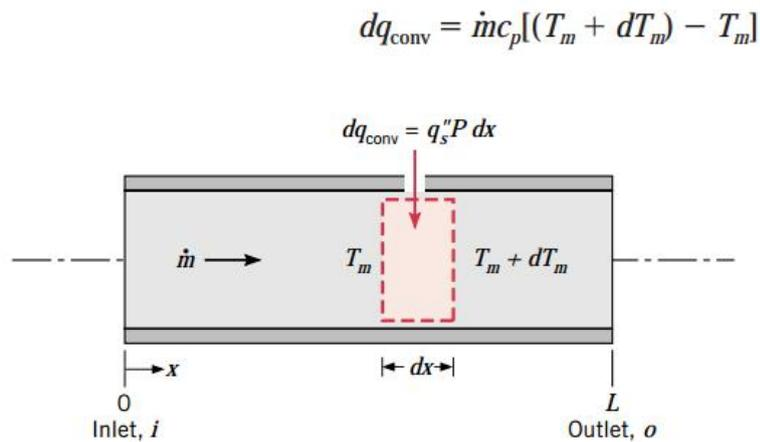
**FIGURE 8.6** Control volume for internal flow in a tube.
