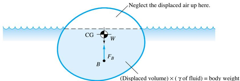
**Fig. 2.17** Static equilibrium of a floating body.
