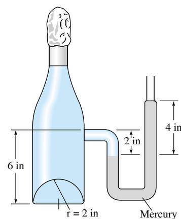
**P2.85** Compute the horizontal and vertical components of the hydrostatic force on the quarter-circle panel at the bottom of the water tank in Fig. P2.85.
