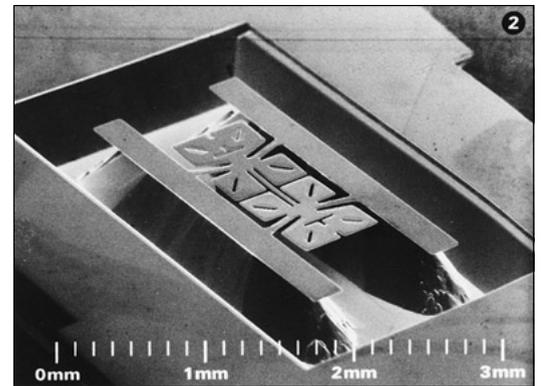
**Fig. 2.28** Pressure sensors with electric output: (a) a silicon diaphragm whose deflection changes the cavity capacitance (Courtesy of Johnson-Yokogawa Inc.); (b) a silicon strain gage which is stressed by applied pressure; (c) a micromachined silicon element which resonates at a frequency proportional to applied pressure. [(b) and (c) are courtesy of Druck, Inc., Fairfield, CT.]
