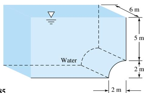
**\*P2.88** Gate  $ABC$  is a circular arc, sometimes called a *Tainter gate*, which can be raised and lowered by pivoting about point  $O$ . See Fig. P2.88. For the position shown, determine (a) the hydrostatic force of the water on the gate and (b) its line of action. Does the force pass through point  $O$ ?
