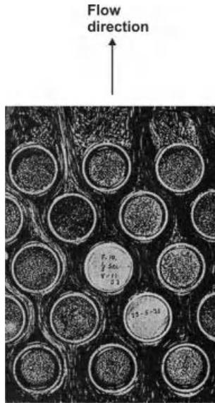
**Figure 4.16** Flow pattern for a staggered tube bank (Çengel (3), reprinted with permission)
