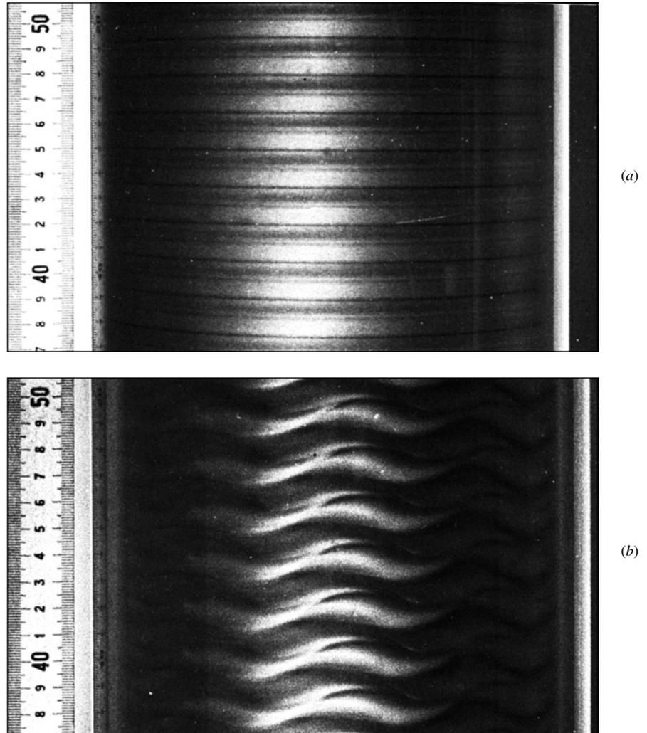
**Fig. 4.18** Experimental verification of the instability of flow between a fixed outer and a rotating inner cylinder. (a) Toroidal Taylor vortices exist at 1.16 times the critical speed; (b) at 8.5 times the critical speed, the vortices are doubly periodic. (After Koschmieder, Ref. 18.) This instability does not occur if only the outer cylinder rotates.
