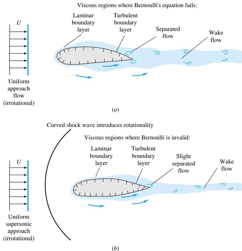
**Fig. 4.11** Typical flow patterns illustrating viscous regions patched onto nearly frictionless regions: (a) low subsonic flow past a body ( $U \ll a$ ); frictionless, irrotational potential flow outside the boundary layer (Bernoulli and Laplace equations valid); (b) supersonic flow past a body ( $U > a$ ); frictionless, rotational flow outside the boundary layer (Bernoulli equation valid, potential flow invalid).
