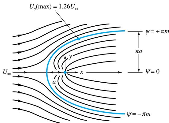
**Fig. 4.15** Superposition of a source plus a uniform stream forms a Rankine half-body.
