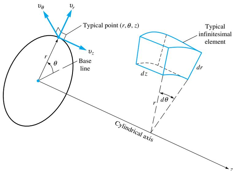
**Fig. 4.2** Definition sketch for the cylindrical coordinate system.
