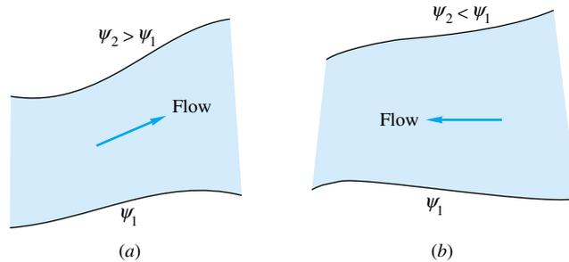
Thus the change in  $\psi$  across the element is numerically equal to the volume flow through the element. The volume flow between any two points in the flow field is equal to the change in stream function between those points:
