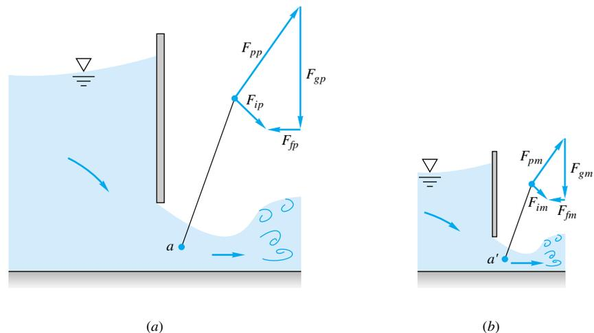
**Fig. 5.7** Dynamic similarity in sluice-gate flow. Model and prototype yield identical homologous force polygons if the Reynolds and Froude numbers are the same corresponding values: (a) prototype; (b) model.
