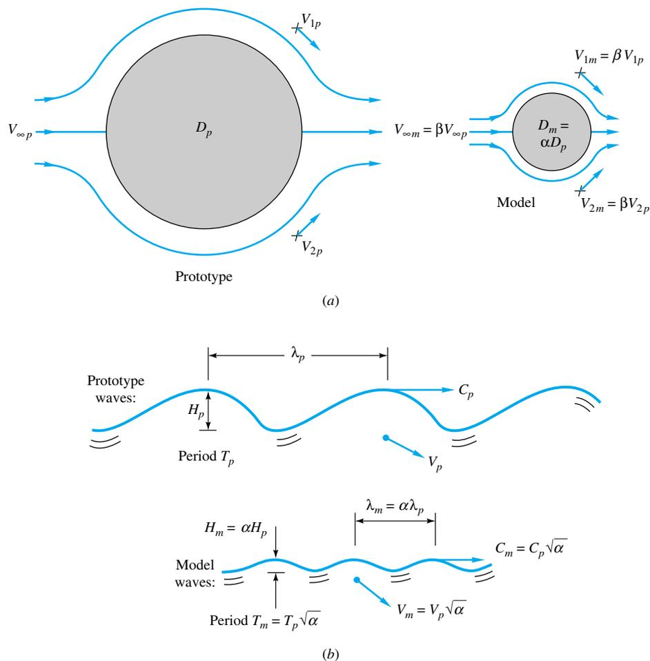
**Fig. 5.6** Frictionless low-speed flows are kinematically similar: (a) Flows with no free surface are kinematically similar with independent length- and time-scale ratios; (b) free-surface flows are kinematically similar with length and time scales related by the Froude number.
