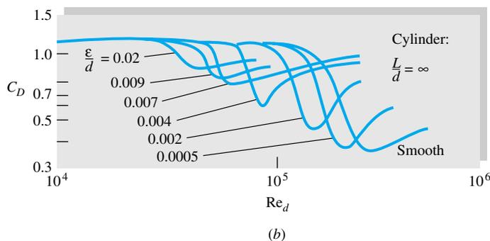
**Fig. 5.3** The proof of practical dimensional analysis: drag coefficients of a cylinder and sphere: (a) drag coefficient of a smooth cylinder and sphere (data from many sources); (b) increased roughness causes earlier transition to a turbulent boundary layer.
