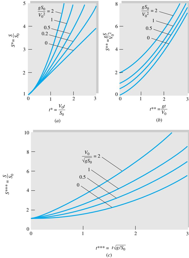
**Fig. 5.1** Three entirely equivalent dimensionless presentations of the falling-body problem, Eq. (5.5): the effect of (a) gravity, (b) initial displacement, and (c) initial velocity. All plots contain the same information.
