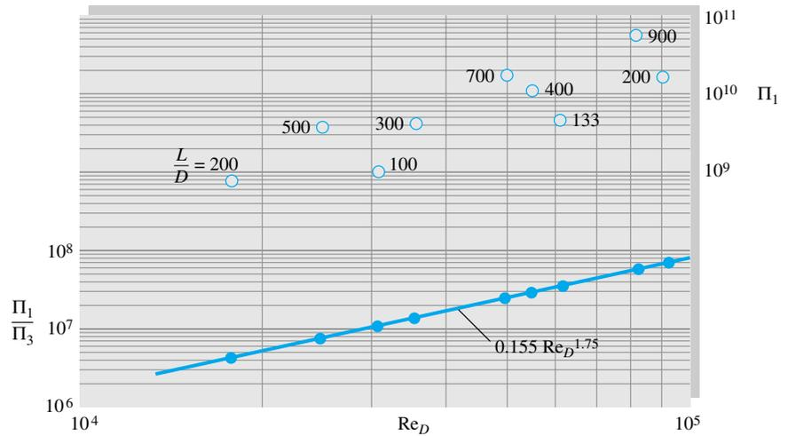
$$\frac{\rho D^3 \Delta p}{L \mu^2} = \text{fcn}\left(\frac{\rho V D}{\mu}\right) \quad \text{flow in a long pipe} \quad \text{Ans. (c)}$$
