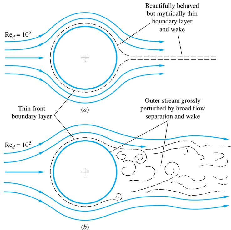
**Fig. 7.2** Illustration of the strong interaction between viscous and inviscid regions in the rear of blunt-body flow: (a) idealized and definitely false picture of blunt-body flow; (b) actual picture of blunt-body flow.
