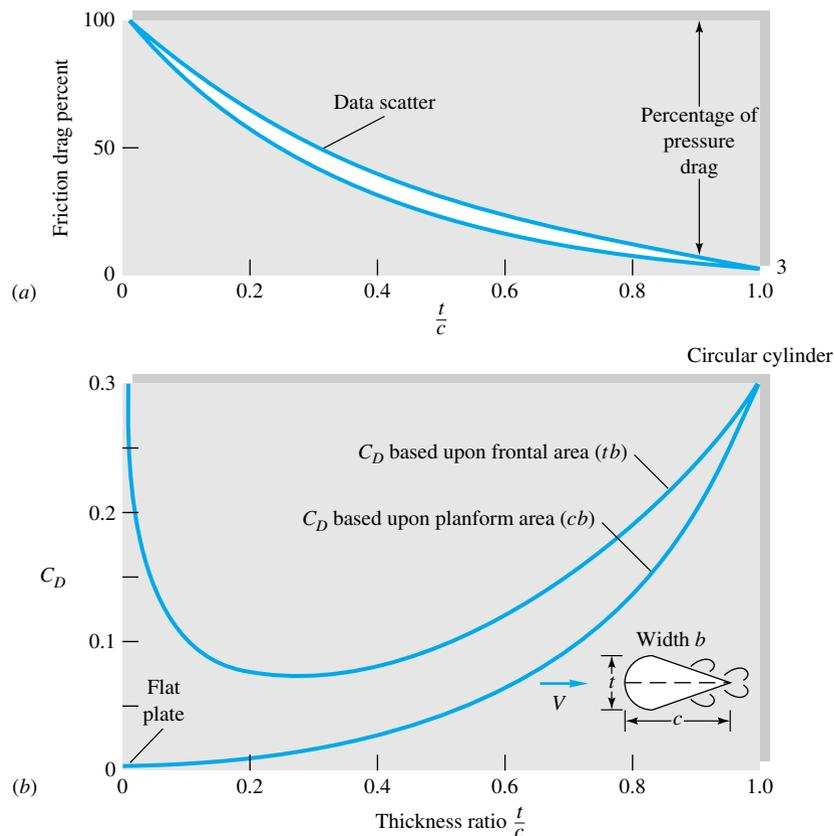
**Fig. 7.12** Drag of a streamlined two-dimensional cylinder at  $Re_c = 10^6$ : (a) effect of thickness ratio on percentage of friction drag; (b) total drag versus thickness when based upon two different areas.
