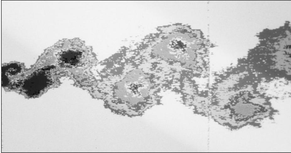
The turbulent wake behind a bluff body immersed in a stream flow is a subject of the present chapter. This is a digitized video image showing the distribution of tracer-dye concentration in the wake of the body. Compare with Fig. 5.2a of the text, which is a laminar wake. (*Courtesy of R. Balachandar, by permission of the American Society of Mechanical Engineers.*)
