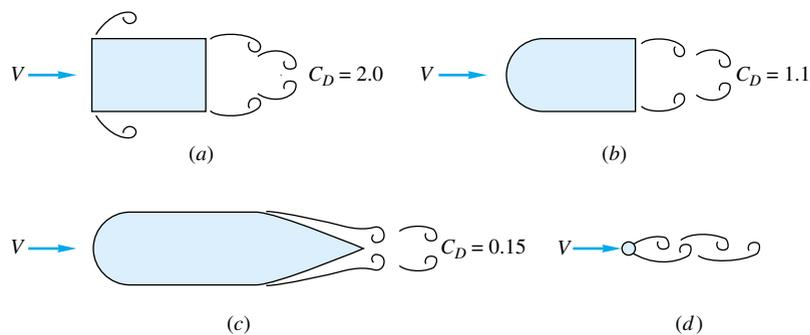
**Fig. 7.15** The importance of streamlining in reducing drag of a body ( $C_D$  based on frontal area): (a) rectangular cylinder; (b) rounded nose; (c) rounded nose and streamlined sharp trailing edge; (d) circular cylinder with the same drag as case (c).
