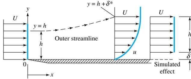
**Fig. 7.4** Displacement effect of a boundary layer.
