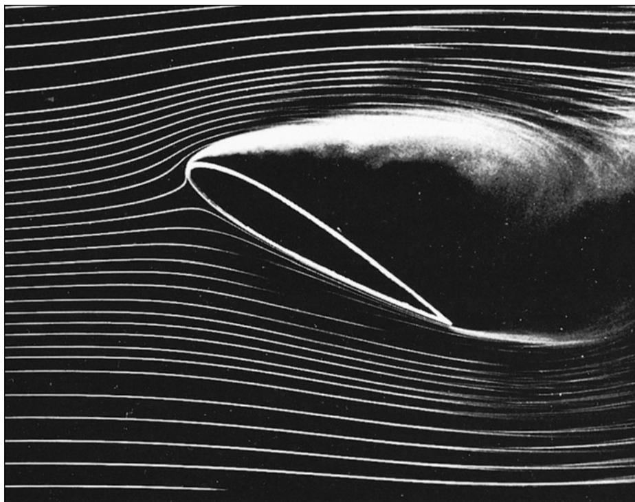
**Fig. 7.24** At high angle of attack, smoke-flow visualization shows stalled flow on the upper surface of a lifting vane. [From Ref. 19, Illustrated Experiments in Fluid Mechanics (*The NCFMF Book of Film Notes*), National Committee for Fluid Mechanics Films, Education Development Center, Inc., copyright 1972.]
