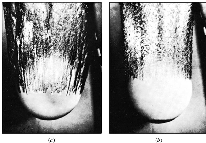
**Fig. 7.14** Strong differences in laminar and turbulent separation on an 8.5-in bowling ball entering water at 25 ft/s: (a) smooth ball, laminar boundary layer; (b) same entry, turbulent flow induced by patch of nose-sand roughness. (U.S. Navy photograph, Ordnance Test Station, Pasadena Annex.)
