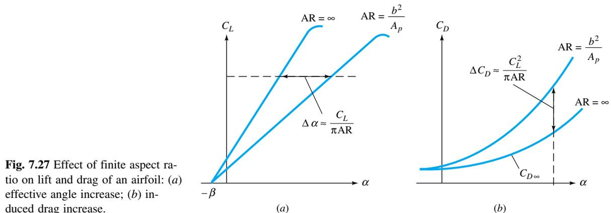
**Fig. 7.27** Effect of finite aspect ratio on lift and drag of an airfoil: (a) effective angle increase; (b) induced drag increase.
