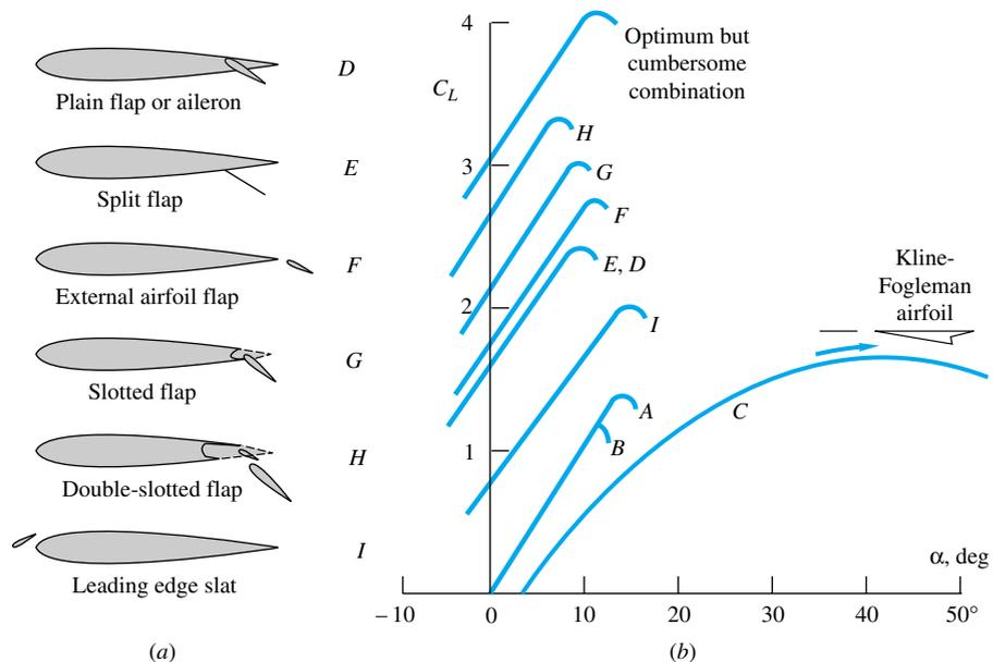
**Fig. 7.28** Performance of airfoils with and without high-lift devices:  $A = \text{NACA } 0009$ ;  $B = \text{NACA } 63-009$ ;  $C = \text{Kline-Fogleman airfoil}$  (from Ref. 17);  $D$  to  $I$  shown in (a): (a) types of high-lift devices; (b) lift coefficients for various devices.
