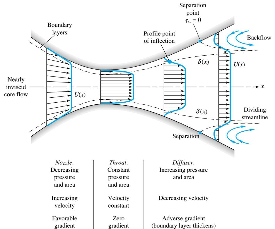
**Fig. 7.8** Boundary-layer growth and separation in a nozzle-diffuser configuration.
