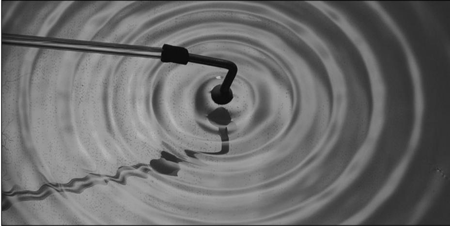
Cylindrical wave pattern produced in a ripple tank. When not modified by the no-slip condition at solid surfaces, waves are nearly inviscid and well represented by the potential theory of this chapter. (Courtesy of Dr. E. R. Degginger/Color-Pic Inc.)
