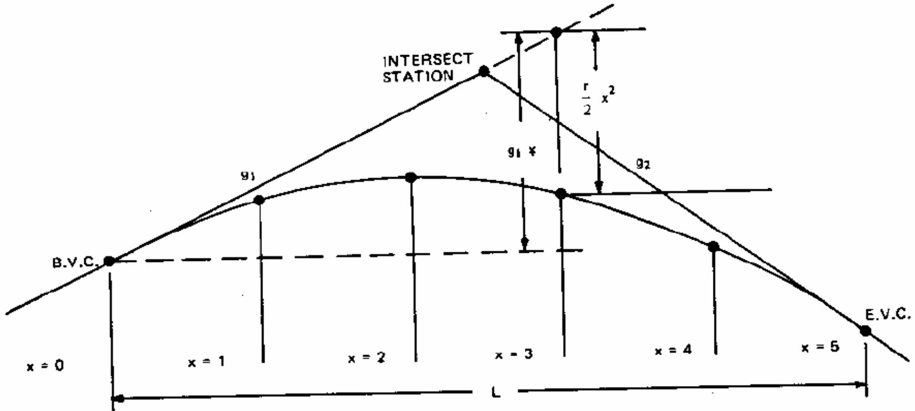
Vertical curves (VC) are used to connect intersecting gradients in the vertical plane.
