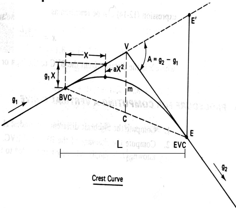
➤ The difference in elevation between the BVC and a point on the  $g_1$  grade line at a distance  $X$  units (feet or meters) is  $g_1 X$  ( $g_1$  is expressed as a decimal).
