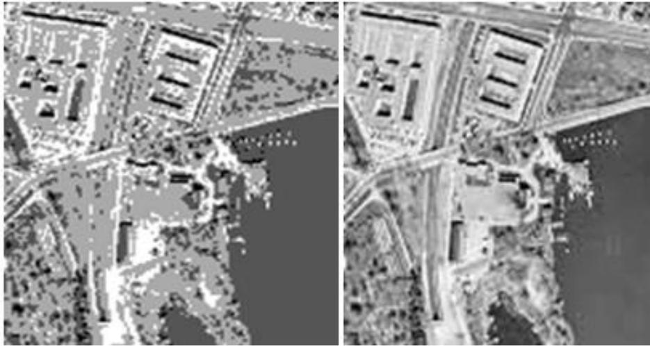
Figure 5-10 Radiometric Resolution
