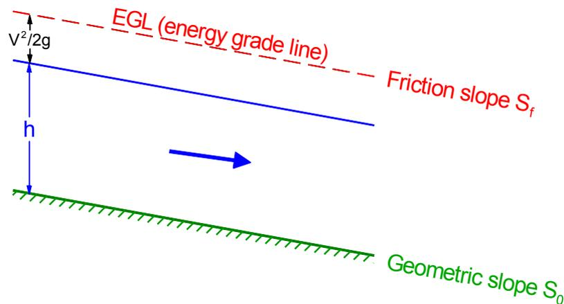
In *normal flow* the downslope component of weight balances bed friction. As a result, the water depth  $h$  and velocity  $V$  are constant and the total-head line (or *energy grade line*) is parallel to both the water surface and the channel bed; i.e. the *friction slope*  $S_f$  is the same as the *geometric slope*  $S_0$ .
