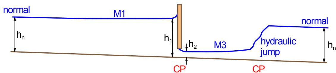
*Flow under a sluice gate – (b) steep slope*
