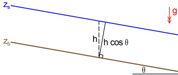
Although not crucial, we make the *small-slope* assumption and make no distinction between the vertical depth  $h$  (which forms part of the total head) and that perpendicular to the bed,  $h \cos \theta$  (which is used to get the flow rate).
