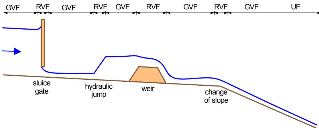
As a result of disturbances due to hydraulic structures (weir, sluice, etc.) or changes to channel width, slope or roughness the downslope component of weight may not locally balance bed friction. As a result, the friction slope  $S_f$  and bed slope  $S_0$  will be different and the water depth  $h$  and velocity  $V$  will change along the channel.
