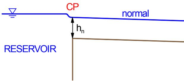
Flow from a reservoir – (b) steep slope
