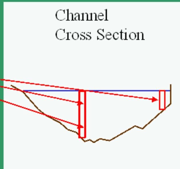
Discharge= Velocity x Depth x Width
