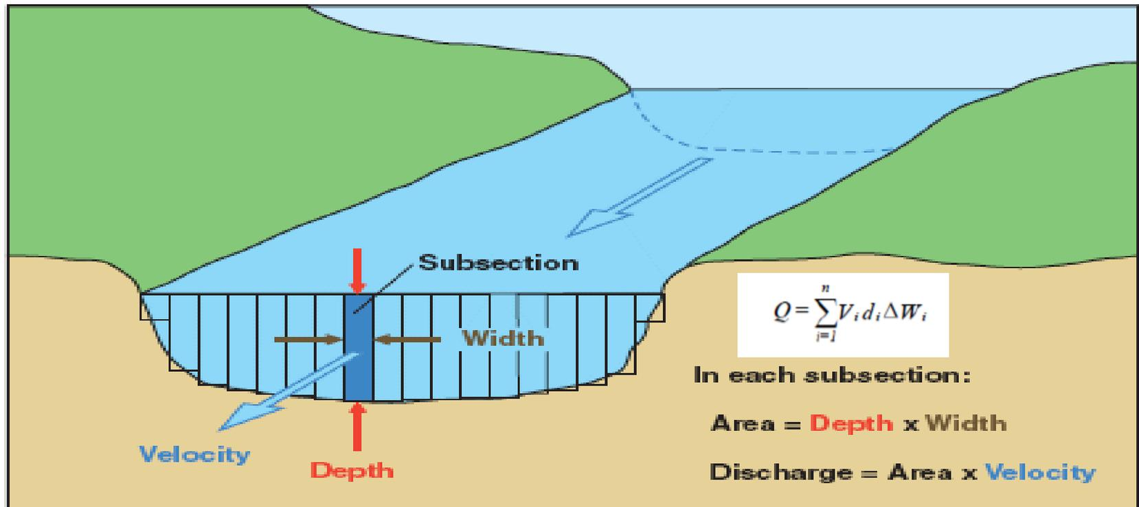
Current-meter discharge measurements are made by determining the discharge in each subsection of a channel cross section and summing the subsection discharges to obtain a total discharge.
