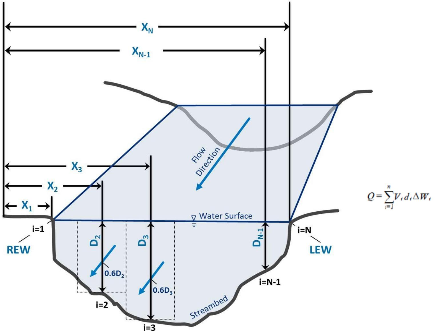
EXAMPLE 4.1 The data pertaining to a stream-gauging operation at a gauging site are given below.
