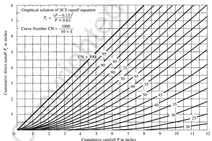
• To standardize these curves, a dimensionless curve number CN is defined such that 0 < CN < 100. For impervious and water surfaces CN = 100; for natural surfaces CN < 100.
