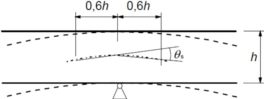
**Figure 1-13 – Plastic rotation of  $\theta_s$  of reinforced concrete sections for continuous beams and continuous one way spanning slabs**
