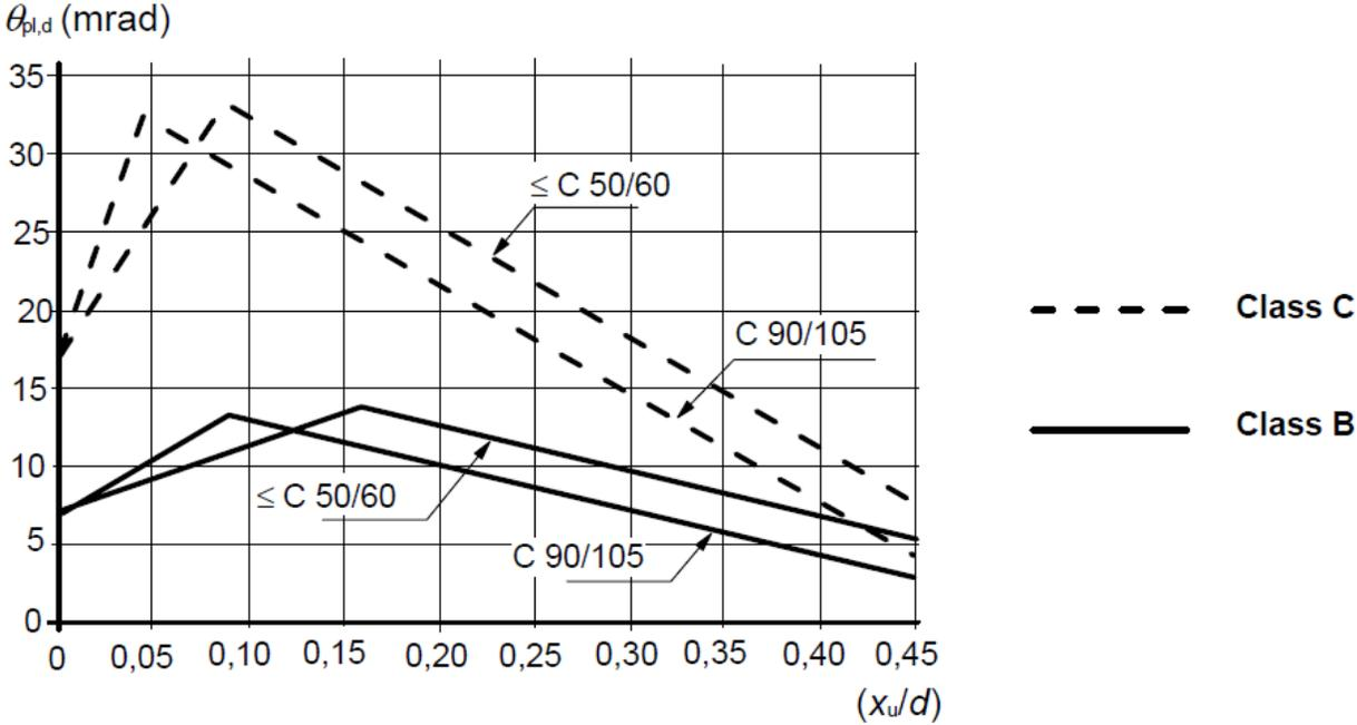
**Figure 1-14 – Allowable plastic rotation,  $\theta_{pl,d}$ , of reinforced concrete sections for Class B and C reinforcement.**
