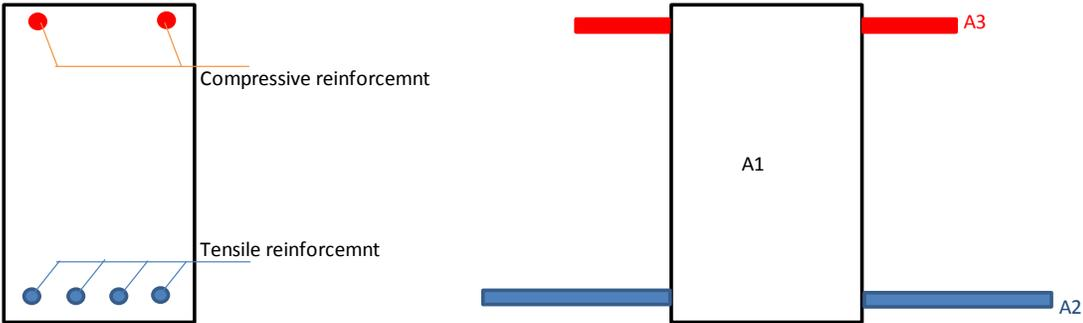
Figure 1-2 - Transformed Un-Cracked Section
