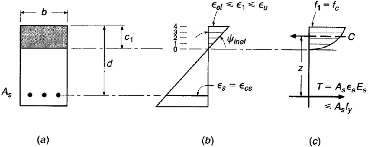
**Figure 1-7 – Cracked beam with concrete in the inelastic range of loading**
