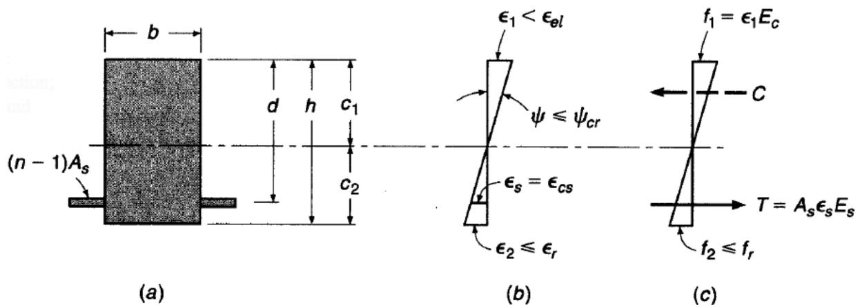
Figure 1-5 – Uncracked beam in the elastic range of loading
