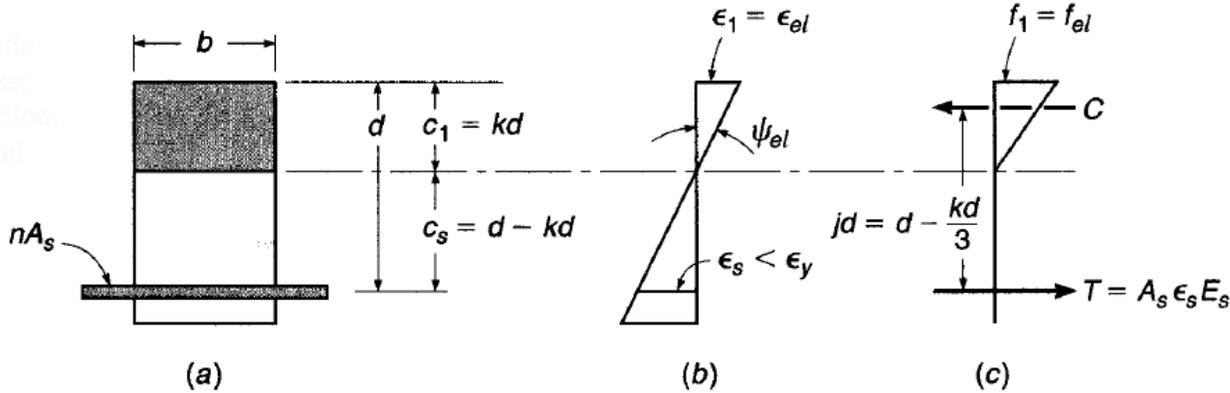
**Figure 1-6 – Cracked beam in the elastic range of material response**
