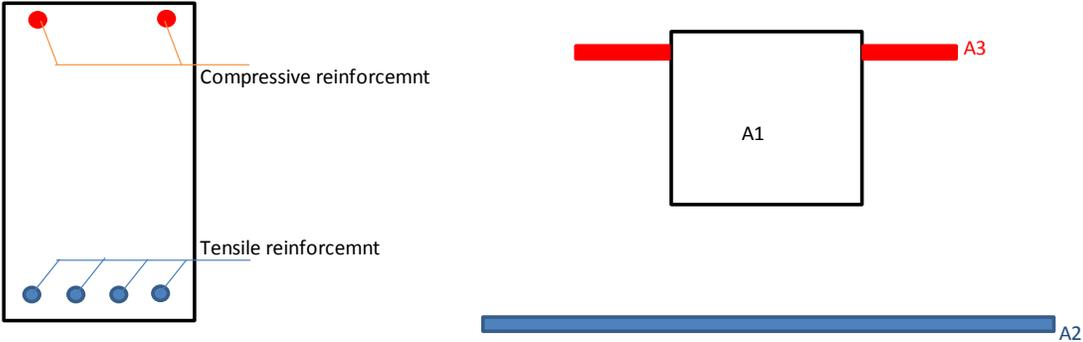
Figure 1-3 - Transformed Cracked Section
