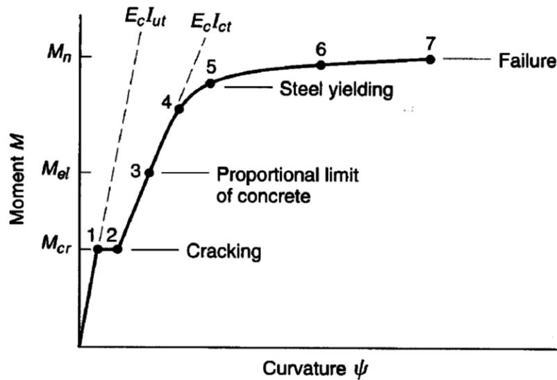
Figure 1-4 Moment-Curvature relationship for Reinforced Concrete Beam
