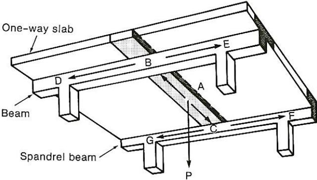
Figure 1-8 – One-way slab and continuous beam
