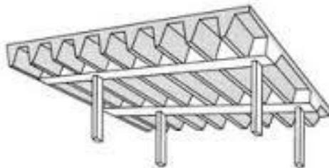
**Figure 2-1 – Ribbed slab layout**
