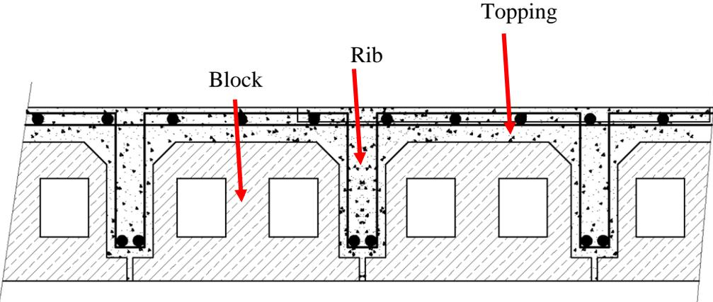
Figure 2-3 Typical ribbed slab cross-section
