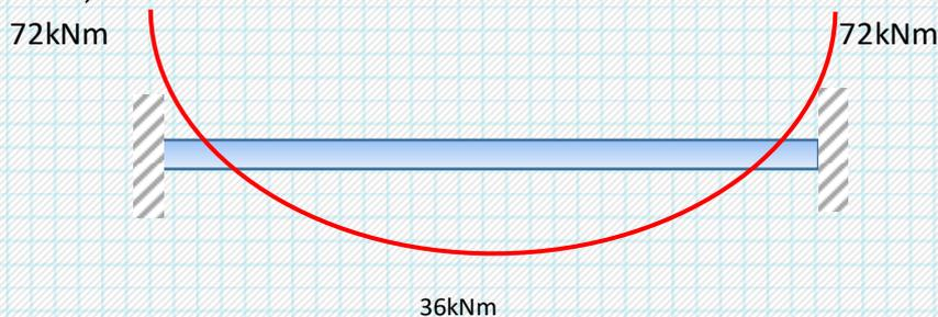
**Step 3:** design the beam at the supports and mid span
