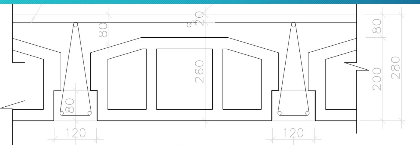
Section of the precast ribs and blocks with the topping. (low-cost housing projects)
