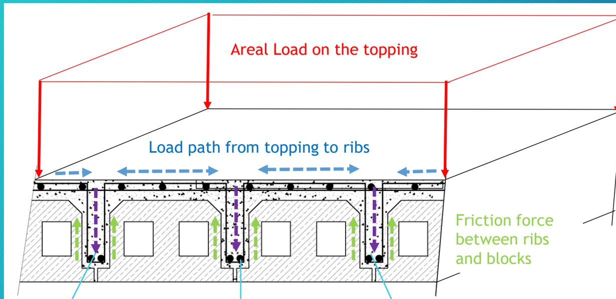
Total load carried by each rib = load from topping + load from blocks
