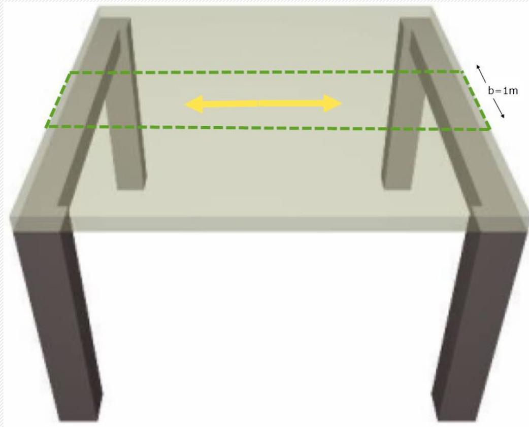
In the design and analysis of one way slab systems a 1m strip of slab along the load transfer direction is considered
