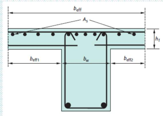
For span moments flange width equal to the distance between ribs = 400 mm
