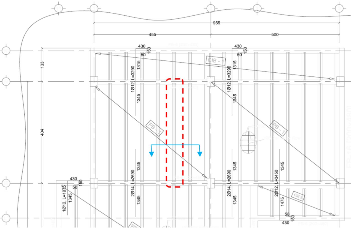
Plan-Layout (precast rib slab system)
