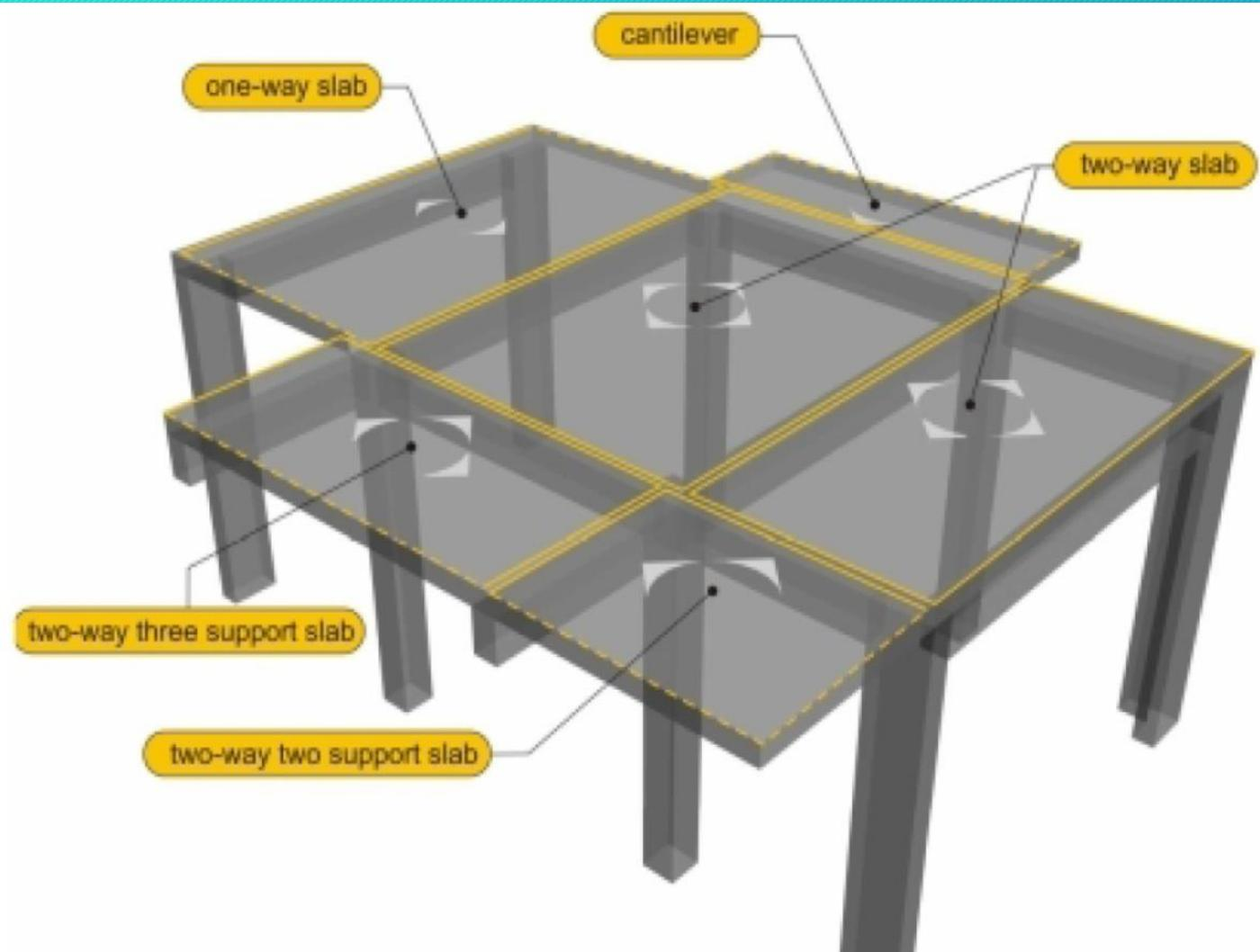
**1. One-way slabs:** They are those either supported on the two out of four opposite sides or the longer span to short span ratio is at least equal to 2.
