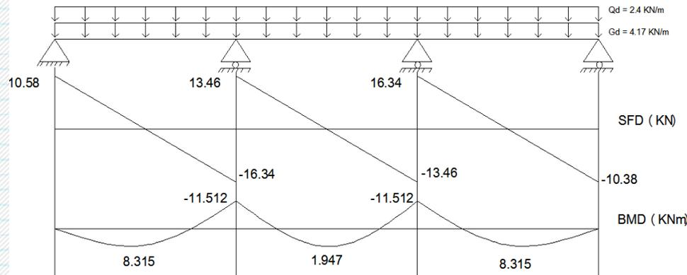
**Case 2: Adjucet span loading for max. support moment at B or C**
