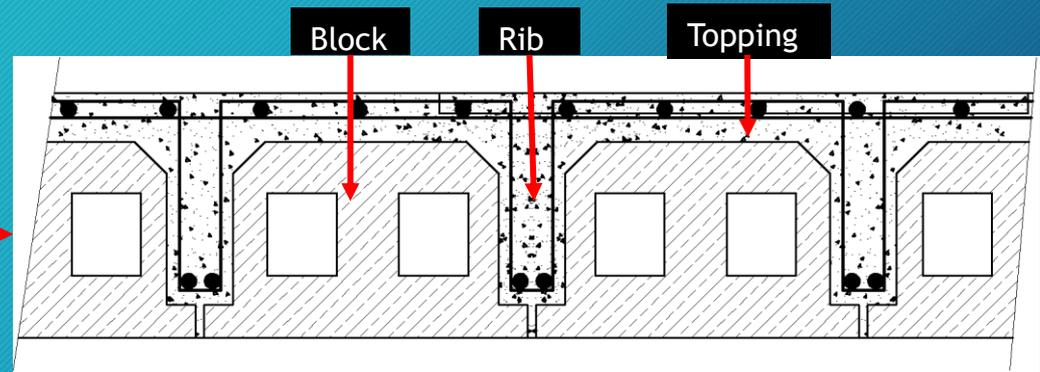
They may be constructed in a variety of ways, two principal methods of construction are:
