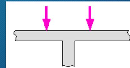
When the total shear force exceeds the shear resistance of the slab, the slab will be ‘pushed down’ around the column, or this can be viewed as the column being ‘pushed’ through the slab, thus:
