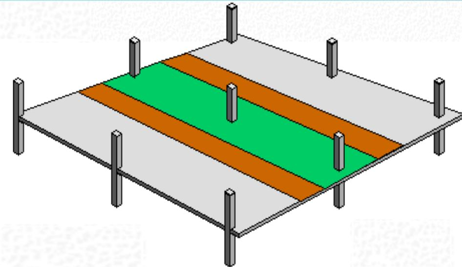
To ensure that the **distribution of reinforcement** corresponds approximately to the **distribution of moments** arising from a rigorous analysis of the slab system, the slab strip is divided into a **column strip** and **middle strip** (half each side), thus:
