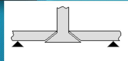
The failure mechanism is by shear, hence the name **Punching Shear**.
