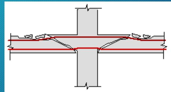
However, **the bottom bars**, being more deeply embedded, are not pushed out in the same way and thus provide more resistance. this is attributable initially to **dowel action**, and then later at larger deformation to its being **kinked**, as shown.
