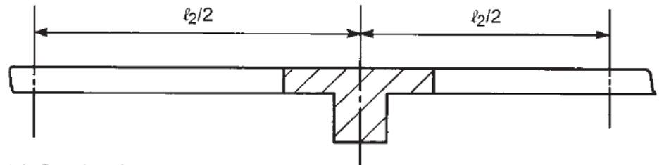
(c) Section for  $I_b$ —Interior beam.
