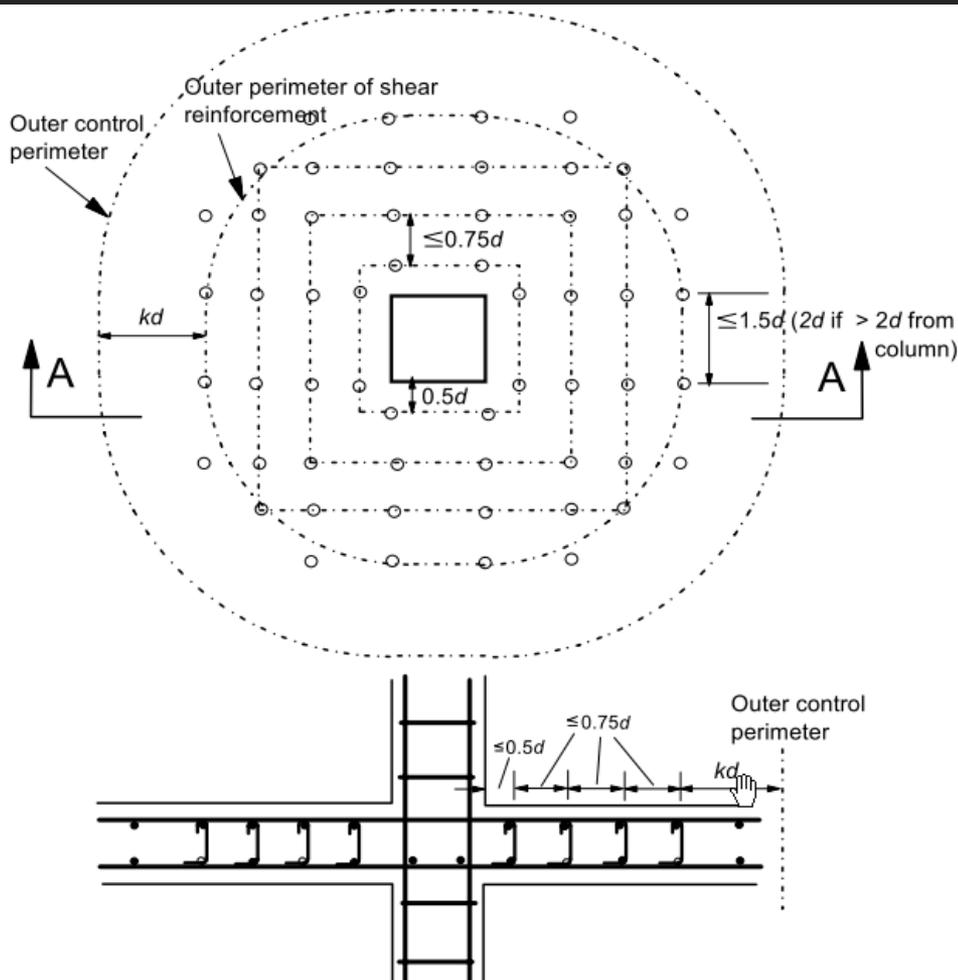
The outer control perimeter at which shear reinforcement is not required, should be calculated from:
