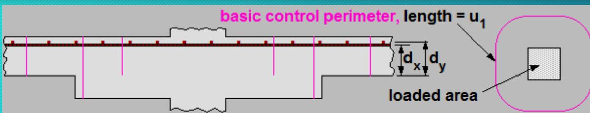
An increased depth of slab or **slab drop/drop panel** around the column reduces  $V_{Ed}$  by increasing the length of the **basic control perimeter**  $u_1$
