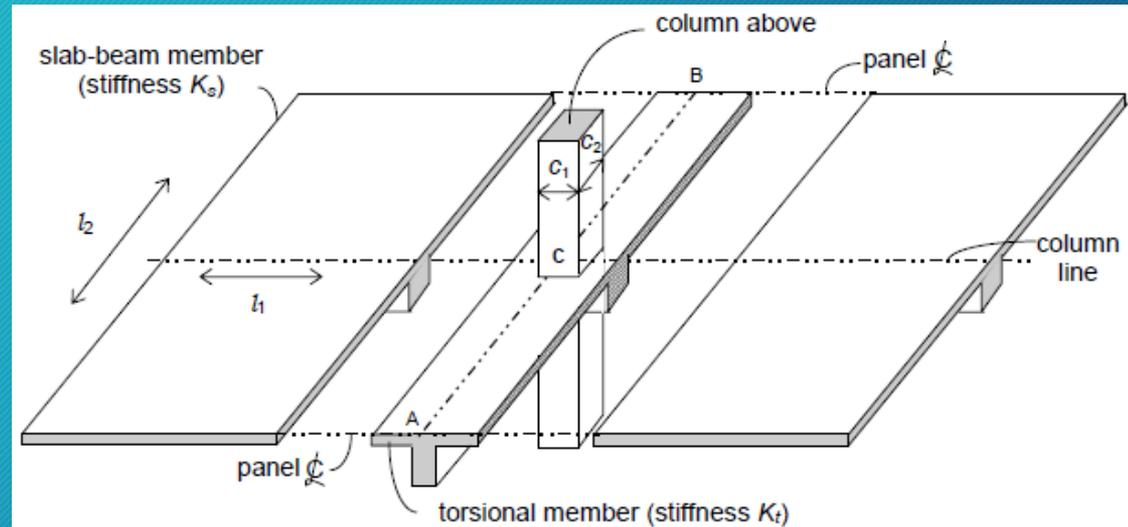
To account for the increased flexibility of the slab-to-column connection, it is recommended to use an equivalent column with stiffness  $K_{ec}$  to replace the actual columns and torsional members.
