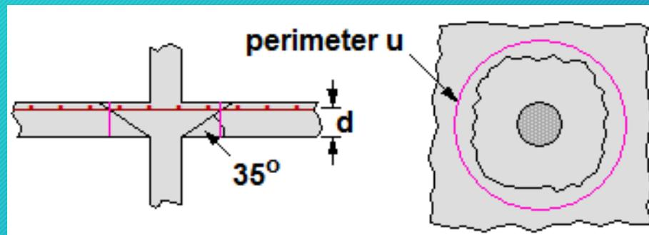
Thus, the shear force acting on a perimeter  $u$  around the loaded area is resisted by a nominal shear stress (capacity)  $V_{Rd,c}$  acting over the average effective depth  $d$  of the section
