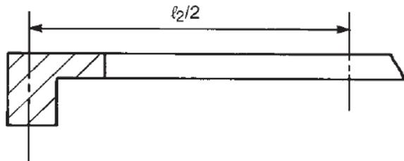
(a) Section for  $I_b$ —Edge beam.
