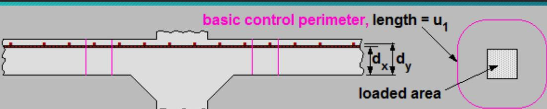
An enlarged **column head** or **column capital** increases the perimeter of the loaded area,  $u_o$  so reducing the shear stress,  $V_{Ed}$ .
