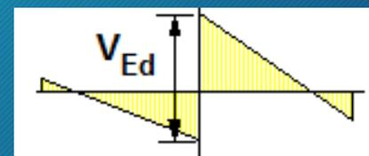
Generally, moment is transferred to the columns so the shear distribution is **not uniform** and a factor,  $\beta$  is used to take account off local concentrations.
