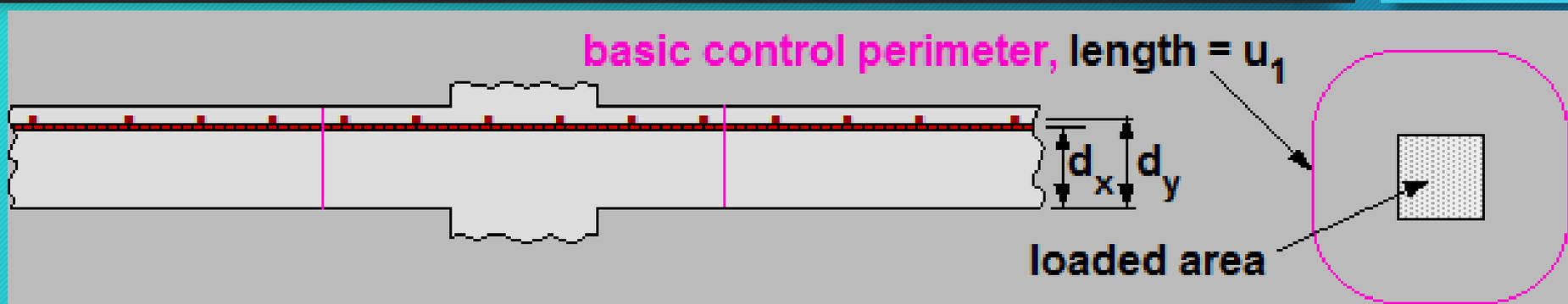
If  $V_{Ed}$  exceeds  $V_{Rd,c}$  at the basic control perimeter by small amount, and this was true of many slab-column connection in the design, then either the loaded area or the slab depth could be increased, although the latter would also increase the permanent load.
