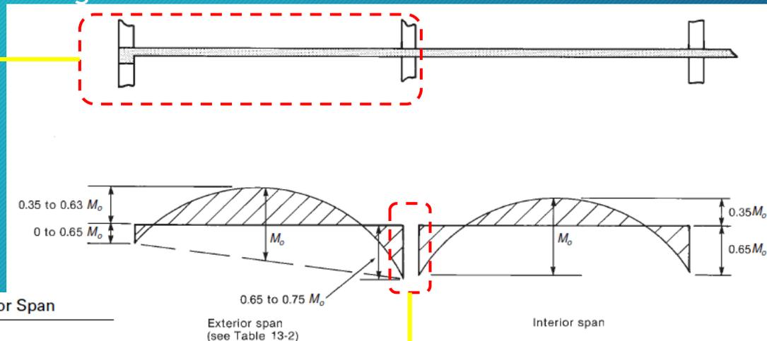
TABLE 13-2 Distribution of Total Factored Static Moment,  $M_o$ , in an Exterior Span
