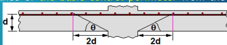
This gives an angle  $\theta = 26.6^\circ$  ( $\arctan(1/2)$ ) with the horizontal, outside the plain of failure.
