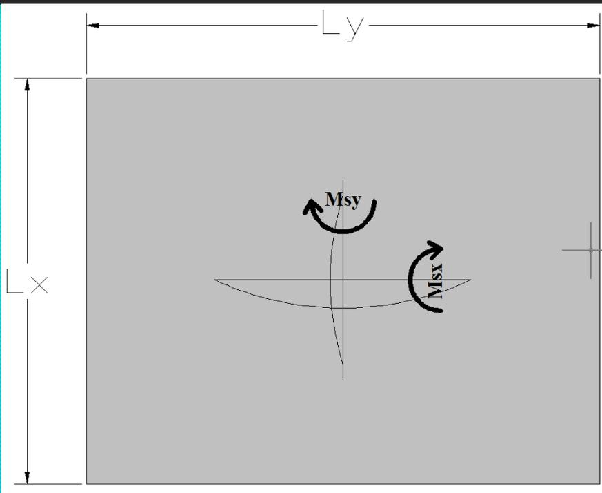
When simply-supported slabs do not have adequate provision to resist torsion at the corners, and to prevent the corners from lifting, the **maximum moments per unit width** are given by the following equations:
