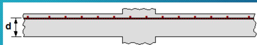
To be largely independent to this ratio, the distance of **the basic control perimeter** from the face of the loaded area is taken as  $2d$ .
