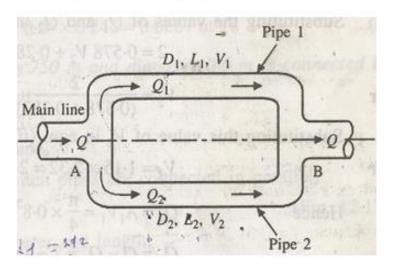
When the pipes are arranged parallel, the loss of head in each pipe (branch) is the same
