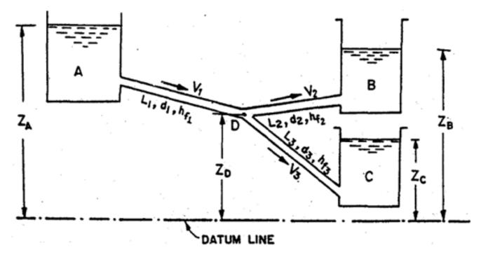
Given the lengths, diameters, and coefficient of friction of each pipe, it is required to find the discharge and the direction of flow in each pipe
