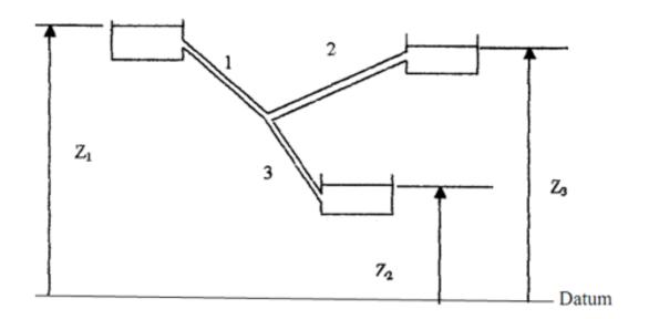
The flow through each pipe is to be determined when the reservoir elevations are given
