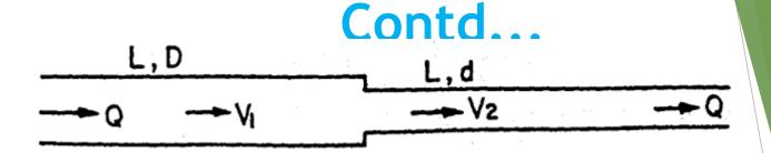
Two pipes of different diameters connected in series
